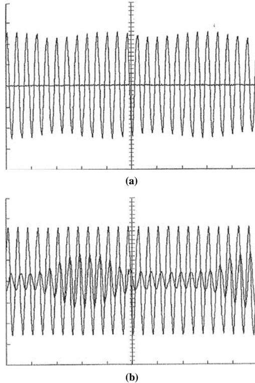
**Notes:** (a) Without voltage-sourced converter + battery energy storage facility; (b) with voltage-sourced converter + battery energy storage facility
