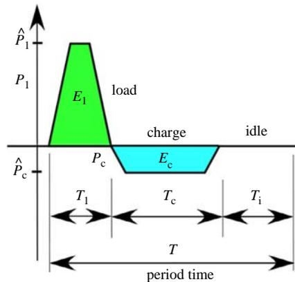
**Notes:** During the total cycle time  $T$ , the battery is discharged to the grid with power  $P_1$  during time  $T_1$  and charged with power  $P_c$  during time  $T_c$ ; remaining time  $T_i$  is idle time
