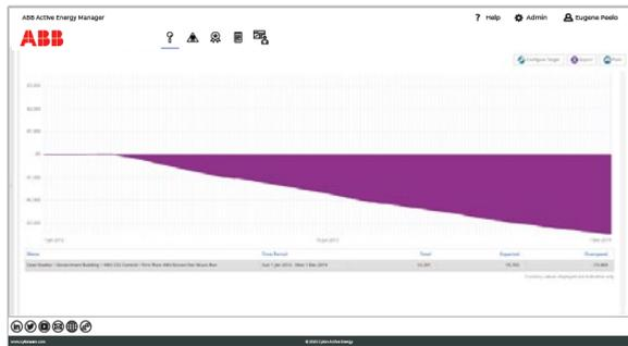
Represents the sum of the daily savings or total savings achieved over the period from the installation of the CO<sub>2</sub> sensors to control the AHU Extract fans. A total of €3.5k was saved for this meter over the two year period.
