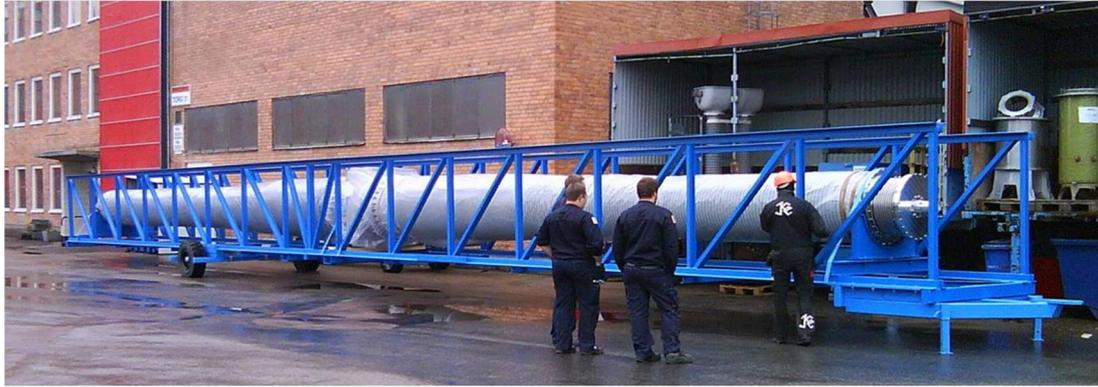
Figure 5. An UHVDC 1100 kV wall bushing
