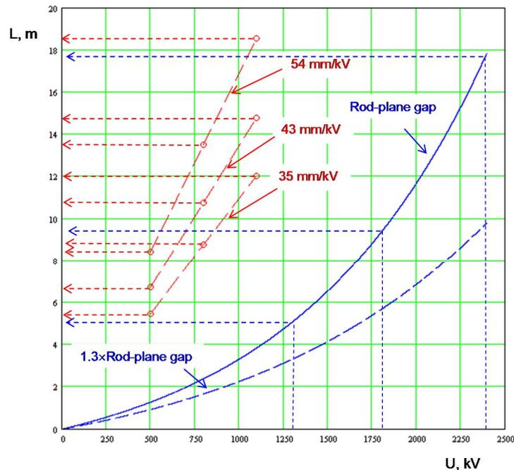
Figure 1. Insulator lengths determined by USCD for DC voltages of 500, 800 and 1100 kV (curves in red dash-lines); or by the  $U_{50}$  of SI of 1300, 1800 and 2390 kV respectively (curves in blue lines).
