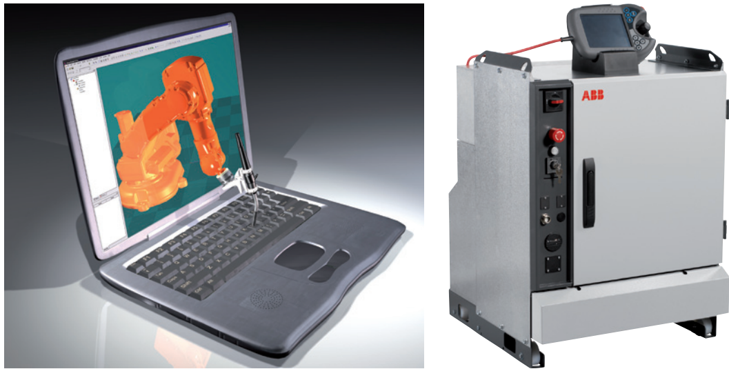
Fig 12: Tools like ABB's PickMaster Software and IRC5 Controller greatly simplify pick-on-the-fly programming
