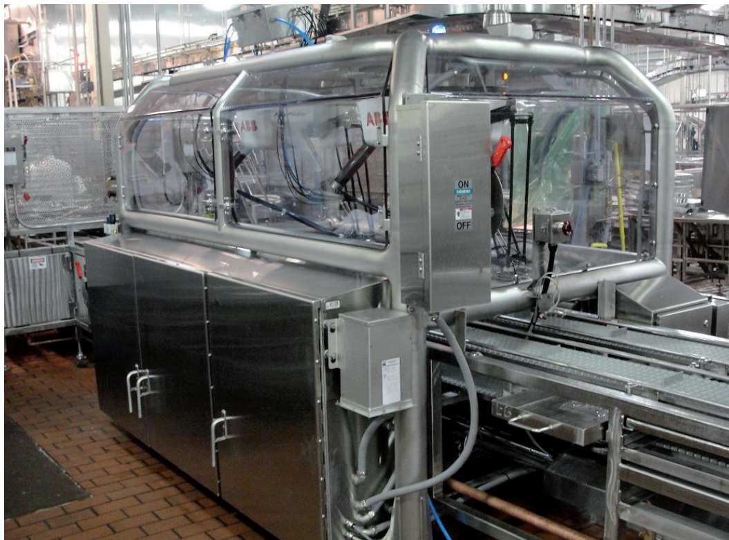
Fig 10: ABB's IRB 360 FlexPicker Delta style robot comes in an IP69K wash down model
