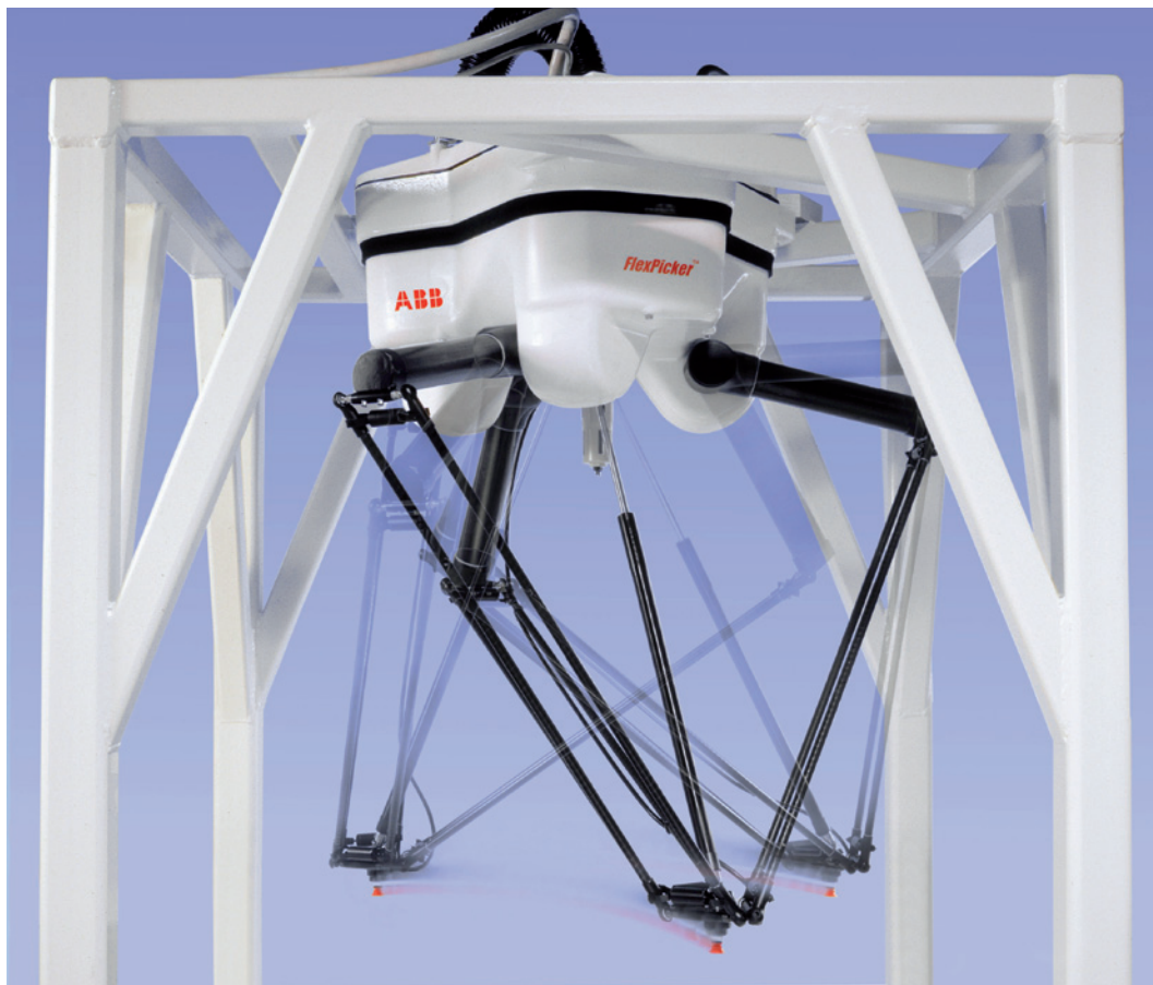
Fig 9: The Delta style robot was introduced in the late 1990s, delivering 120 to 150 pick and place cycles per minute.
