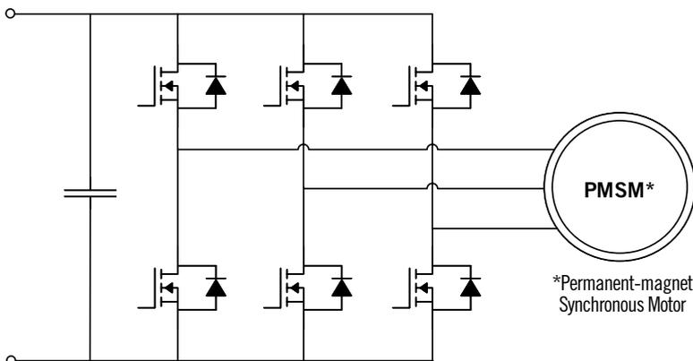
FIGURE 3 Schematic structure of a two-level converter (© ABB)
