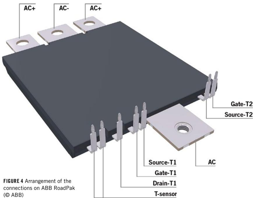
**FIGURE 4** Arrangement of the connections on ABB RoadPak (© ABB)
