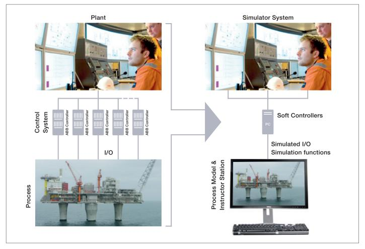
With 800xA Simulator, it is possible to create a simulator system of the running plant with identical layout, view and control logic. The control system runs on more cost and space efficient hardware, disconnected from the real process. A dynamic process model simulates the process and I/O signals. An external process model environment can connect to 800xA Simulator.
