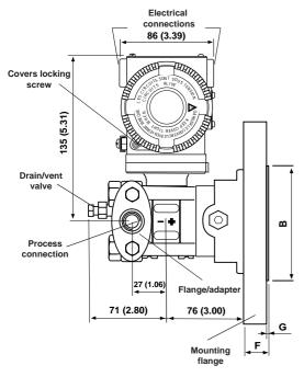
NOTE: On low pressure side, process connection, gasket groove and gaskets are in accordance with DIN 19213. Bolting threads for fixing adapter or other devices (i.e. manifold etc.) on process flange is 7/16"-20 UNF.
