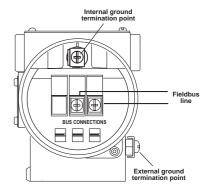
HART hand-held communicator may be connected at any wiring termination point in the loop, providing the minimum resistance is 250 ohm. If this is less than 250 ohm, additional resistance should be added to allow communications.
