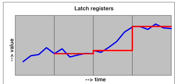
Figure 7.1 Sample and Hold registers, or 'Latches'
