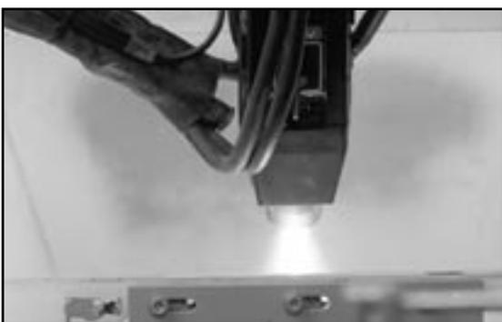
5. Applying an insulating and passivating layer on the cylindrical surface and of metal electrodes on the flat surfaces.
