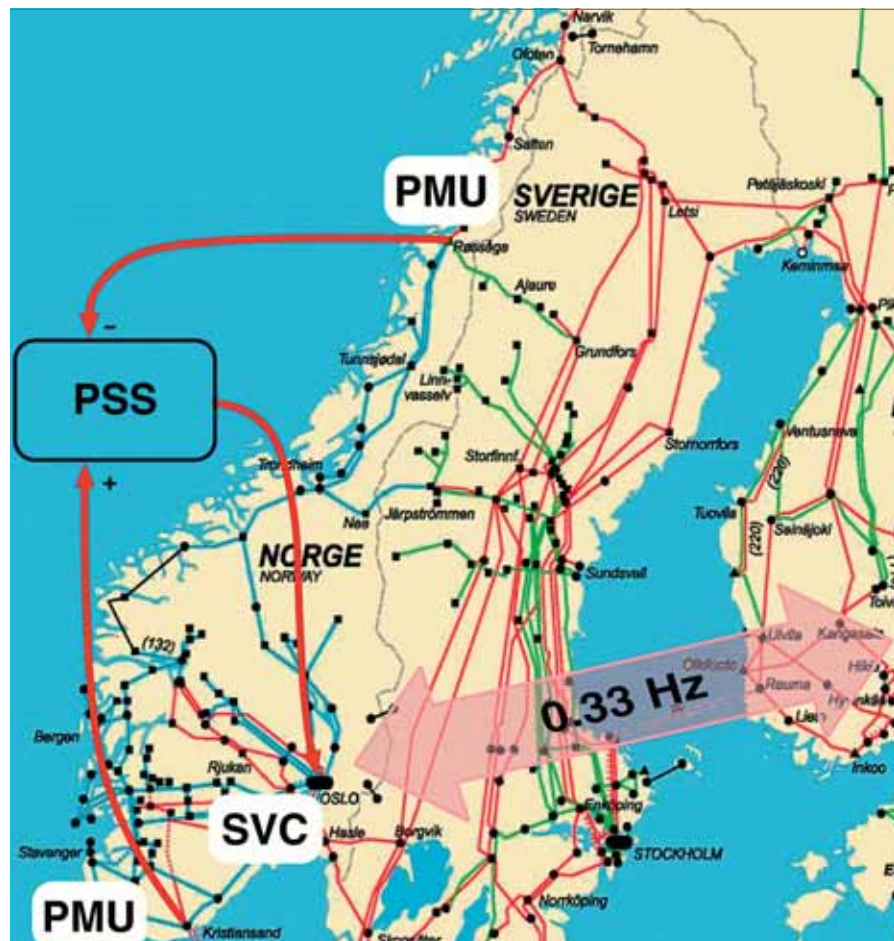
5 Controller tuning for 0.33 Hz mode regulating the SVC in Sylling using angle measurements from Nedre Røssåga and Kristiansand
