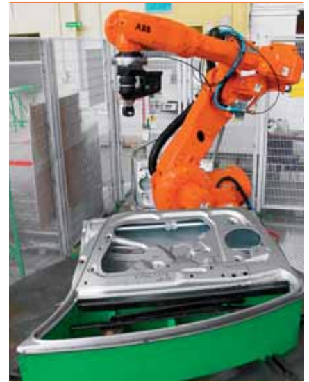
1 Spot-welding robot in car manufacturing
