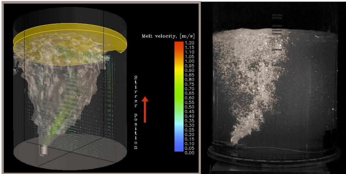
Figure 8. CFD simulation (left) and water modeling (right) results for EMGAS stirring in ladle furnace [11]
