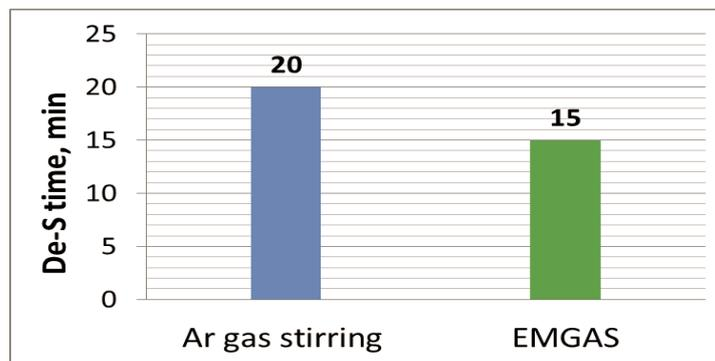
Figure 12. De-sulfurization time needed for sulfur reduction from 47 ppm to 7 ppm under Ar-gas and EMGAS stirring for a 150t ladle furnace
