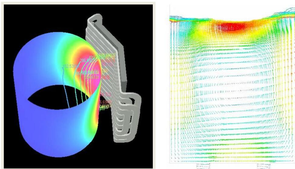
Figure 1. The 3D calculation of electromagnetic forces in a ladle installed with EMS (left) and the CFD velocity distribution in the melt (right)
