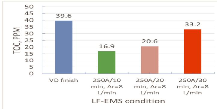
Figure. 4 The effect of soft EMGAS stirring time on the total oxygen removal in ladle refining
