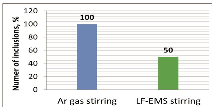
Figure 7 Number of non-metallic inclusions after EMS respective Ar gas stirring in the ladle furnace
