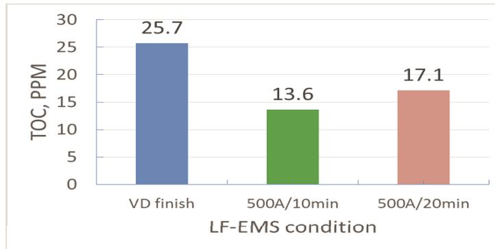
Figure. 5 The effect of EMS soft stirring time on the total oxygen removal in ladle refining
