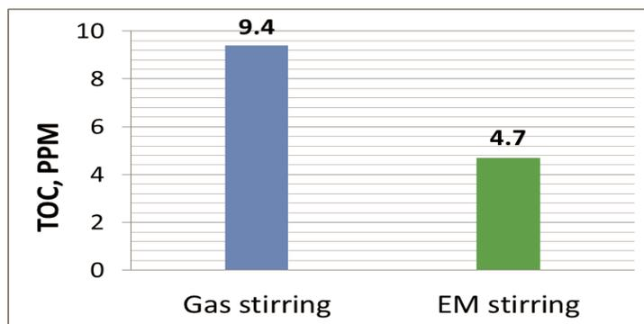
Figure 6. Total oxygen content in ball-bearing steel produced with gas and electromagnetic stirring respectively
