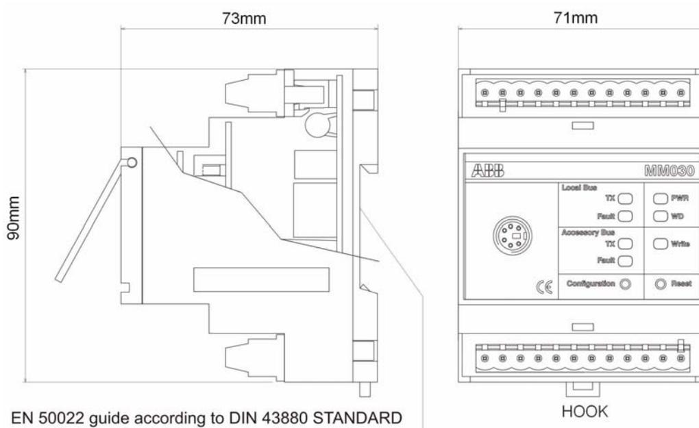
Figure 15. MM030 and Accessory Devices dimensions
