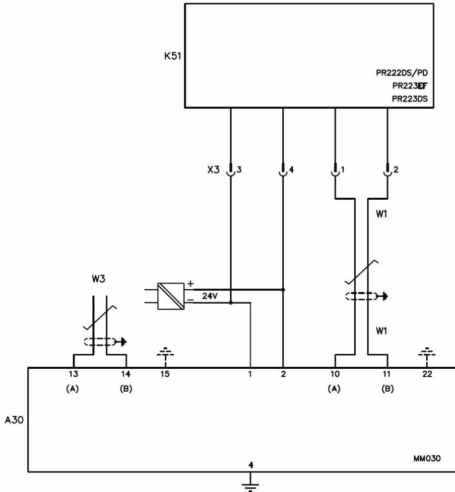
Figure 21. MM030 with PR222DS/PD and PR223 trip units circuit diagram
