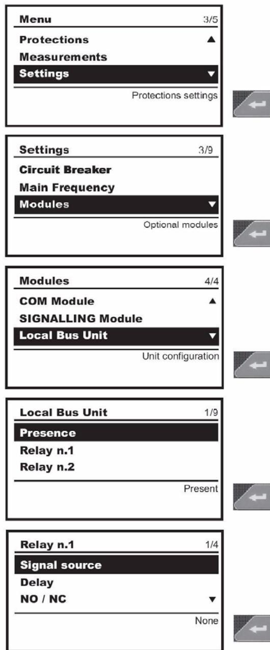
Figure 11. Trip unit local display menu for setting user-defined signalling
