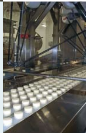
At Ilchester Cheese, an IRB 340 picks the cheese with the help of a vision system that allows it to move at lightning speed.
