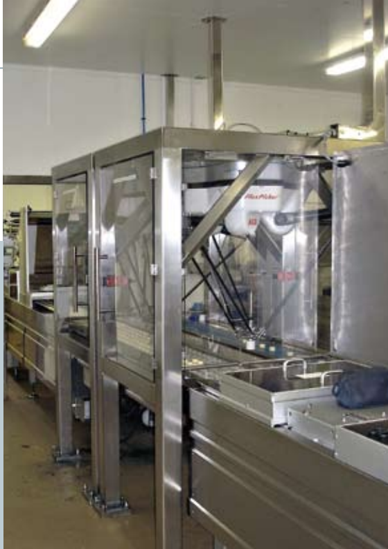
At Ilchester Cheese, an IRB 340 picks the cheese with the help of a vision system that allows it to move at lightning speed.
