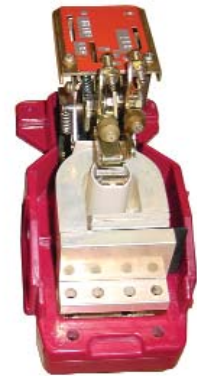
OD device after replating
