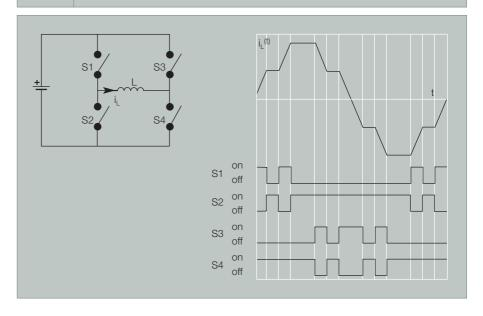
power depends heavily on the switched current and on the pulse rate, and is typically of the order of 10 to 50 watts.
