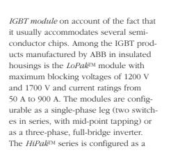
single switch with ratings from 1200 V / 3600 A over the voltage classes 1700 V, 2500 V, 3300 V, up to 6500 V / 600 A.
