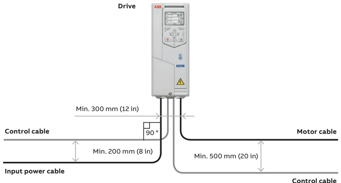
08 Fig. Running different cable types in cable trays.
