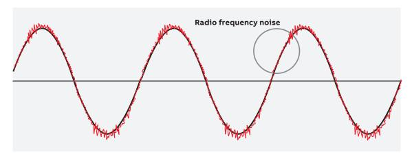
04 Fig. Mechanisms of EM disturbances transfer. The electromagnetic noise is usually stronger at positive and negative peaks of the sine wave where line voltage reaches the highest value.
