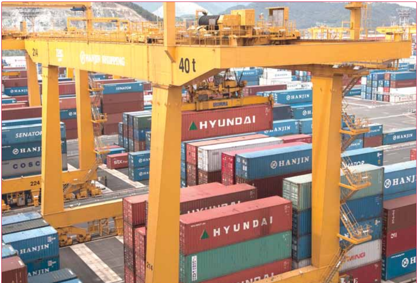
Figure 1. A cantilever automatic stacking crane in operation.
