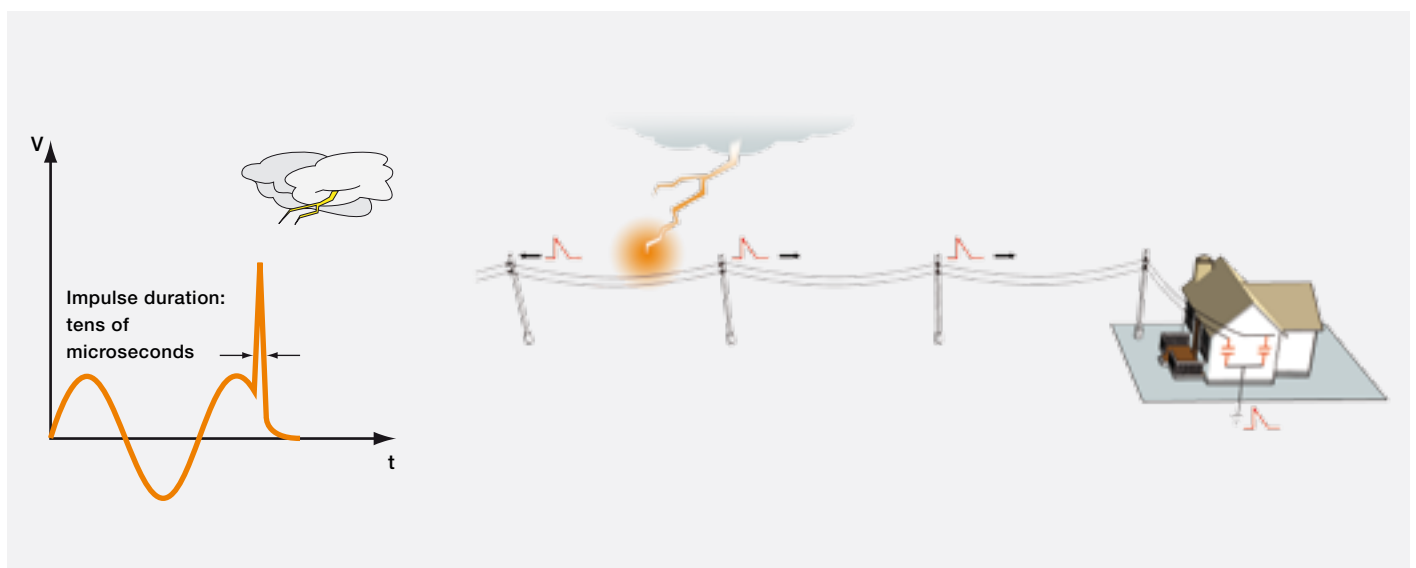
01 Atmospheric overvoltages are caused by indirect lightning strikes on power lines
