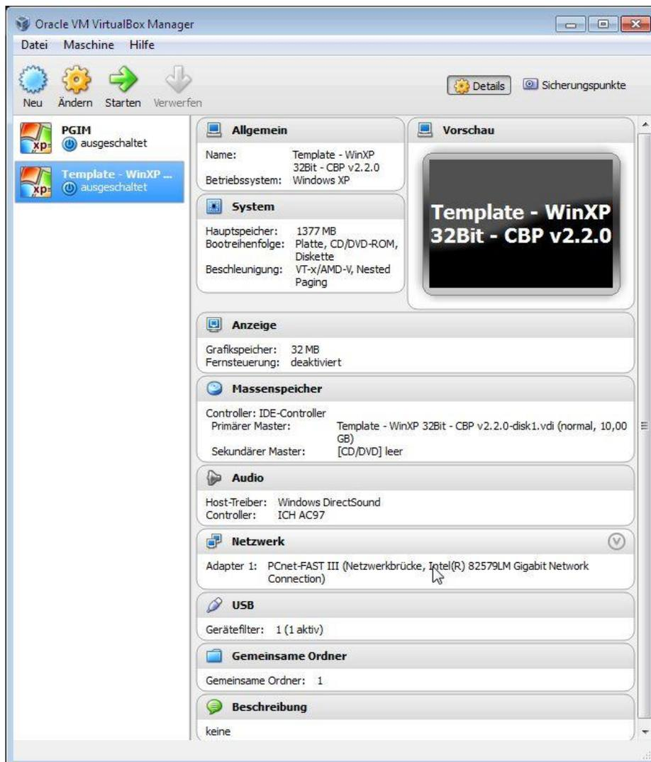
Network setting: Using the Ethernet adapter of the host as network bridge.
