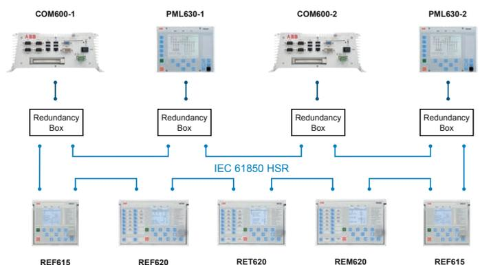
Figure 2. PML630 HSR solution
