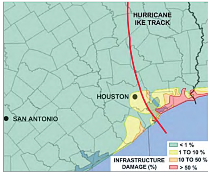
Figure A4-6 – Power grid damage from records obtained with field damage assessments [24]
