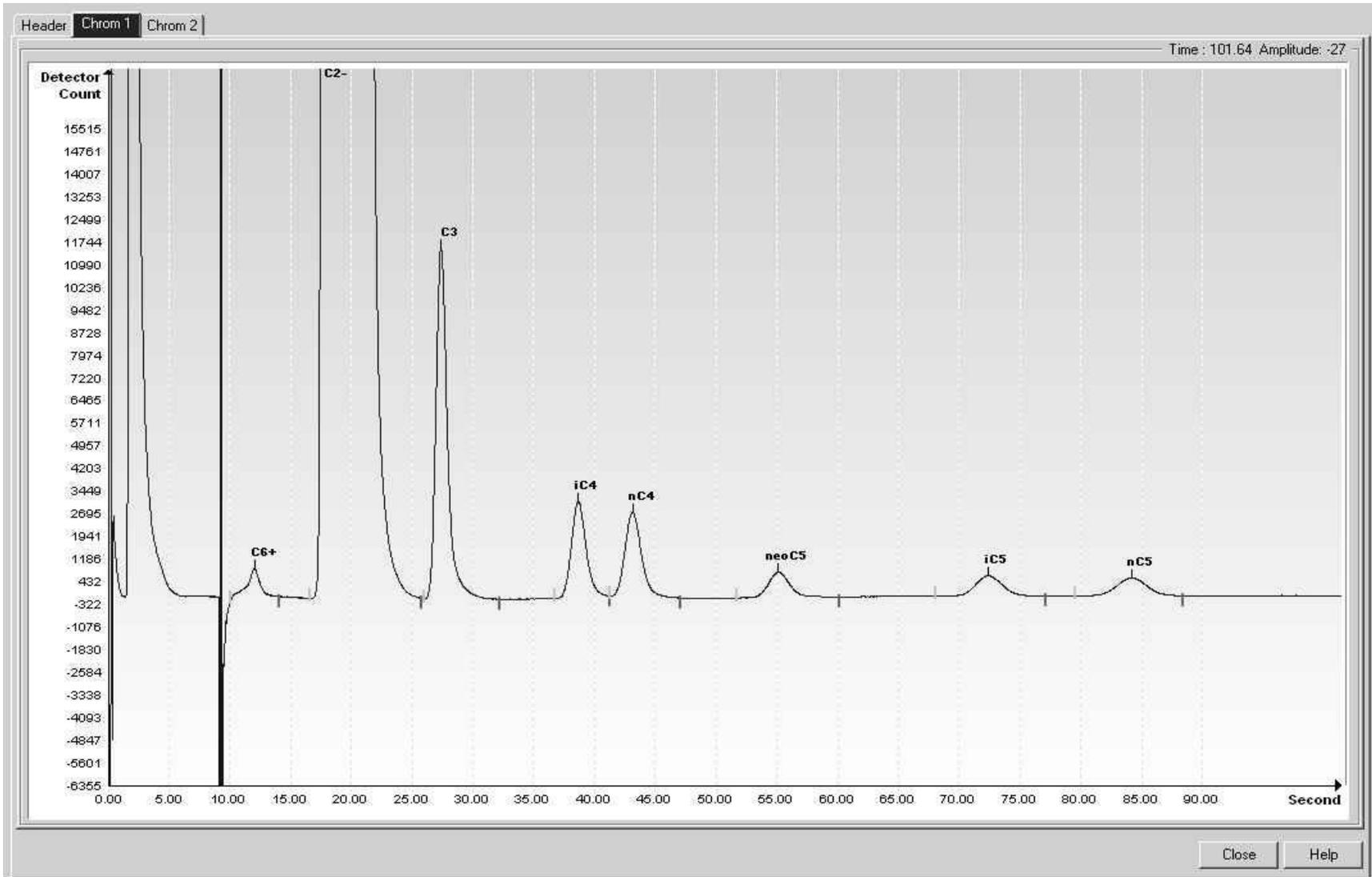
Figure 7-13 BCD Hydrogen Reference Chromatogram
