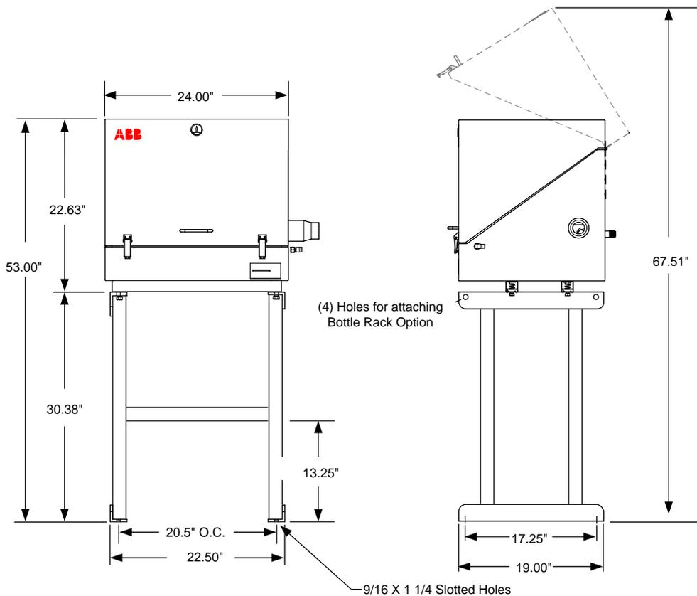
**Figure 2-7 ENC82S–Enclosure Installation**
