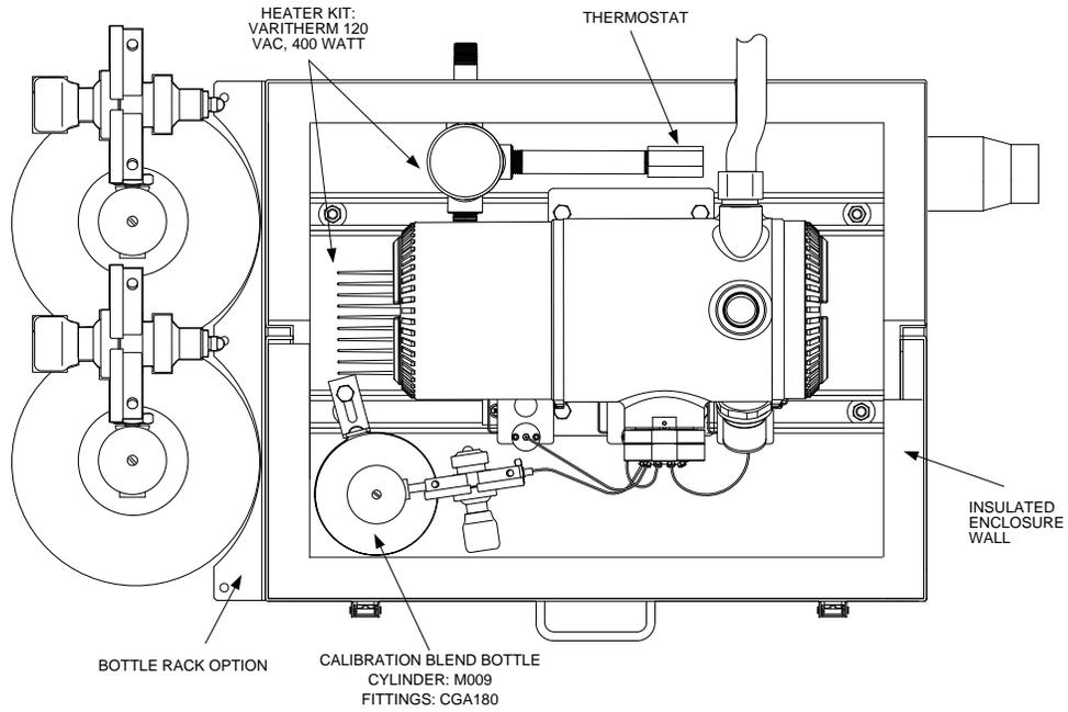
**Figure 1-22 ENC82S Environmental Enclosure with Electric Heater**
