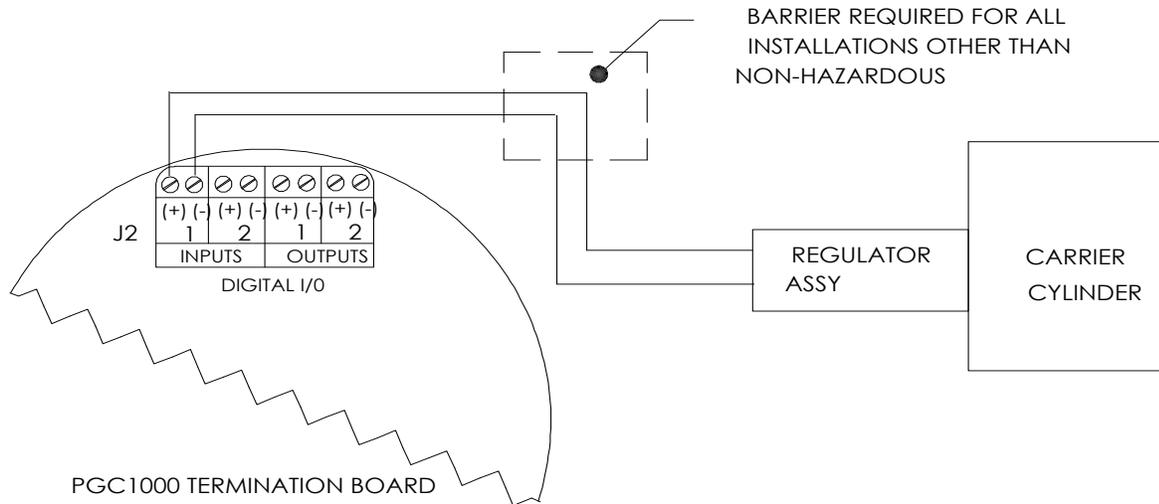
**Figure 2-40 Carrier Gas Low Pressure Switch Wiring Instructions**
