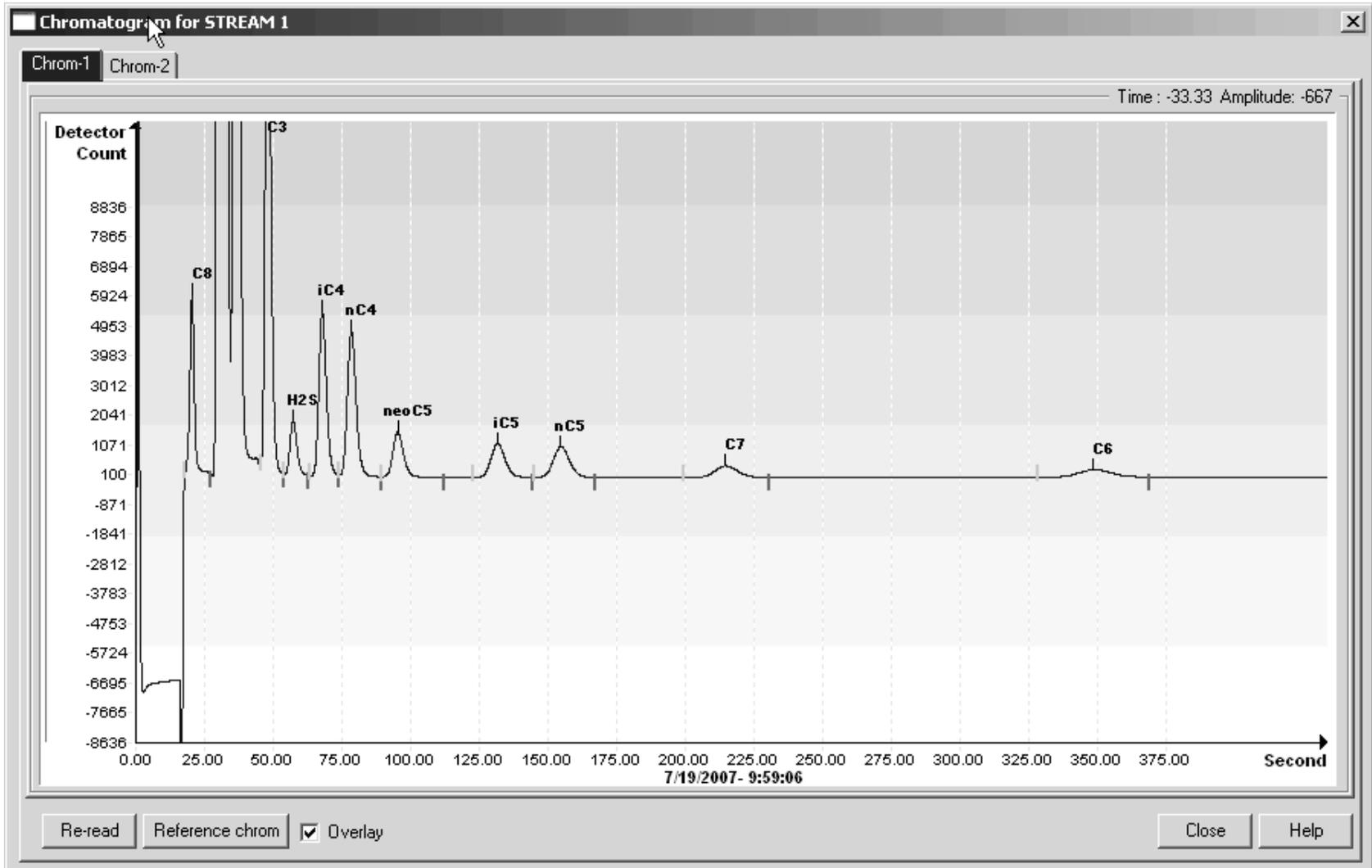
Figure 7-16 BCH Helium Reference Chromatogram
