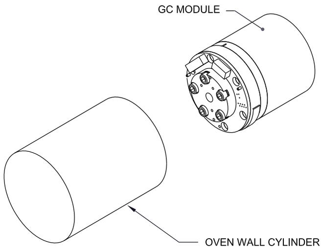
**Figure 1-12 GC Module Assembly**
