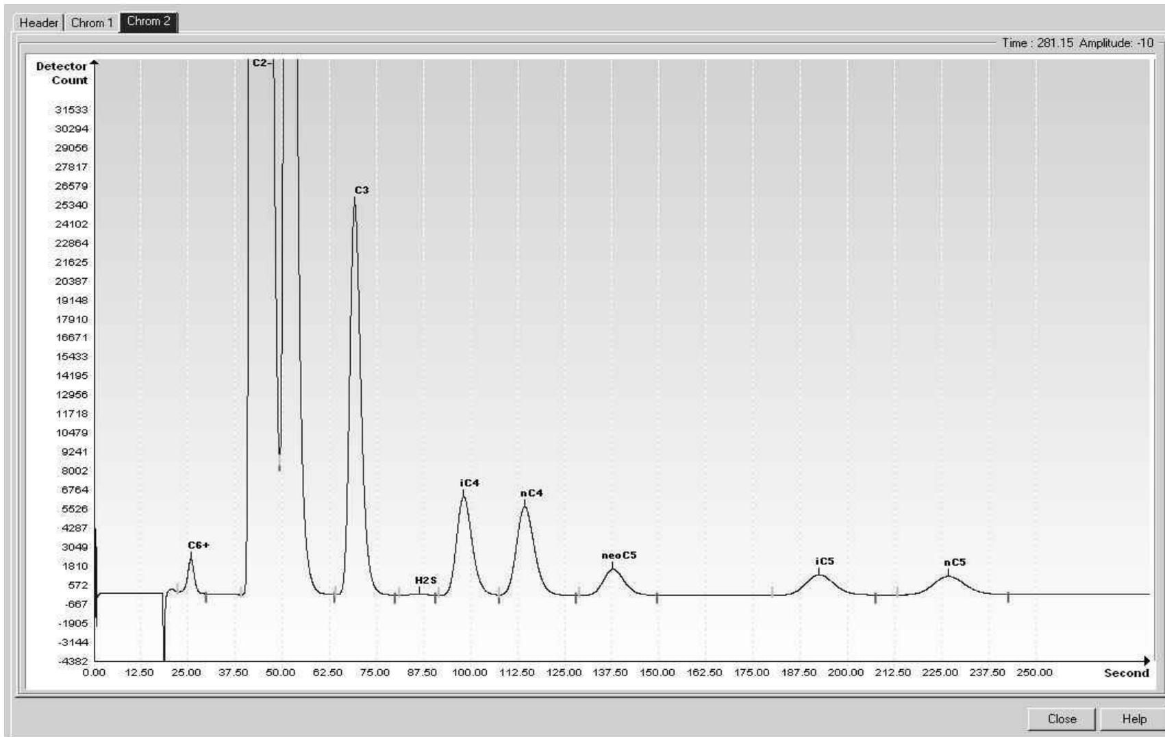
Figure 7-6 BBM Helium Reference Chromatogram
