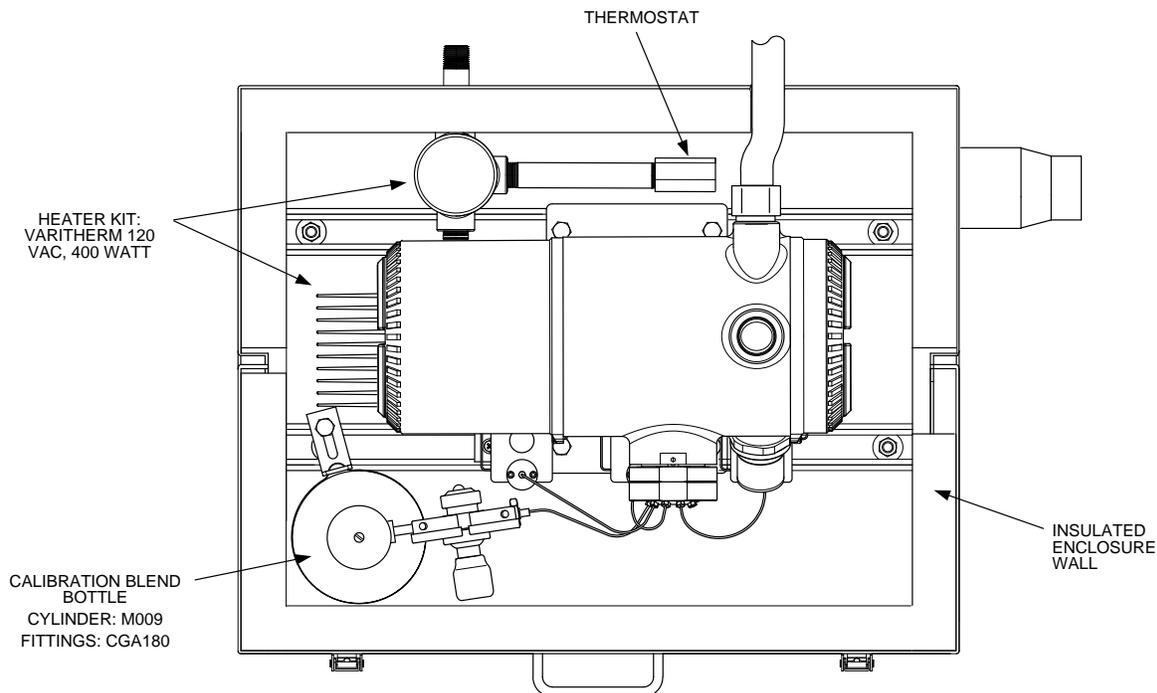
**Figure 2-56 ENC82S Electric Heater Installed in Enclosure**
