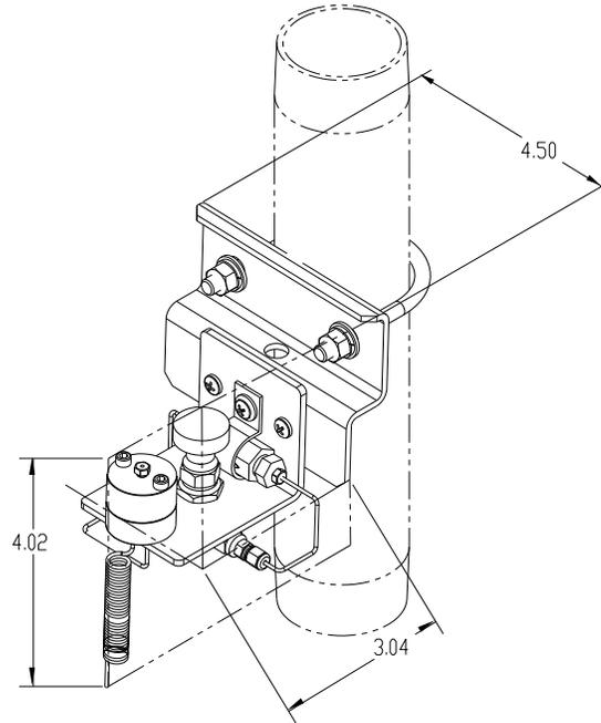
**Figure 1-26 Single Stream Conditioning Module Dimensions**
