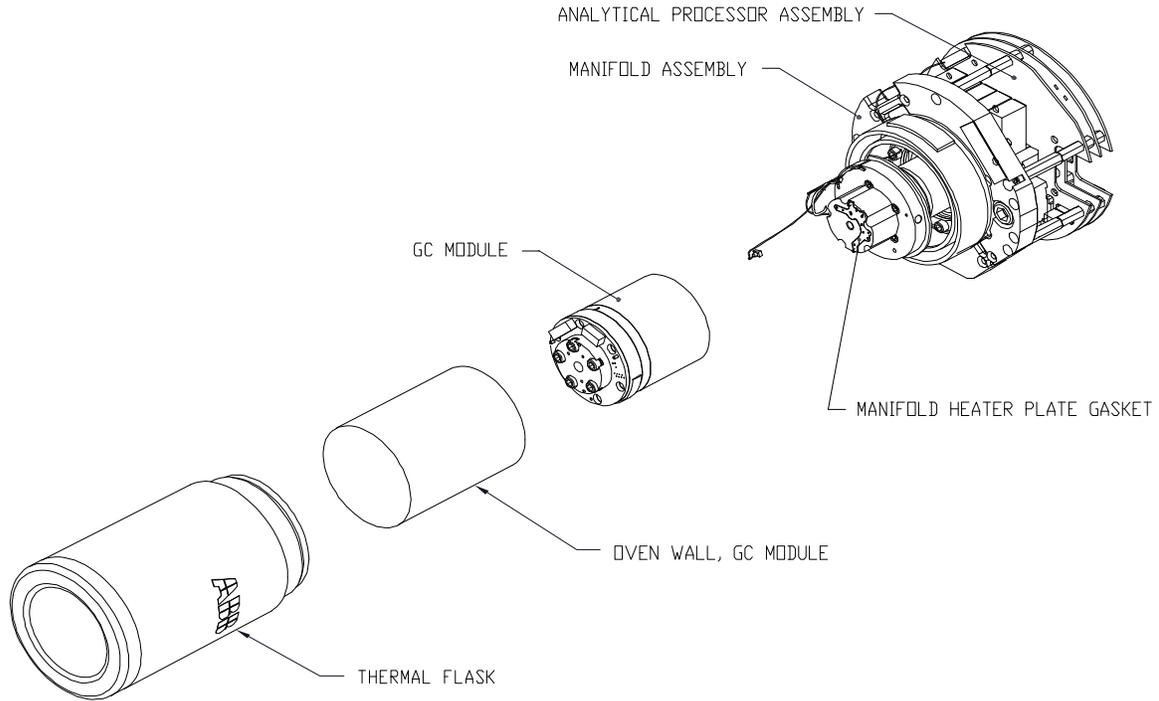
**Figure 4-8 GC Module, Exploded View**
