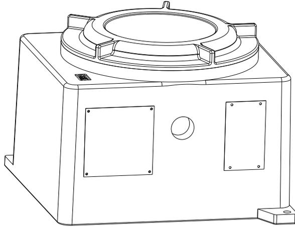
**Figure 1-32 Explosion Proof AC Power Supply**
