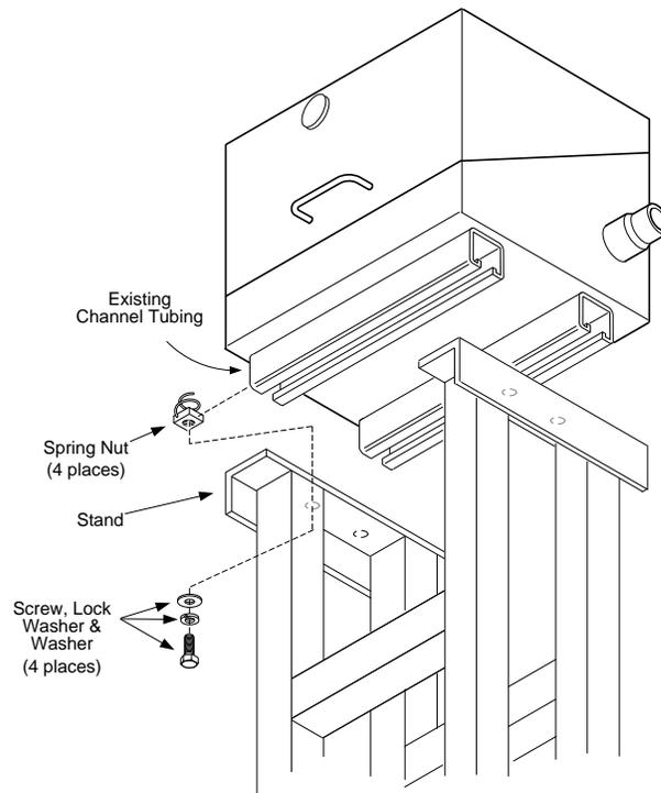
**Figure 2-8 ENC82S–Enclosure Mounting Hardware**
