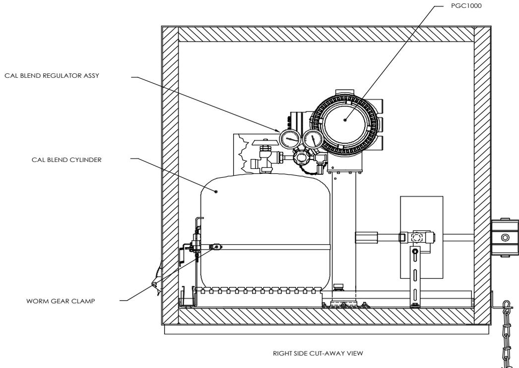
**Figure 2-41 Calibration Bottle Location**
