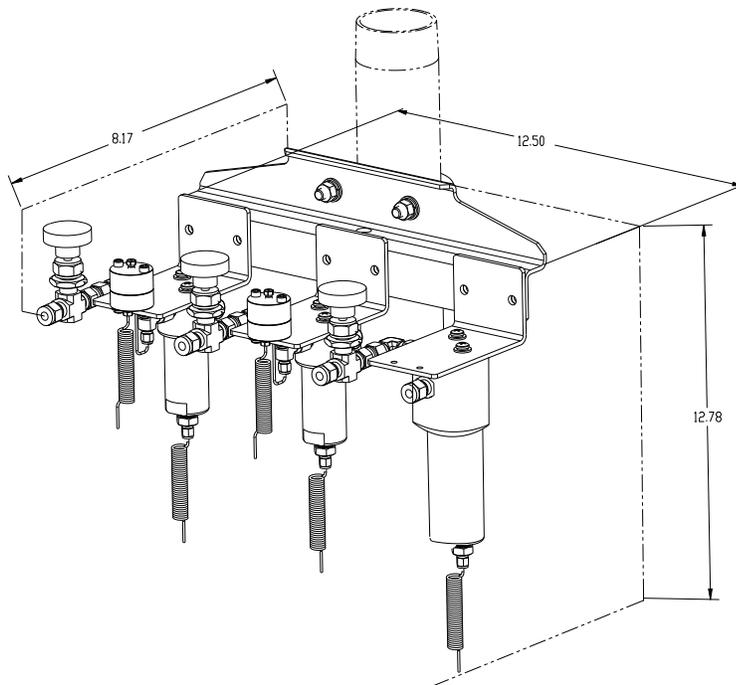
**Figure 1-27 Multiple Stream Conditioning Module Dimensions**
