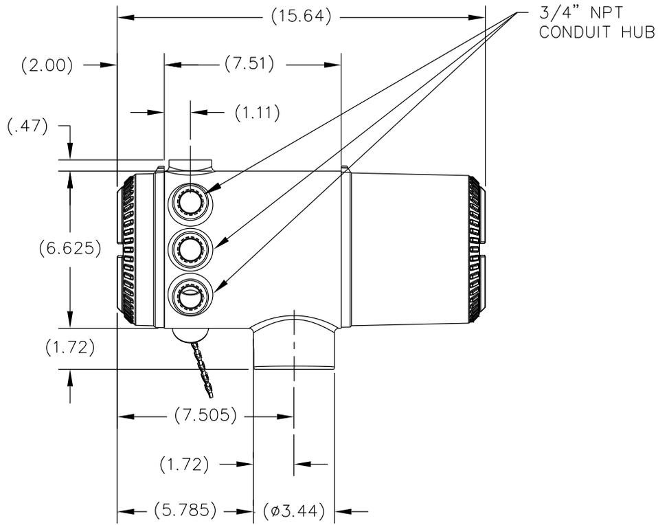
**Figure 1-5 PGC1000 Enclosure Left Side**
