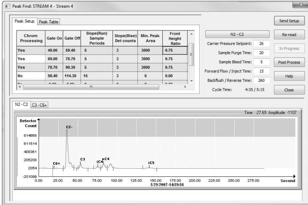
Figure 6-12 Manual Peak Find Setup Screen
