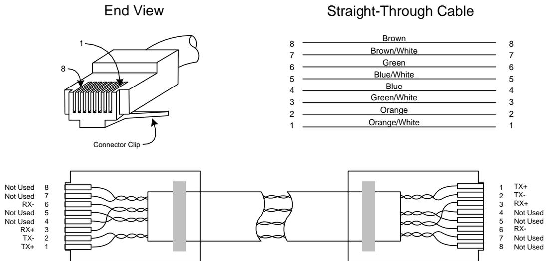
**Figure 3-2 Ethernet Cable-Typical**
