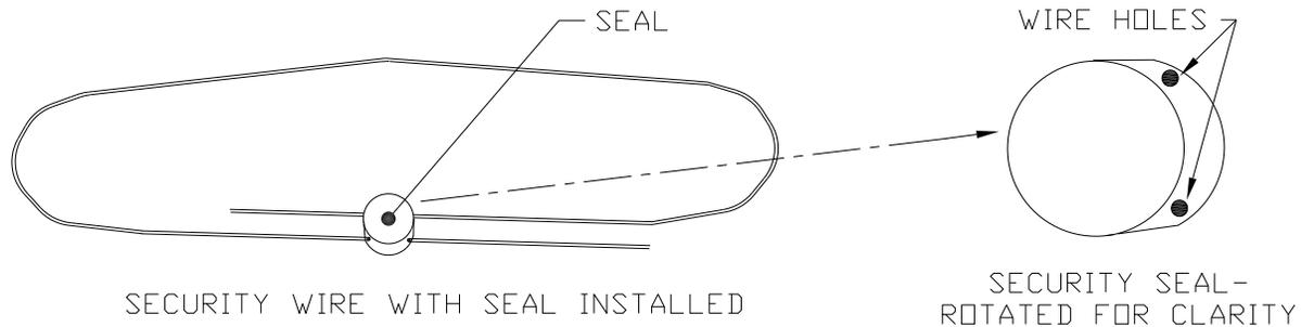
**Figure 1-29 Security Wire with Seal**
