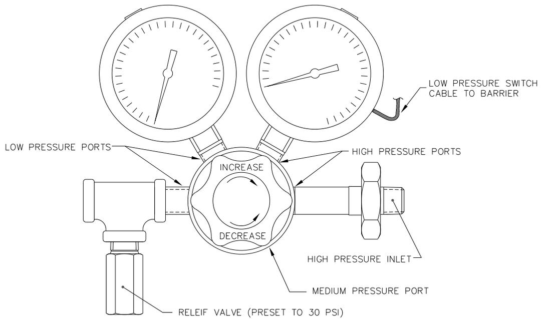
**Figure 2-43 Calibration Gas Pressure Regulator with Relief Valve**
