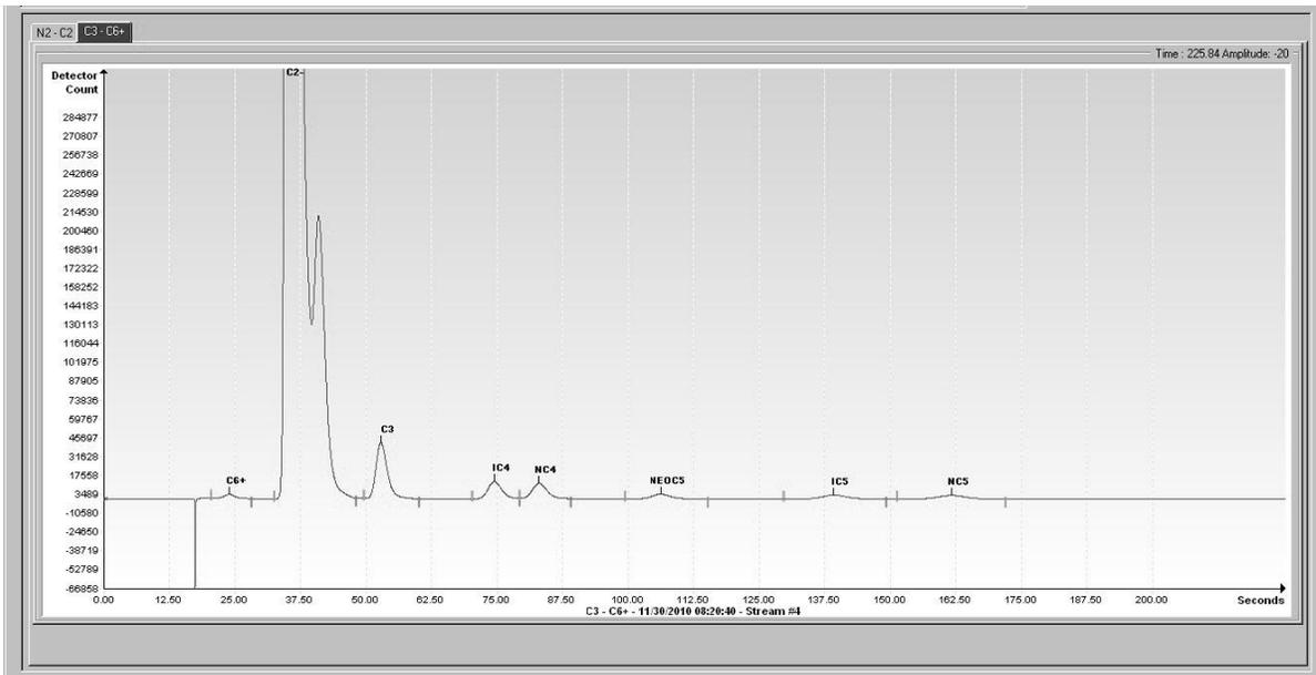
**Figure 6-15 Run Cycle Chromatogram**
