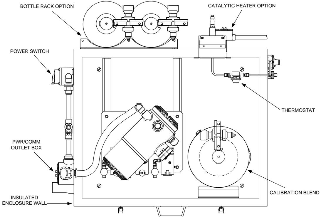
**Figure 1-21 ENC82L Environmental Enclosure with Catalytic Heater**
