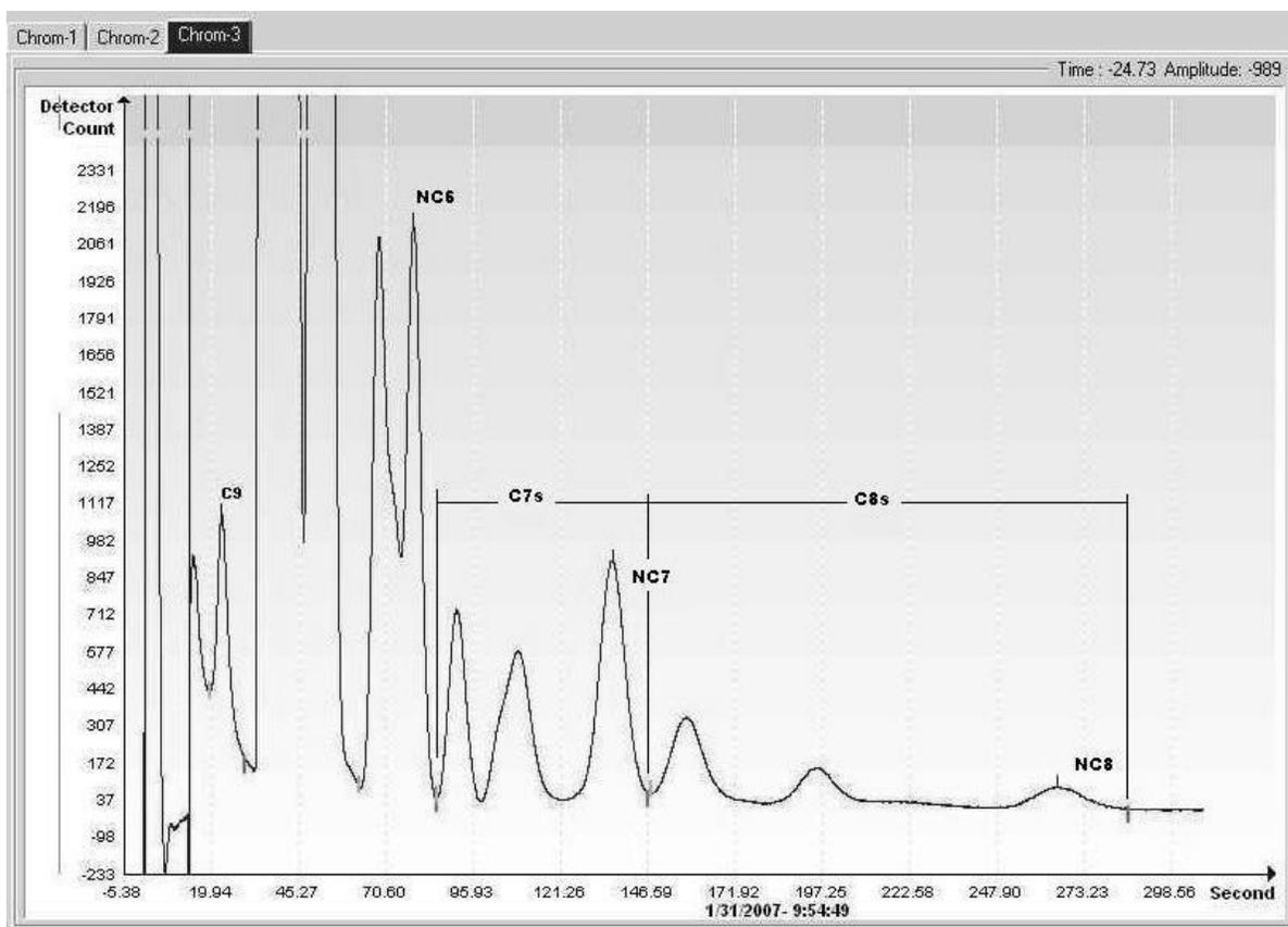
**Figure 6-13 Example of a C9+ Chromatogram**
