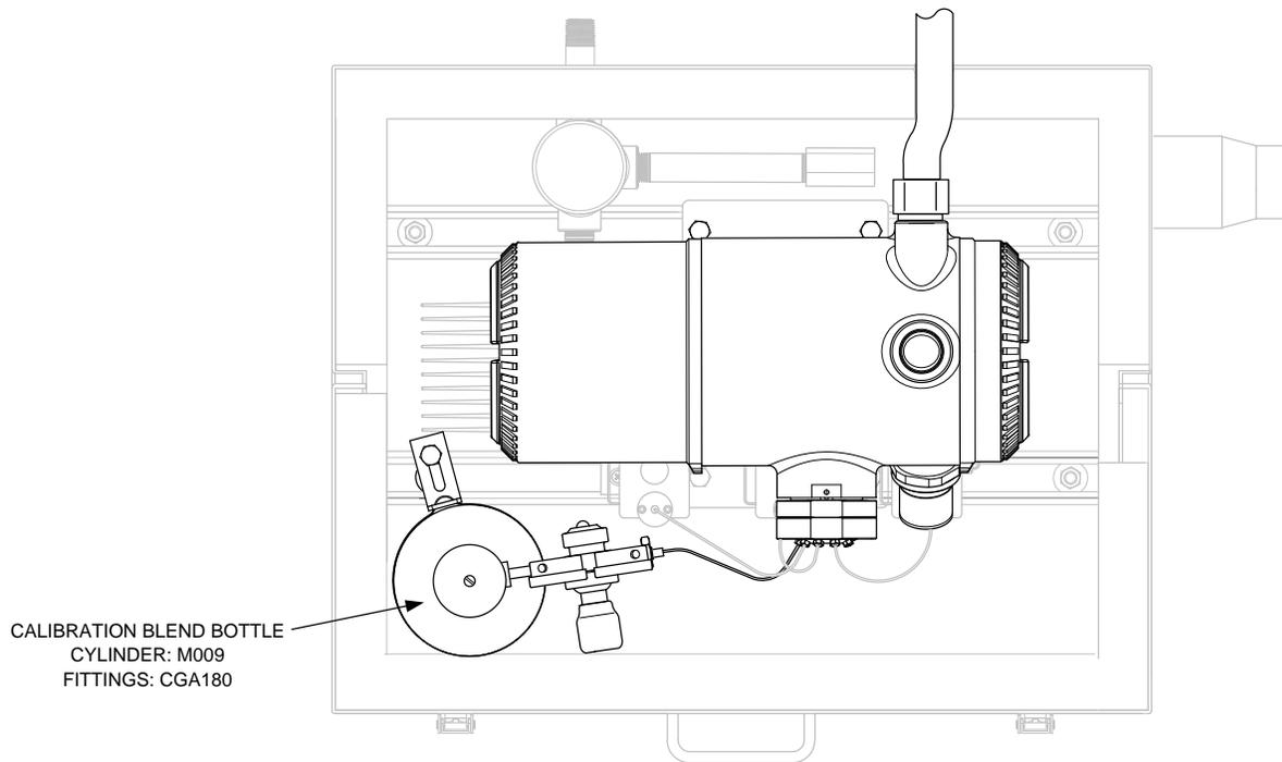
**Figure 2-42 Calibration Bottle Location**
