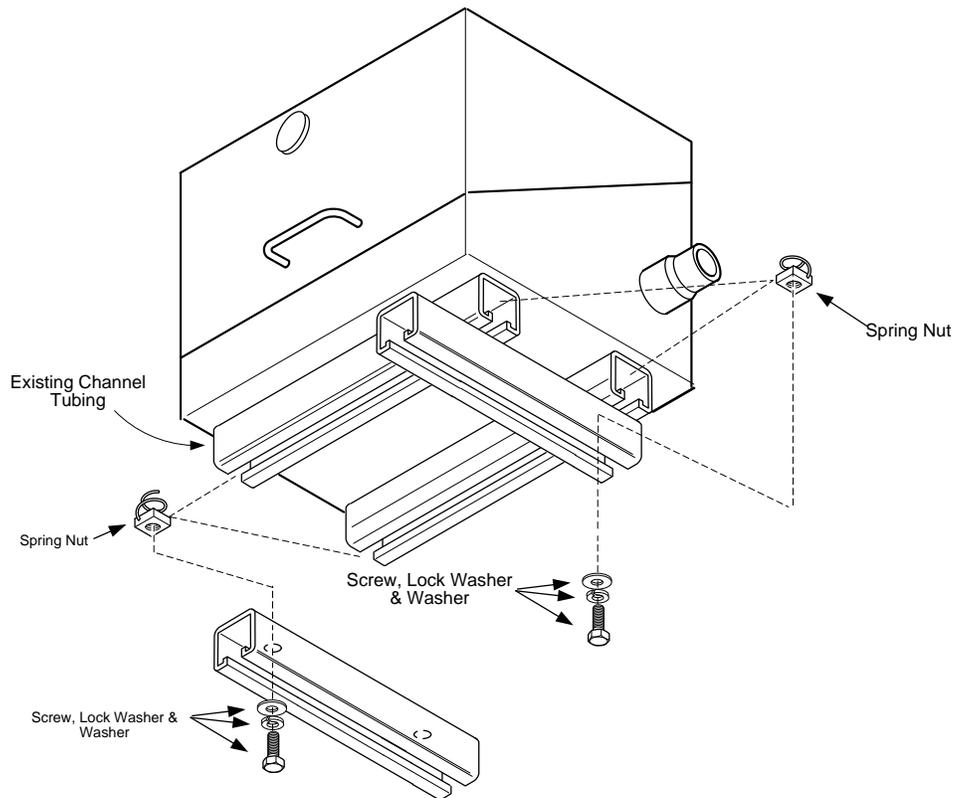
**Figure 2-15 ENC82S–Channel Tubing Installation**
