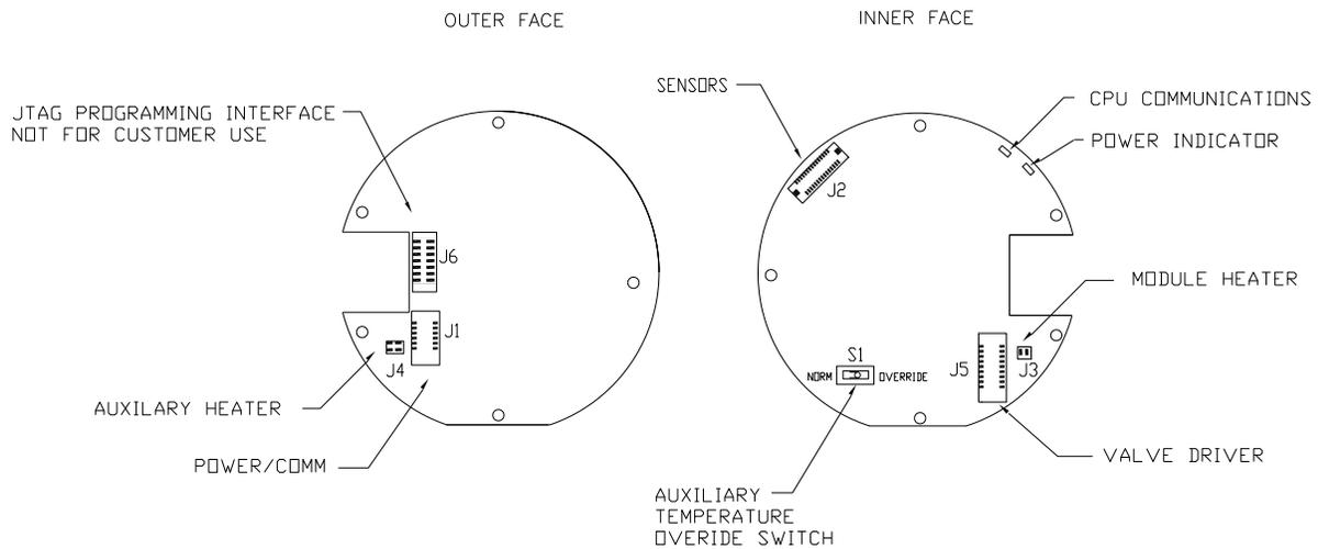
**Figure 4-7 Analytical Processor Board**
