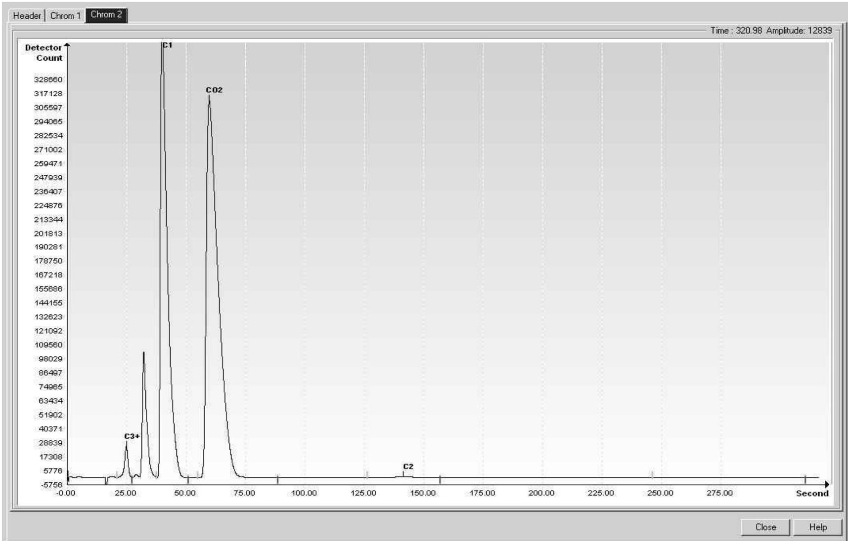
**Figure 7-11 BCB Helium Reference Chromatogram**
