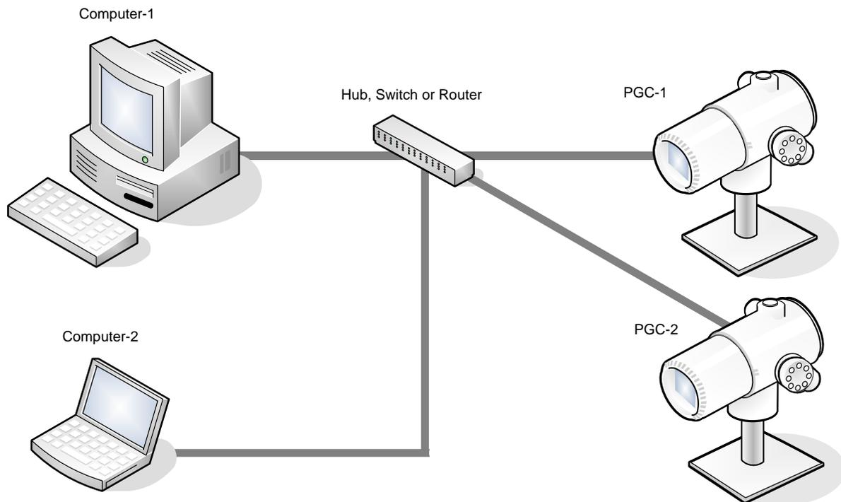
**Figure 3-1 Ethernet Connections**
