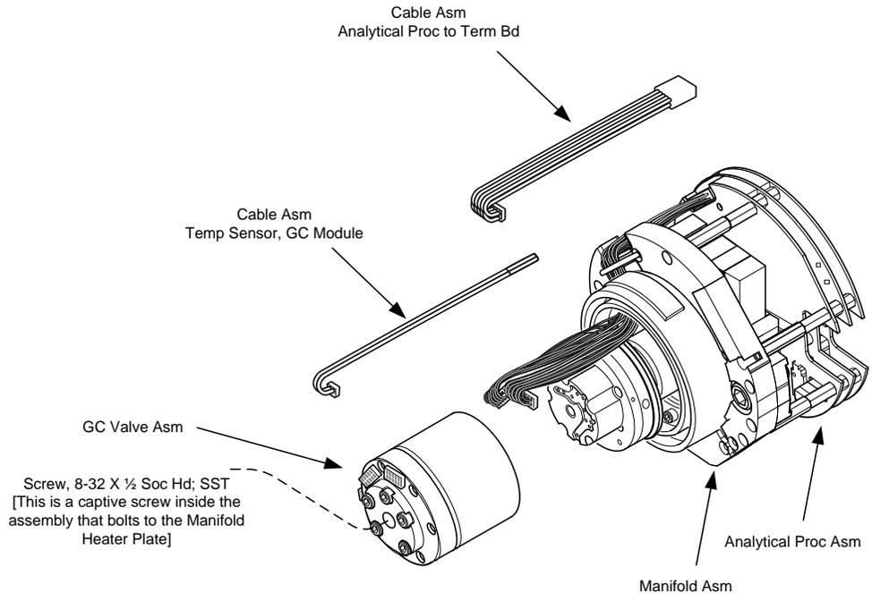
**Figure 4-2 Analytical Module View, Exploded**
