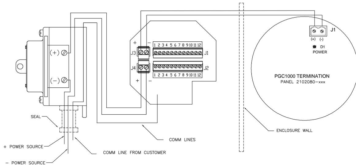
**Figure 2-31 Power Wiring Diagram**
