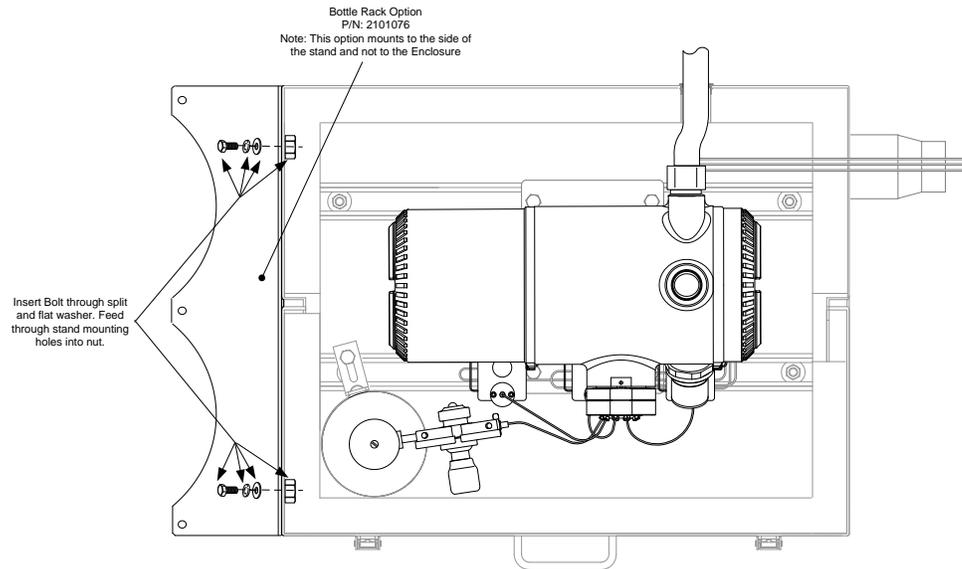
**Figure 2-38 ENC82S–Dual Bottle Rack Installation**
