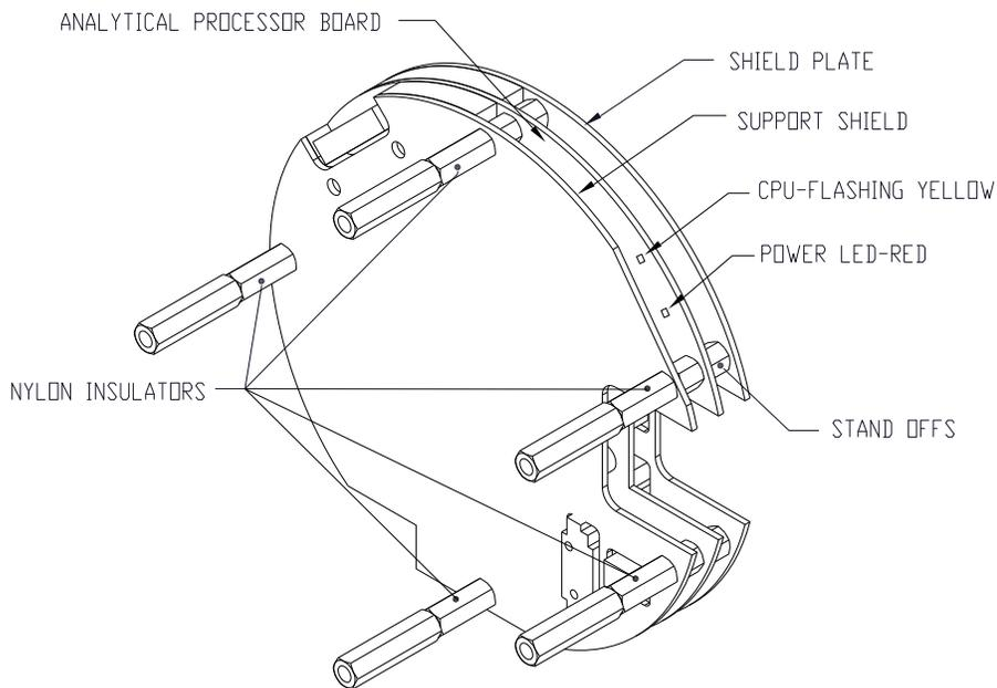
**Figure 1-11 Analytical Processor Assembly**
