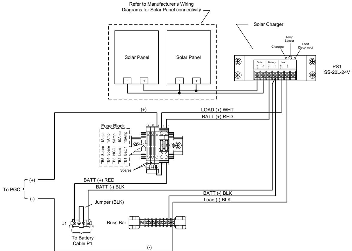
**Figure 5-3 Solar Panel Wiring Instructions**
