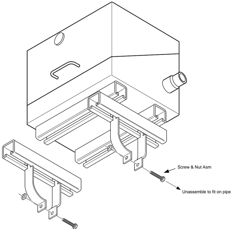
**Figure 2-17 ENC82S– Pipe-Mount Assembly**
