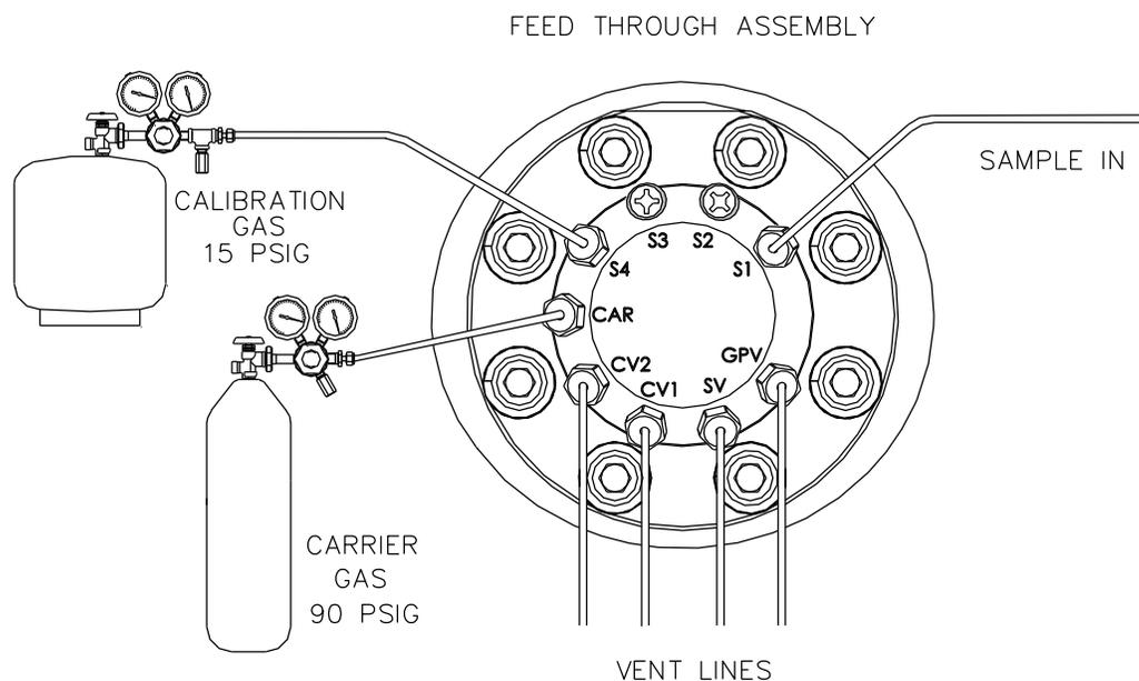
**Figure 2-46 Vent Line Connections on Feed-Through Assembly**
