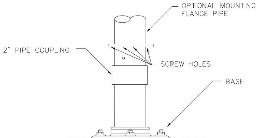
**Figure 2-22 PGC1000 Optional Mounting Flange Pipe**
