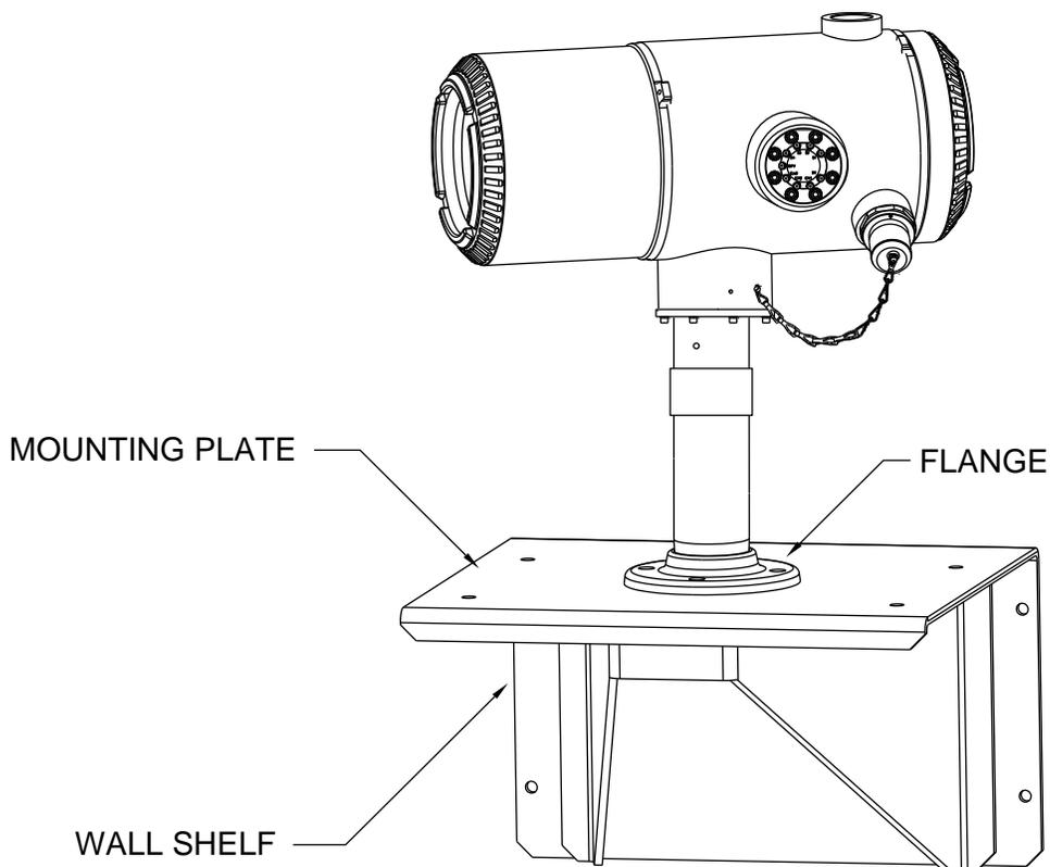
**Figure 2-2 Typical Wall Shelf Mount Installation**
