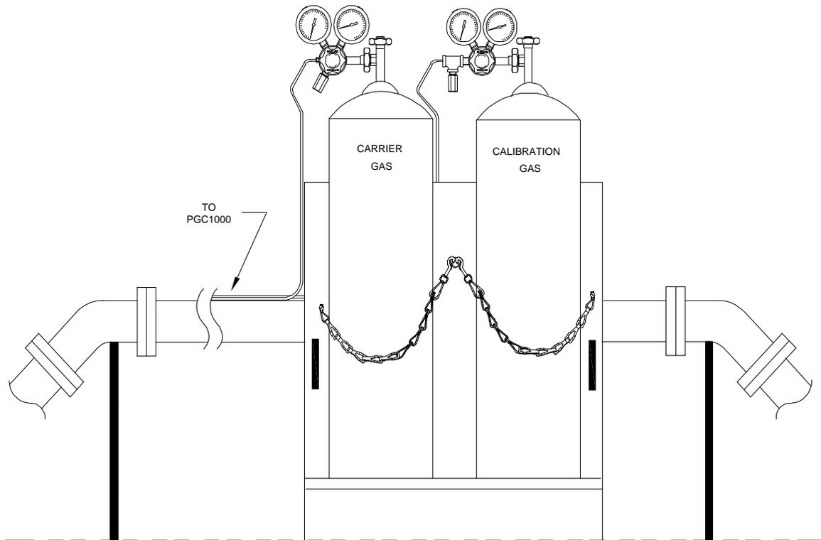
*Figure 2-35 Carrier/Calibration Gas Bottle Rack Installation*
