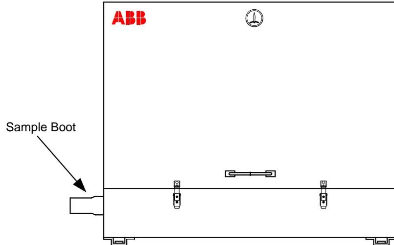
**Figure 2-26 ENC82L–Environmental Enclosure Sample Boot**
