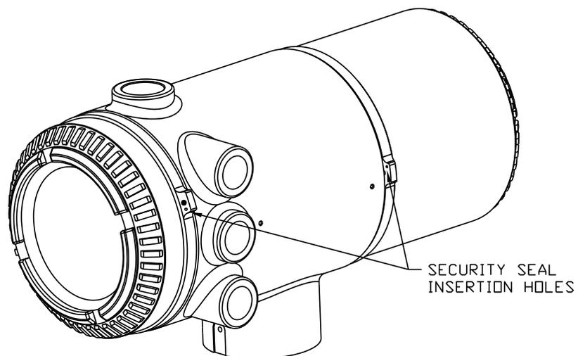
**Figure 1-28 PGC1000 End Cap Tabs for Security Seal**
