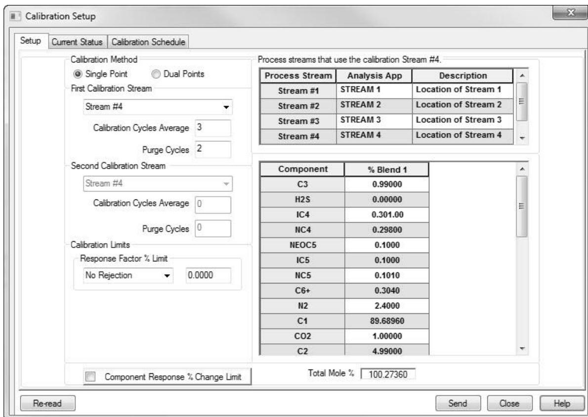
**Figure 6-20 Typical Calibration Setup for a C6+ Application**
