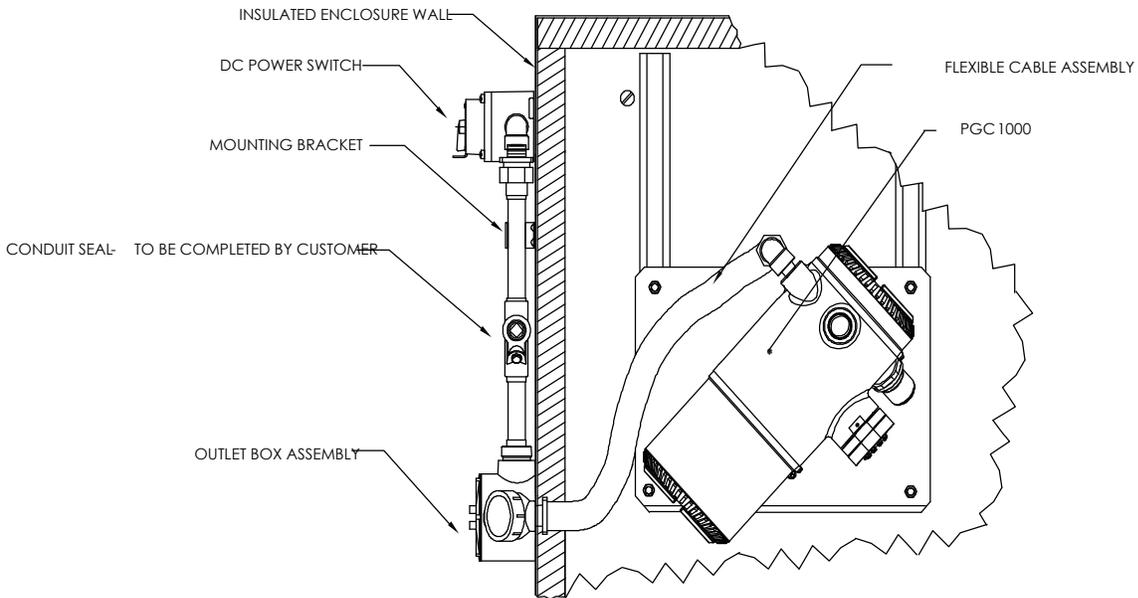
**Figure 2-30 Assembled Power/Communication Assembly**
