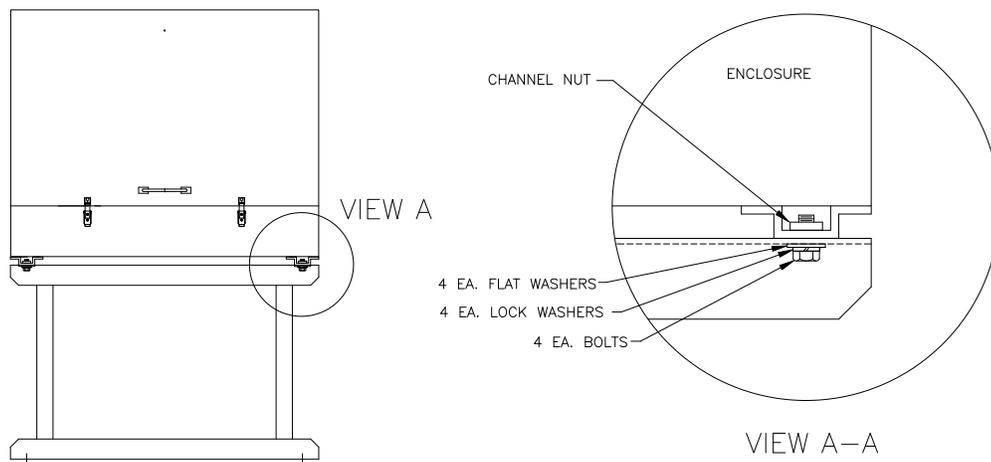
**Figure 2-6 ENC82L–Enclosure Mounting Hardware**
