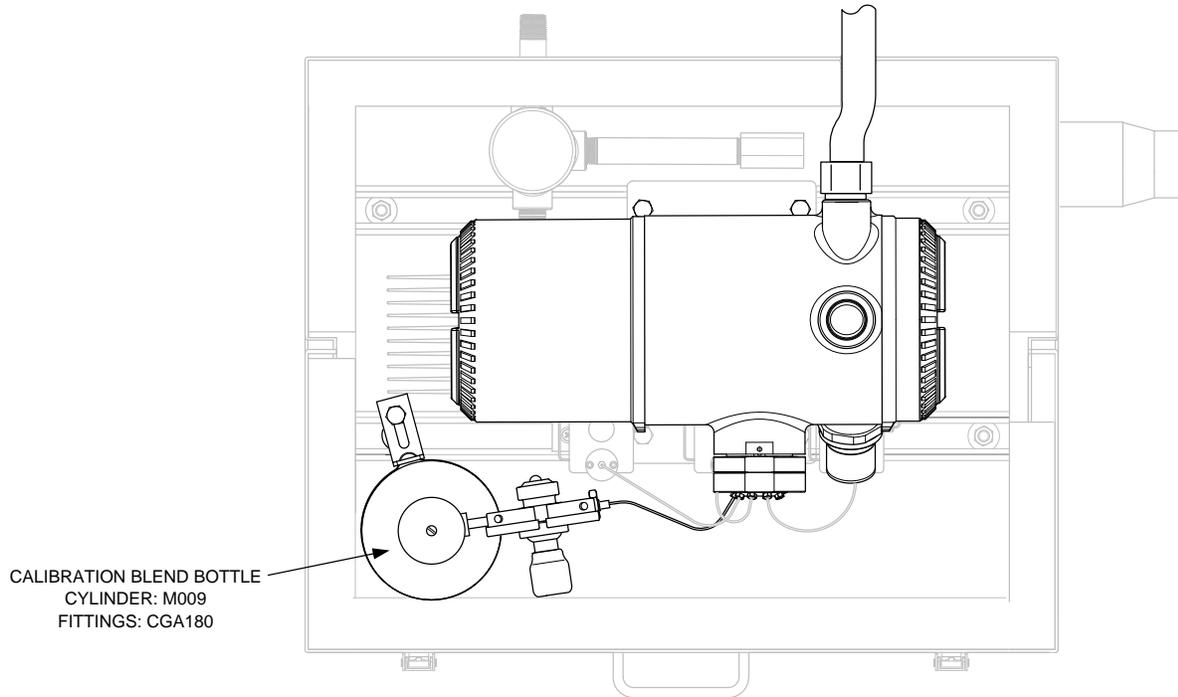
**Figure 2-42 Calibration Bottle Location**
