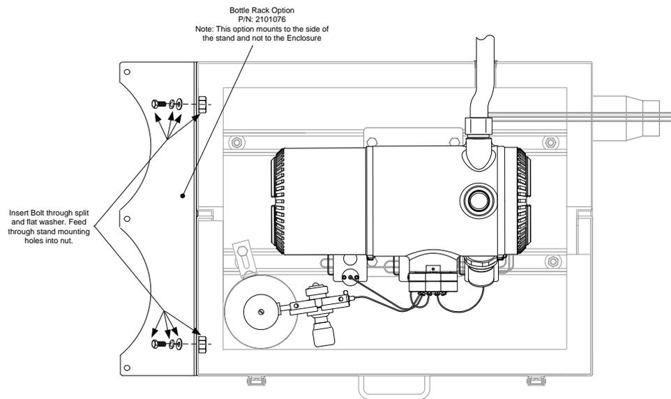
**Figure 2-38 ENC82S–Dual Bottle Rack Installation**
