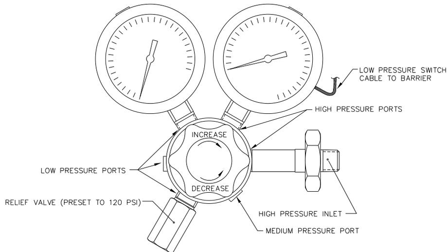
**Figure 2-39 Carrier Gas Pressure Regulator with Relief Valve**
