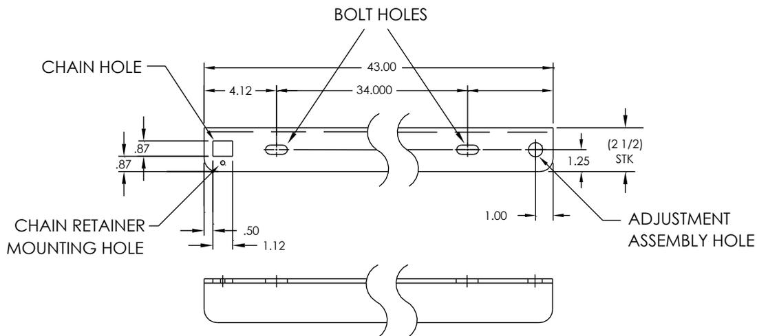
**Figure 2-9 ENC82L–Mounting Brackets**
