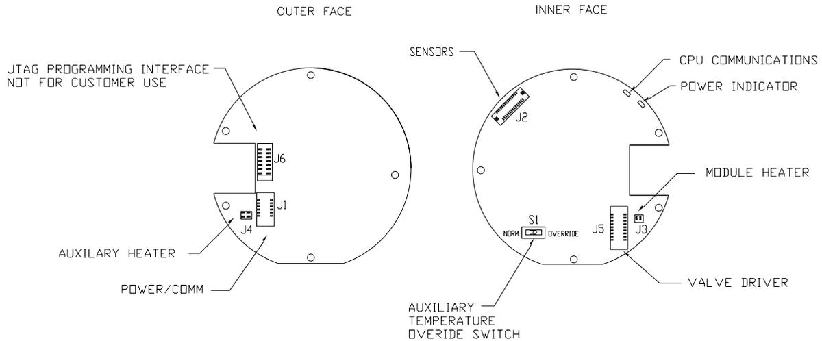
**Figure 4-7 Analytical Processor Board**
