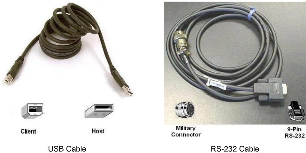
**Figure 3-4 MMI Communication Cables**
