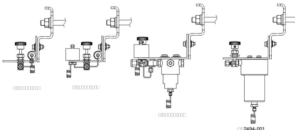
**Figure 1-24 Available Sample Conditioning Modules**
