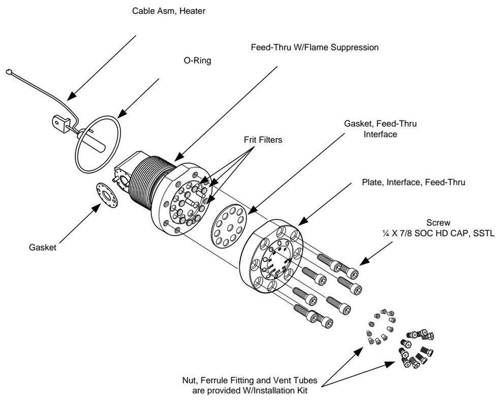
**Figure 4-3 Feed-Through Assembly**
