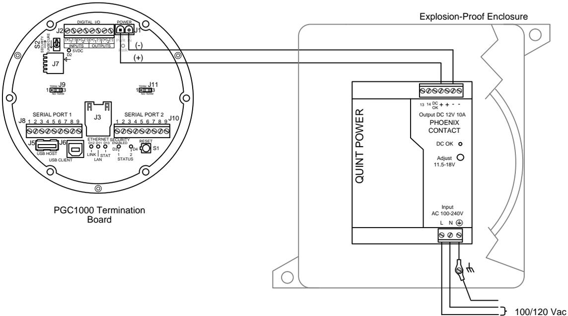
**Figure 2-68 Explosion-Proof AC Power Supply Wiring Instructions**
