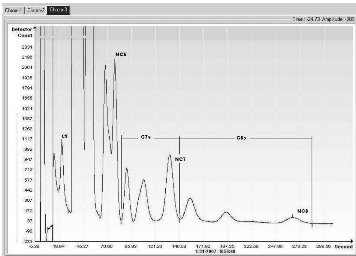
**Figure 6-13 Example of a C9+ Chromatogram**
