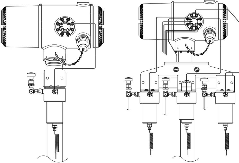
**Figure 1-25 Single and Multiple Stream Sample Conditioning Assemblies**
