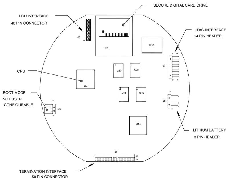
**Figure 4-11 Primary Component Side Digital Controller Board**
