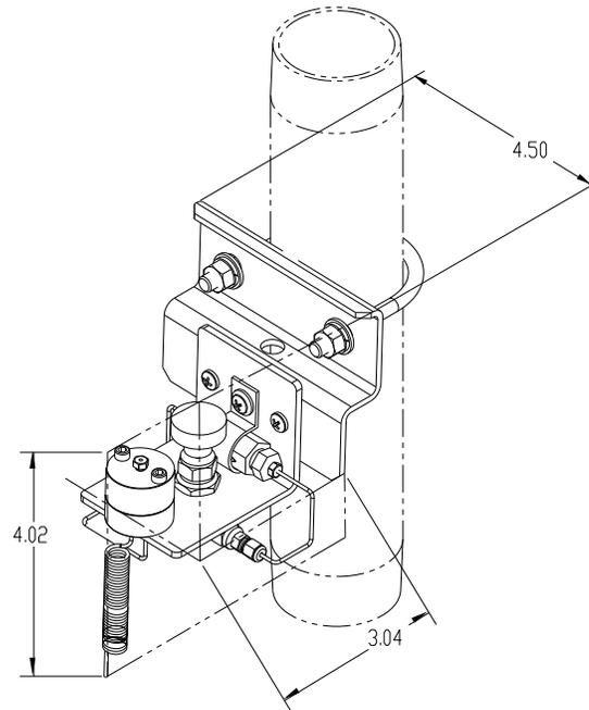
**Figure 1-26 Single Stream Conditioning Module Dimensions**
