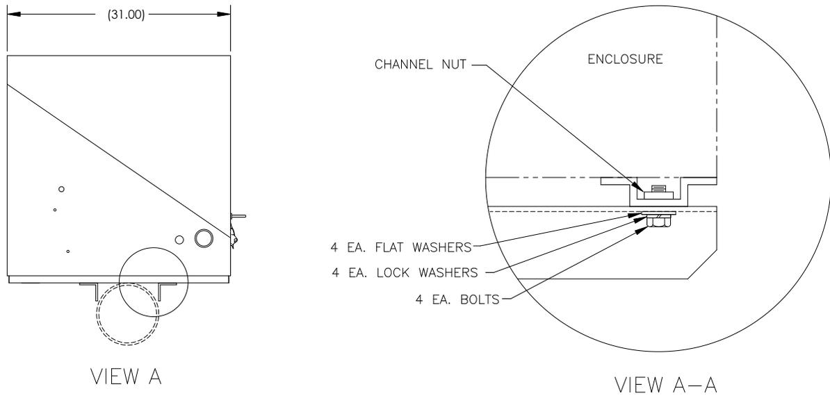
**Figure 2-10 ENC82L-Mounting Hardware Installation**
