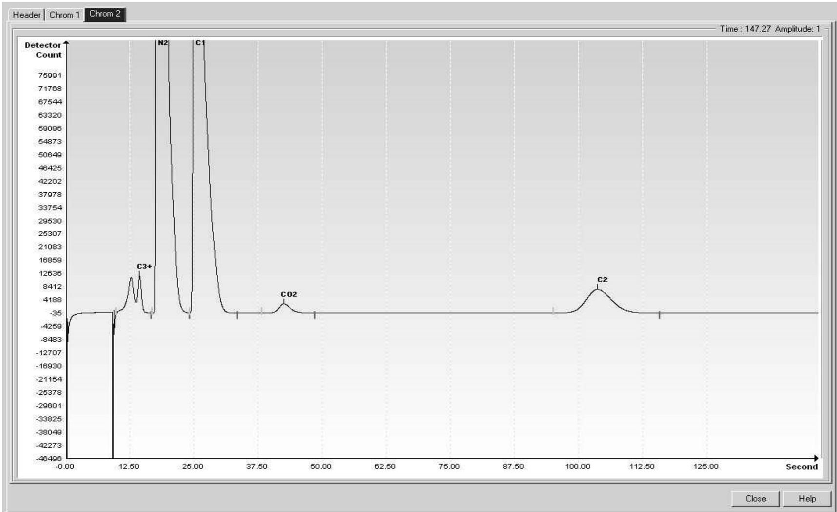
Figure 7-14 BCF Hydrogen Reference Chromatogram
