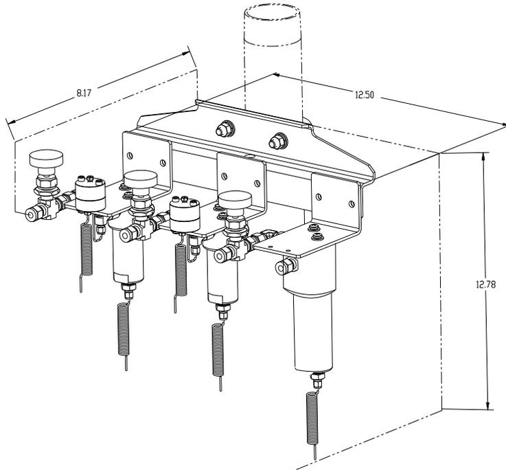
**Figure 1-27 Multiple Stream Conditioning Module Dimensions**
