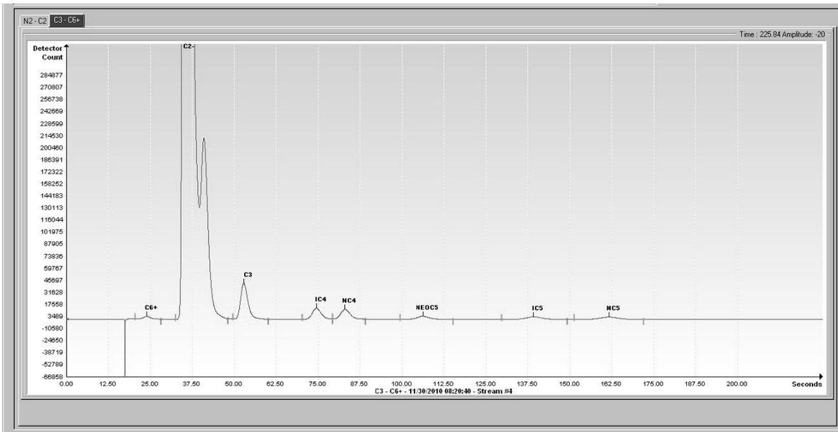
**Figure 6-15 Run Cycle Chromatogram**
