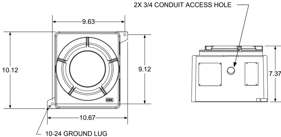
**Figure 2-66 Explosion-Proof AC Power Supply Top/Front Dimensions**
