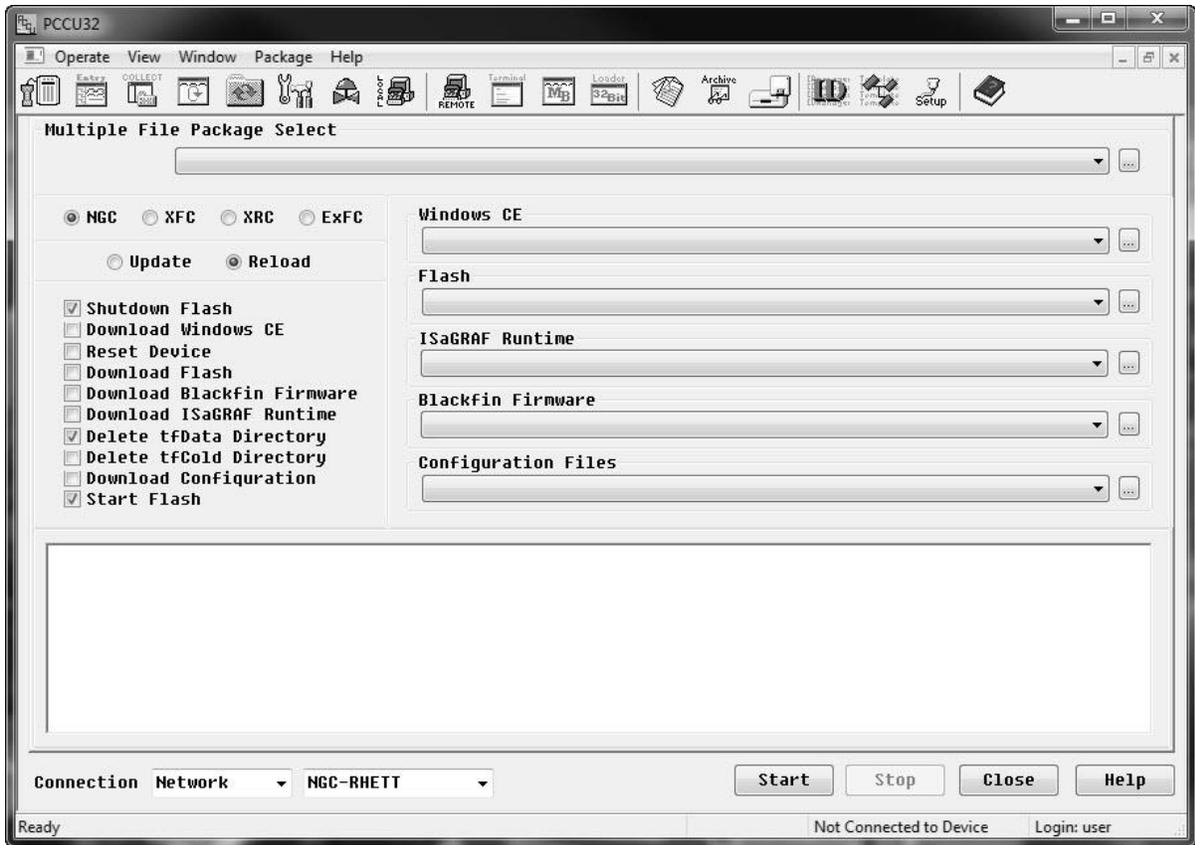
**Figure 6-2 PGC1000 Cold Boot via PCCU32 and the 32-Bit Loader**
