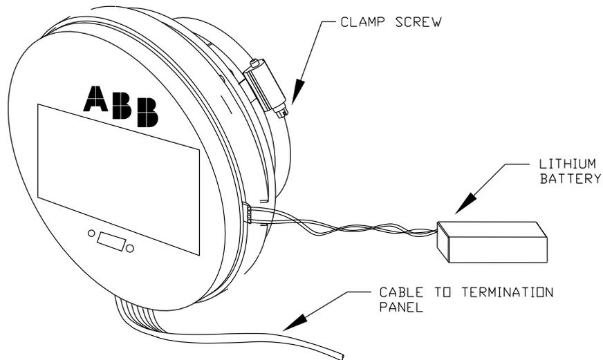
**Figure 4-4 Digital Controller Complete Assembly**
