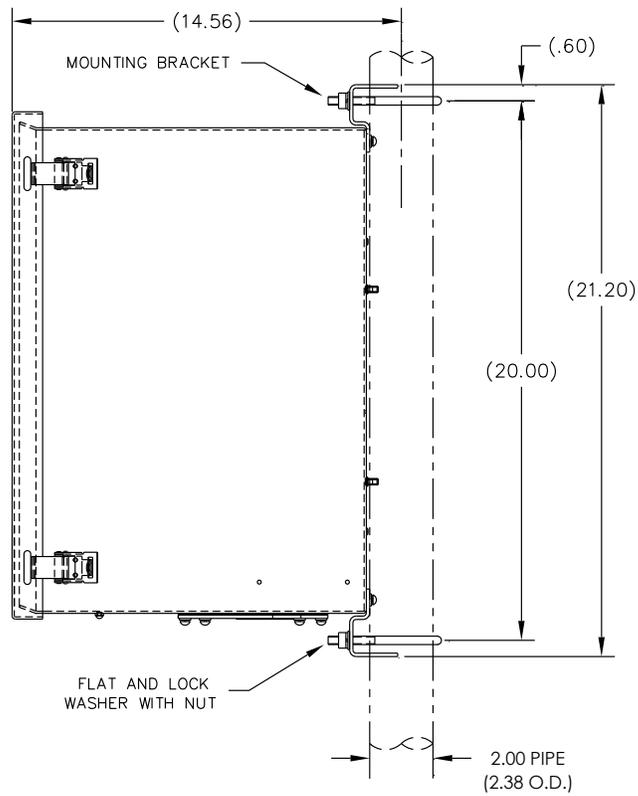
**Figure 2-60 6700 Enclosure Pipe-Mounting Installation**
