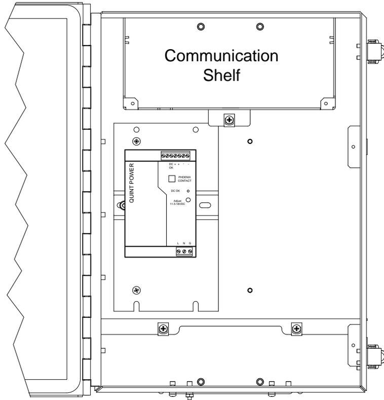
**Figure 2-70 6700 Optional Equipment Enclosure Unit with Power Supply**
