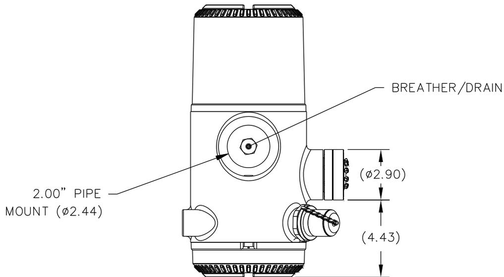
**Figure 1-7 PGC1000 Enclosure Bottom View**
