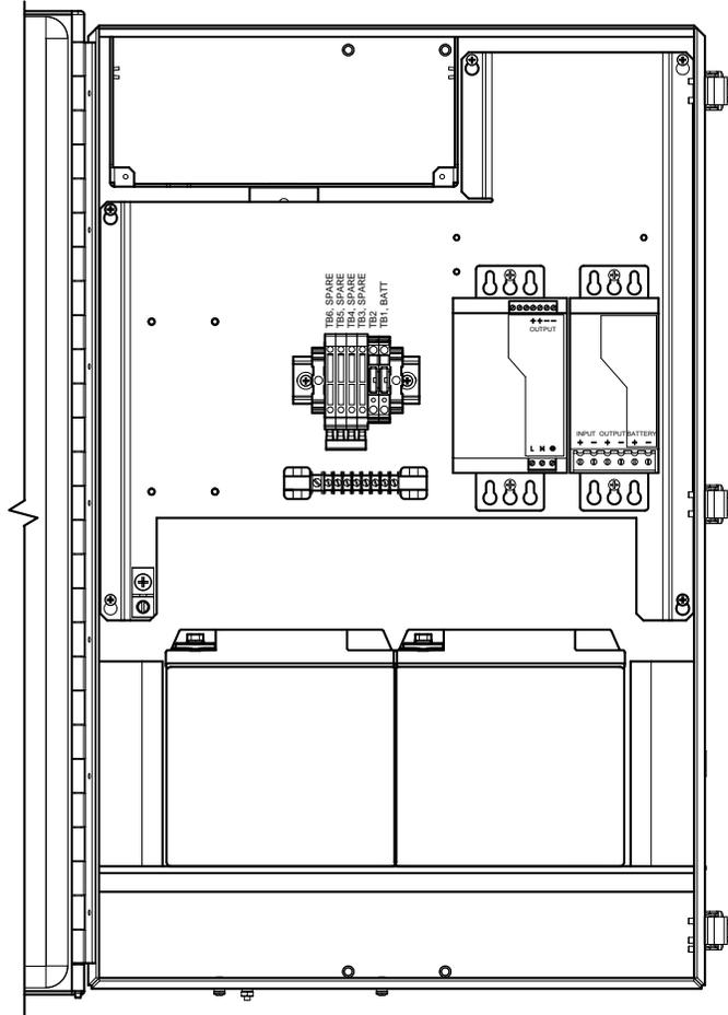
**Figure 1-31 6800 Enclosure with 115/230 Vac UPS Power Option**
