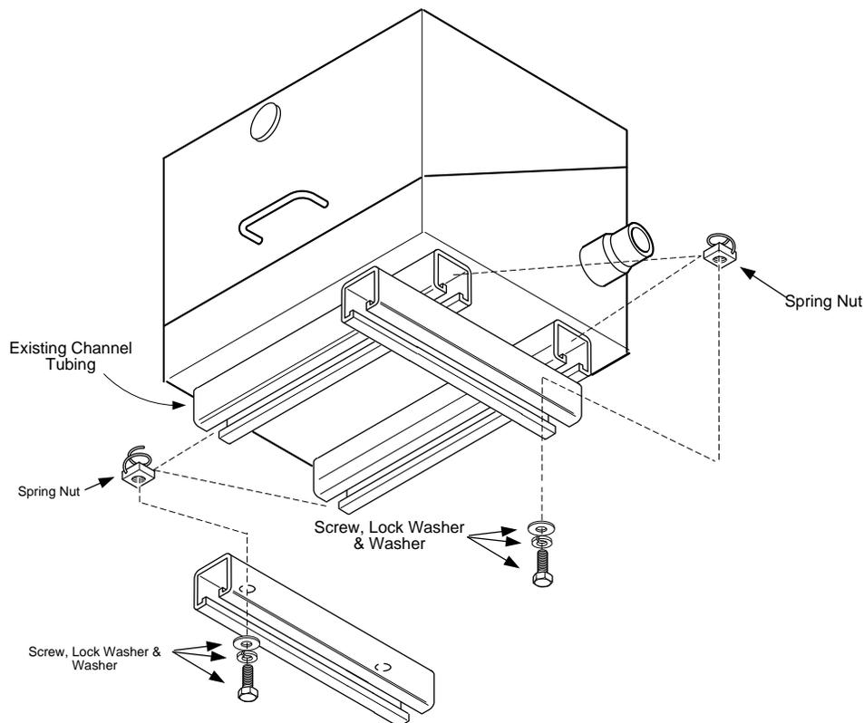
**Figure 2-15 ENC82S–Channel Tubing Installation**
