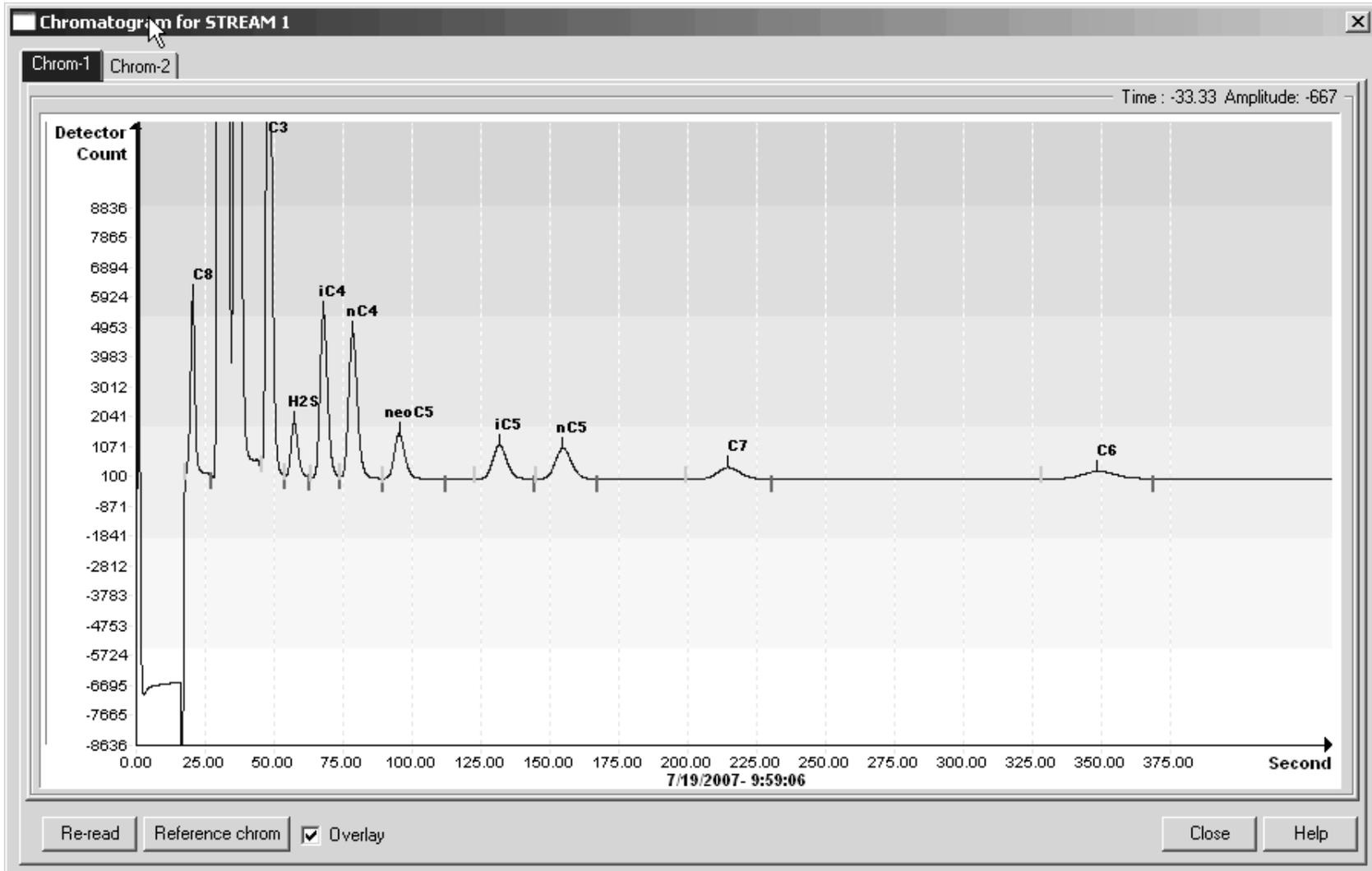
Figure 7-16 BCH Helium Reference Chromatogram
