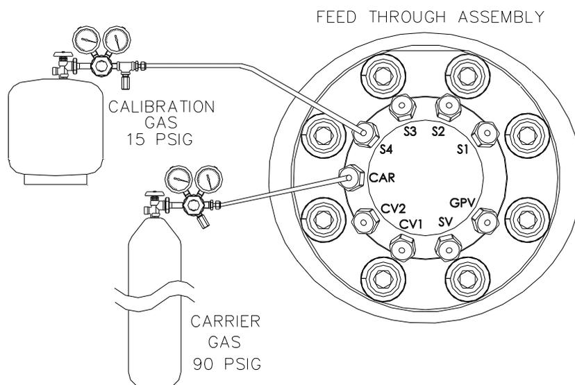
**Figure 2-45 Carrier and Calibration Gas Connections**
