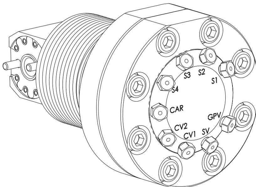
**Figure 1-8 PGC1000 Feed-Through Assembly**
