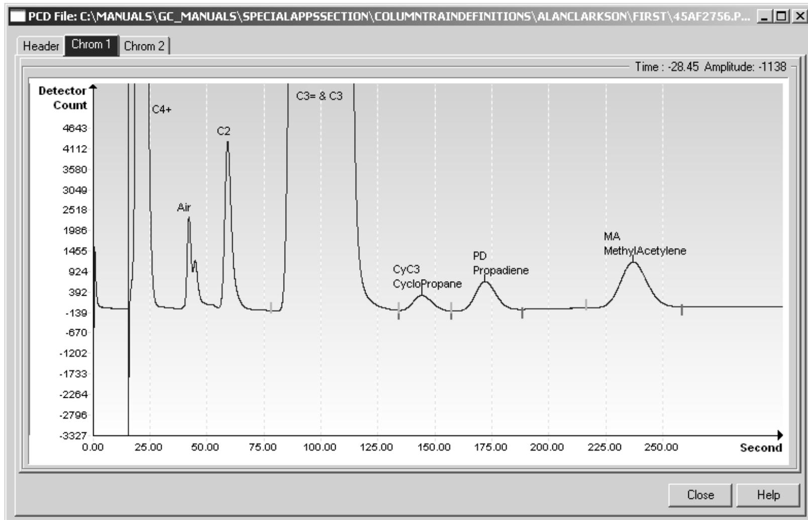
Figure 7-10 BBX Hydrogen Reference Chromatogram
