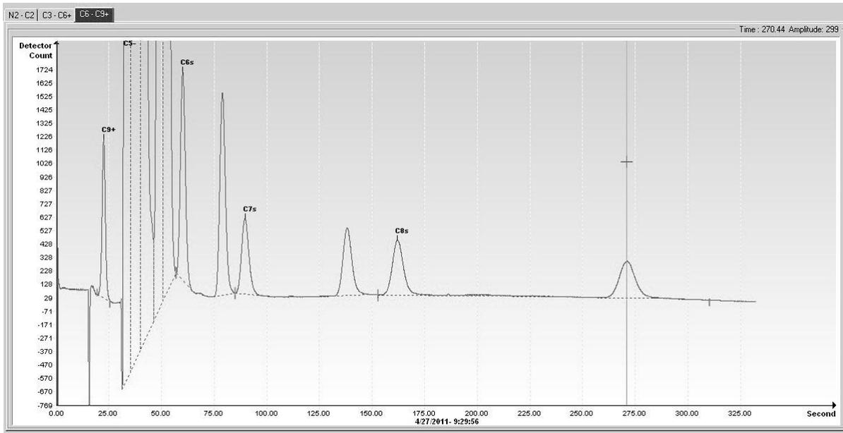
**Figure 6-19 Example of a C9+ Chromatogram**
