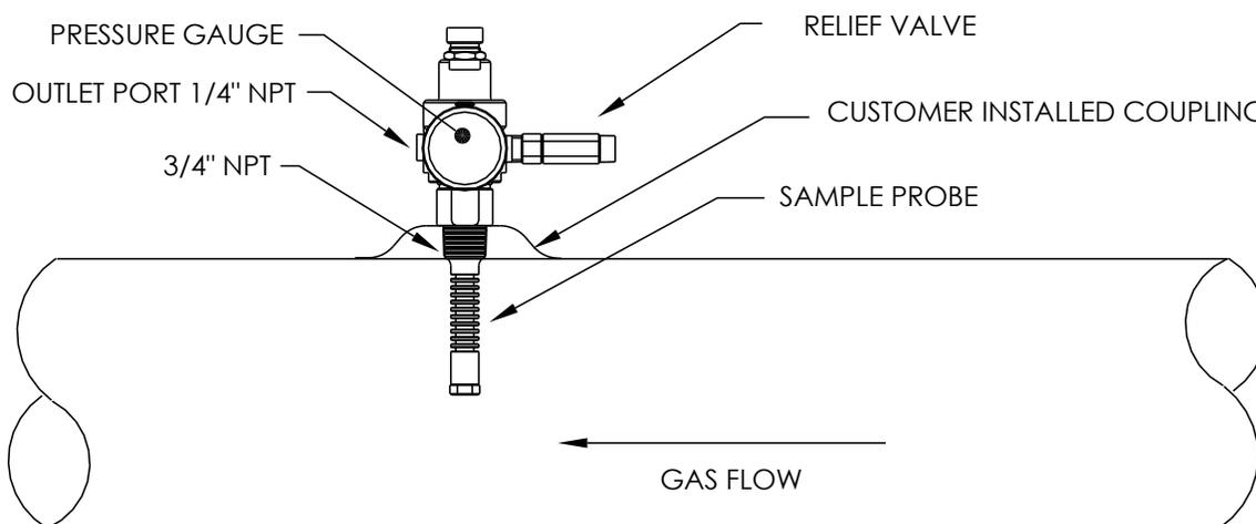
**Figure 1-19 Temperature Compensated Regulator with Sample Probe**
