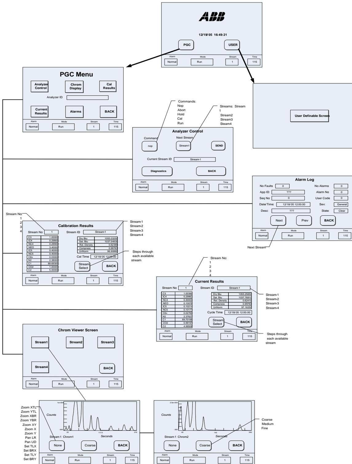
**Figure 1-14 Optional PGC1000 VGA Display Screens**
