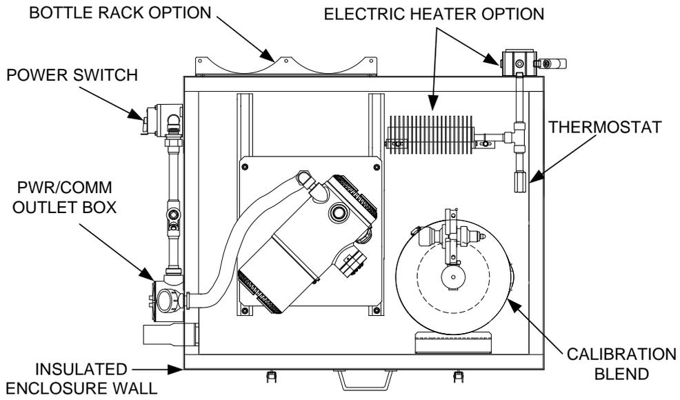
**Figure 1-20 ENC82L Environmental Enclosure with Electric Heater**
