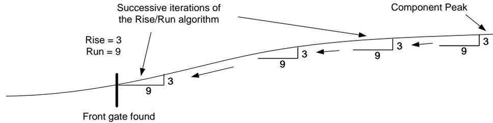
**Figure 6-7 A Successful Front Gate Determination**
