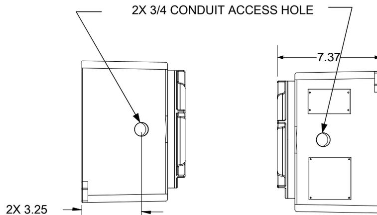
**Figure 2-67 Explosion-Proof AC Power Supply Side Dimensions**
