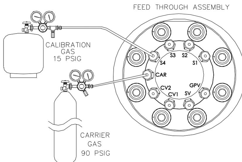
**Figure 2-45 Carrier and Calibration Gas Connections**
