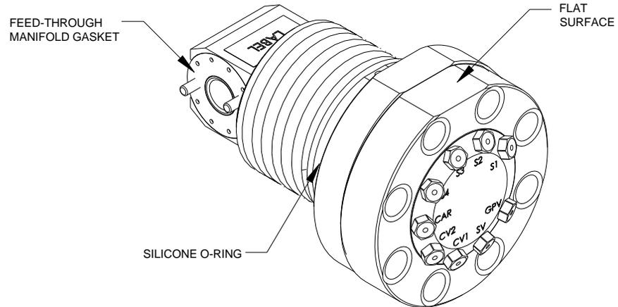
**Figure 4-10 Feed-Through Assembly**
