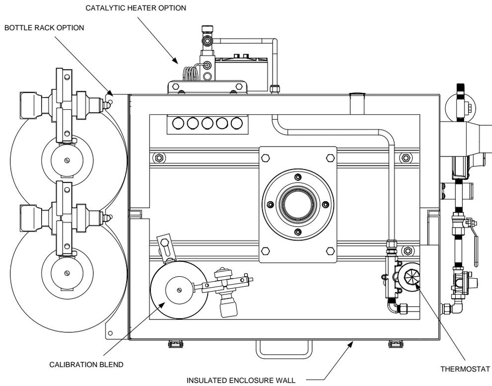
**Figure 1-23 ENC82S Environmental Enclosure with Catalytic Heater**
