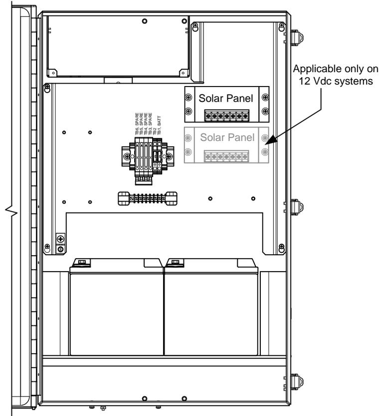
**Figure 1-30 6800 Enclosure with 12/24 Vdc Solar Panel Power Pack Option**
