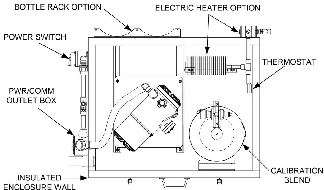
**Figure 2-55 ENC82L Electric Heater Installed in Enclosure**
