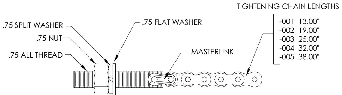
**Figure 2-11 ENC82L-Adjustment Assembly**
