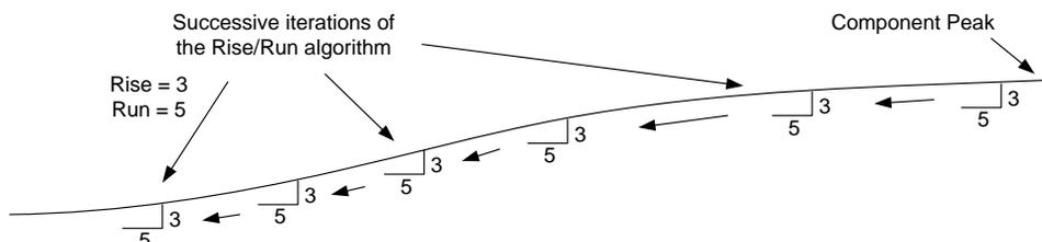
**Figure 6-6 Failure to Define a Front Gate**
