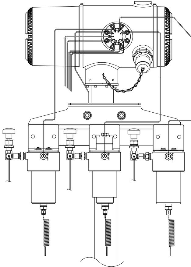
**Figure 2-25 Sample Conditioning Module Line Installation**
