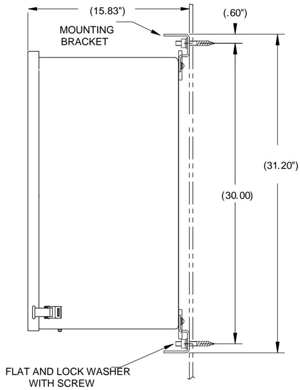
**Figure 2-64 6800 Enclosure Wall-Mounted Installation**
