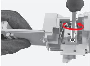
By means of the flat screwdriver push as indicated by the arrow the microswitch I/O assembly and manually remove it.
