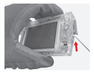
**77** By means of the flat screwdriver unhook the HMI box from the display.
