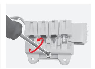
**105** Manually separate the S51 signal assembly from the motor PCS support.
