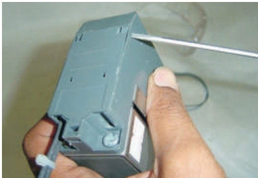
Figure 2. Removing the existing cover
