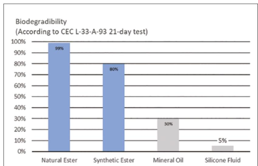
Figure 4. Biodegradability performance of fluids after 21 days
