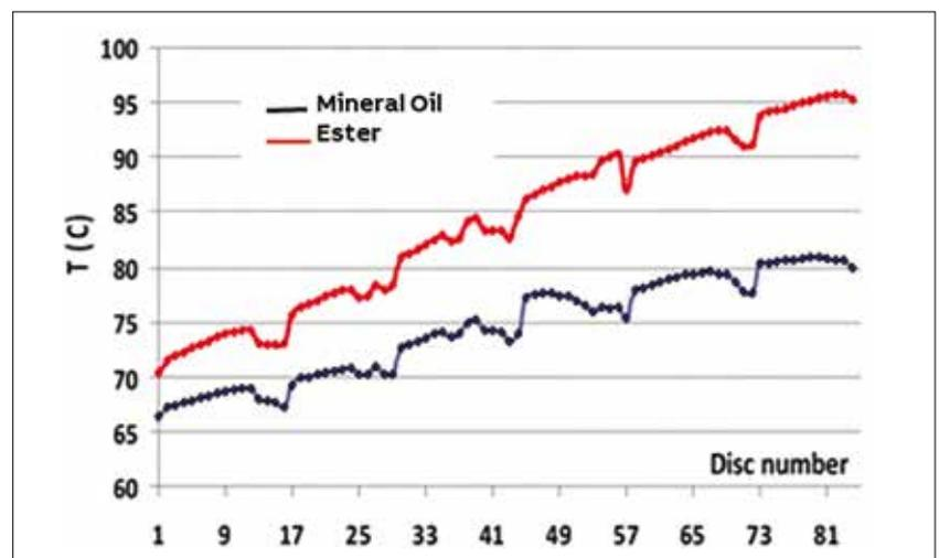
Figure 8b. Winding temperature gradients disc by disc
