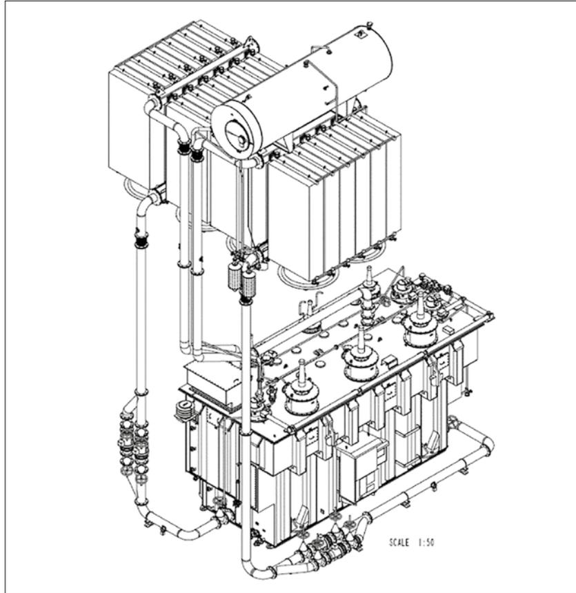
Figure 11. Transformer with cooling equipment mounted externally above ground level
