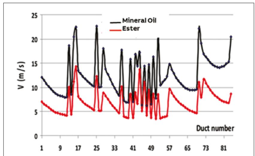
Figure 8a. Fluid velocities disc by disc
