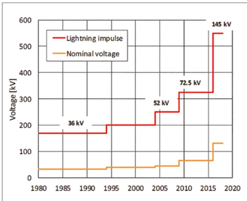
Figure 12. Evolution of the voltage level for Hitachi ABB Power Grids dry-type transformers
