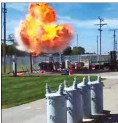
a) Mineral oil failure
