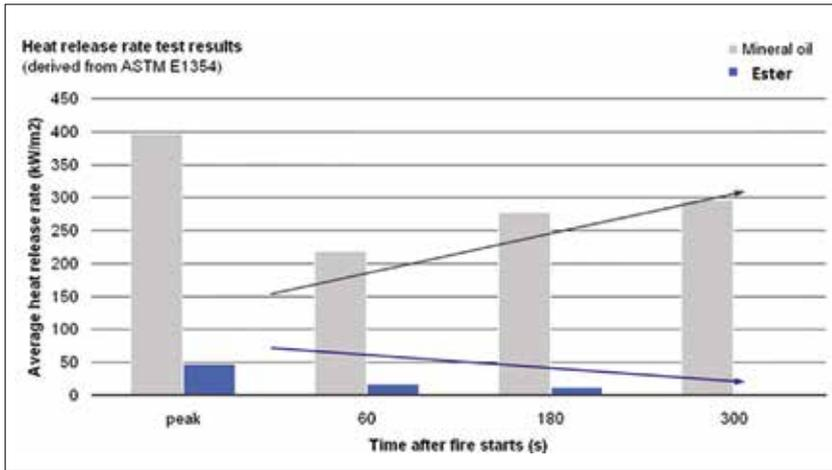
Figure 2. Heat release rates of esters and mineral oil
