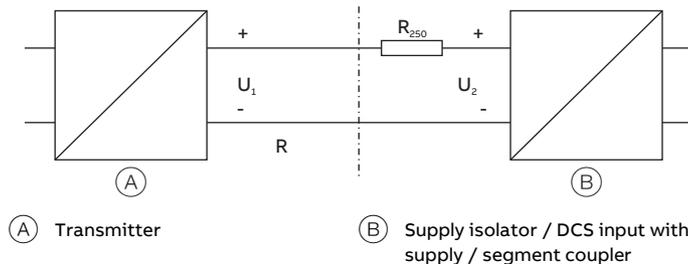
Figure 23: HART load resistance
