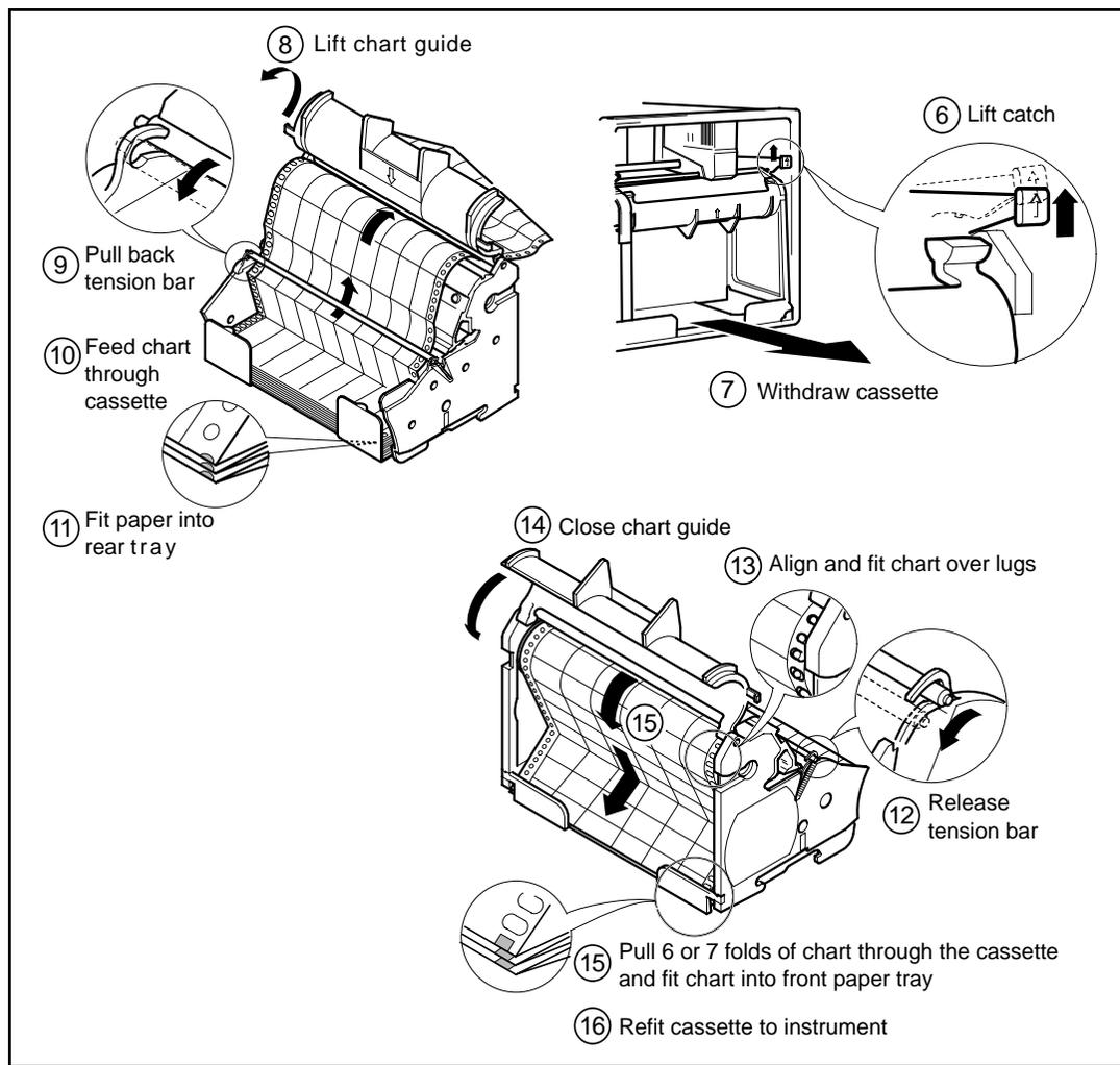
**Caution.** Once chart loading is complete, ensure the correct chart type is set in the **Chart Control Configuration Page** – see Section 3.4.1 in the User Guide.
