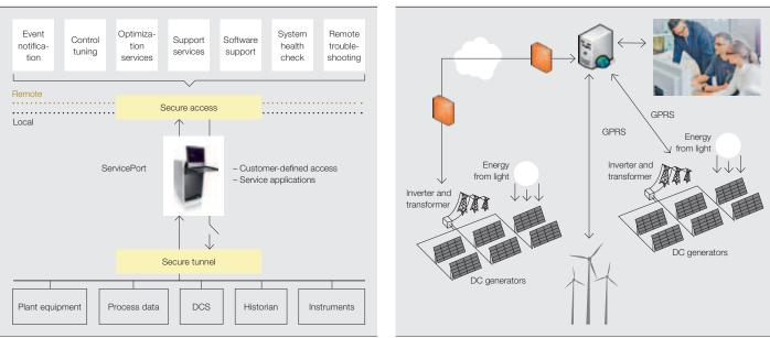
ServicePort is a remote-enabled service interface that provides process automation systems with an on-site connection to the service center. defined security features, this on-site node acts as a service coordinator. It supports system configuration, preventive and corrective maintenance management, system diagnostics, condition monitoring, corrective implementation and service scheduling  $\rightarrow$  3.
