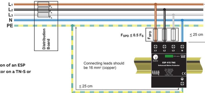
Figure 3: Parallel installation of an ESP 415/XXX Protector on a TN-S or TT supply
