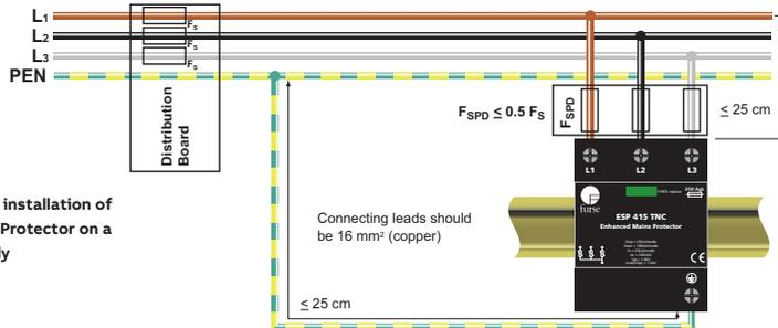
Figure 4: Parallel installation of an ESP 415/XXX Protector on a TN-C or TT supply
