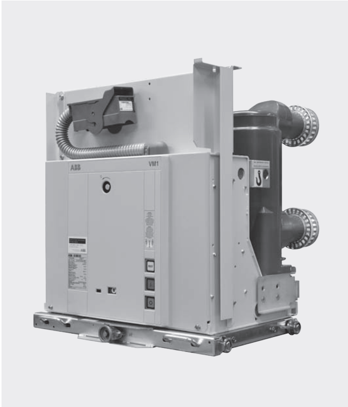
Figure 9/5: Vacuum circuit-breaker type VM1, high current, on withdrawable part, 12 kV, 3150 A, 50 kA, mechanism side.
