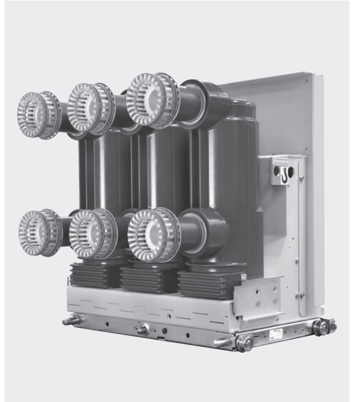
Figure 9/6: Vacuum circuit-breaker type VM1, high current, on withdrawable part, 12 kV, 3150 A, 50 kA, pole side.
