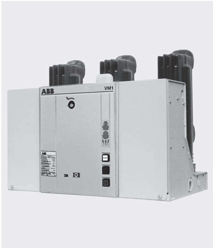
Figure 9/1: Vacuum circuit-breaker, type VM1, high-current, for fixed installation, 12 kV, 1600...2000 A, 40 kA, mechanism side.
