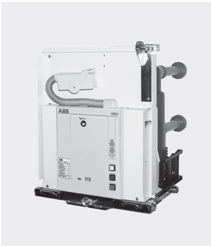
Figure 9/3: Vacuum circuit-breaker, type VM1, on withdrawable part, 24 kV, 1250 A, \leq 25 kA, mechanism side (use in ZS8.4 only).
