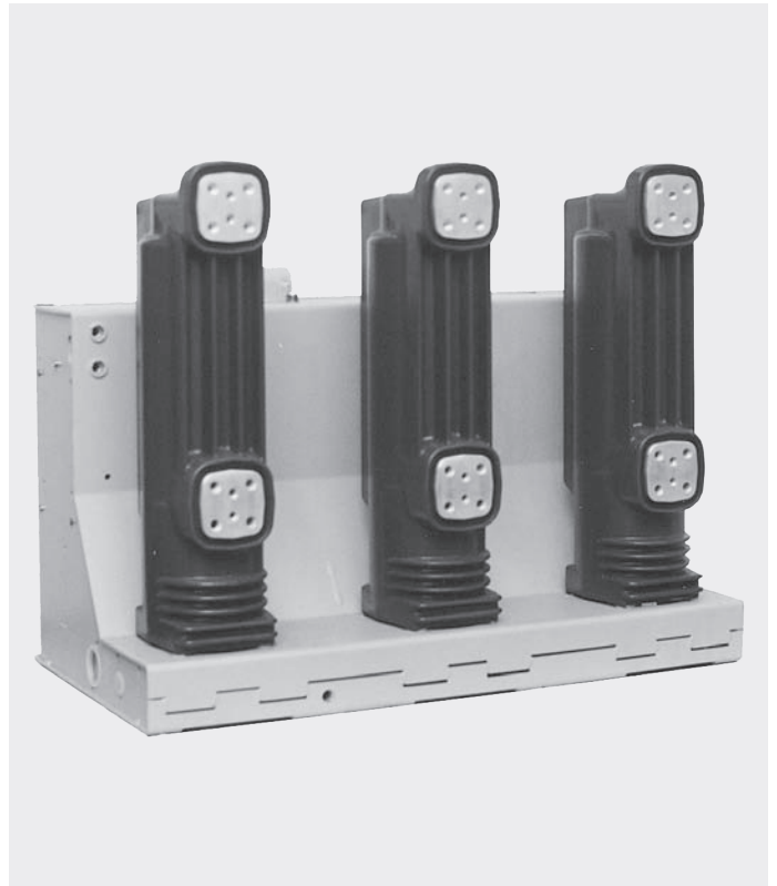
Figure 9/2: Vacuum circuit-breaker, type VM1, high-current, for fixed installation, 12 kV, 1600...2000 A, 40 kA, pole side.
