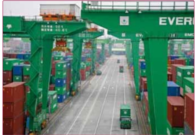
Figure 2. Side-loading with Internal Transfer Vehicles (ITVs), Kaohsiung, Taiwan.
