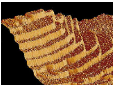
AFM (Atomic Force Microscope) picture showing terraces of material in steps of 1/2 and 1 unit cell
