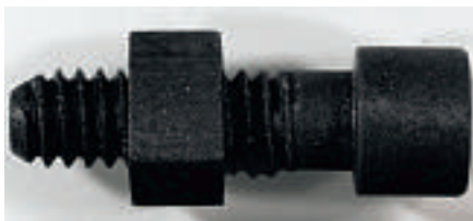
Machined nut and bolt made from MAX ceramics
