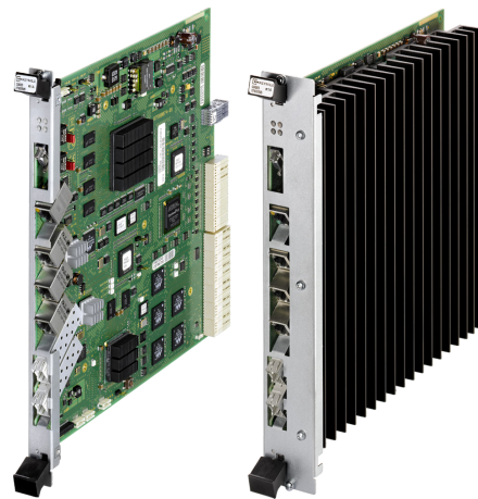
01 Core unit COGE5 (left) and variant for fanless operation COGE5-F
