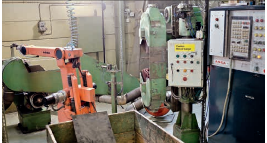
1 First IRB 6 customer – overview of cell
