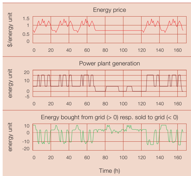
3 Time evolution of: price of electricity (upper plot), generated power (middle plot), and power exchange with the grid (lower plot).
