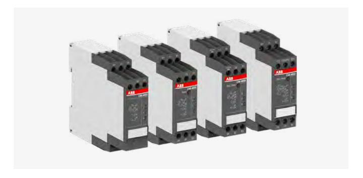
The thermistor motor protection relays of the CM-MSx range protect motors with PTC sensors against high temperature. These sensors are incorporated in the motor windings, thus measuring the motor heat directly.
