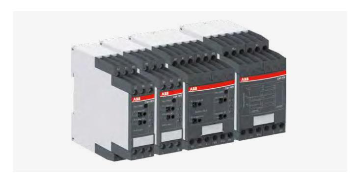
The insulation monitoring relays of the CM-IWx range guarantee a continuous insulation monitoring of an IT system. The devices recognize insulation faults as they develop and warn immediately if the value has fallen below the minimum set threshold. This ensures a reliable operation of the system and prevents operational interruption caused by a second, more severe, insulation fault which may lead to a short circuit tripping the main circuit breaker.
