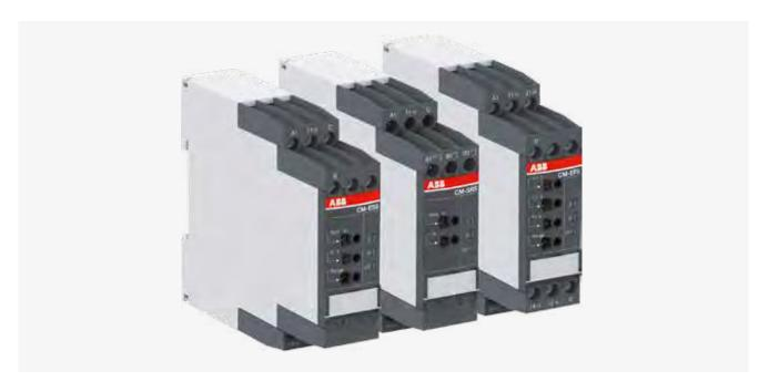
For the monitoring of currents and voltages in single-phase AC/DC systems, ABB's CM-range contains a wide selection of powerful and compact devices, all in an only 22.5 mm wide housing. This product range includes current and voltage monitoring relays for over- and undercurrent and voltage protection – from 3 mA to 15 A, and from 3 V to 600 V.
