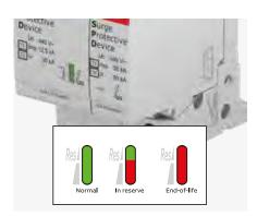
A safety reserve system for an extended protection. T1-T2s and T2s. These Surge Protective Devices are equipped with two varistors per pole. If one varistor is damaged, the SPD gives advanced warning that it is approaching the end of its life while the other varistor continues to protect the equipment, allowing to perform Preventive Maintenance.
