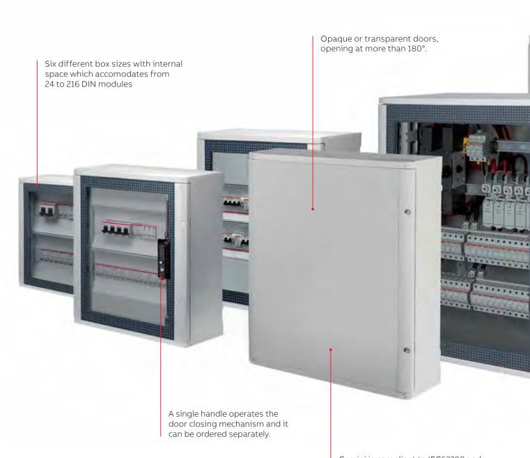
Gemini is compliant to IEC62208 and UL 508A standards. IP66 certifies Gemini is completely protected against the infiltration of solid bodies and is resistant to the penetration of jets of water similar to sea waves.
