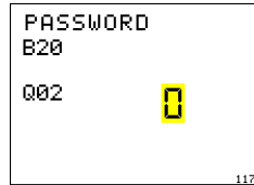
Fig.13-4 Setting the password z-19117
