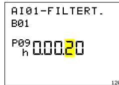
Fig.13-7 Filter time constant 0.00.20 h = 20 s z-19120
