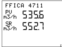
Fig.7-7 Process value PV = flow A and SP = setpoint flow A
