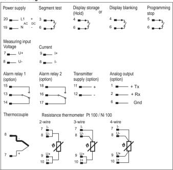
Relay contact positions are shown for de-energized state.
