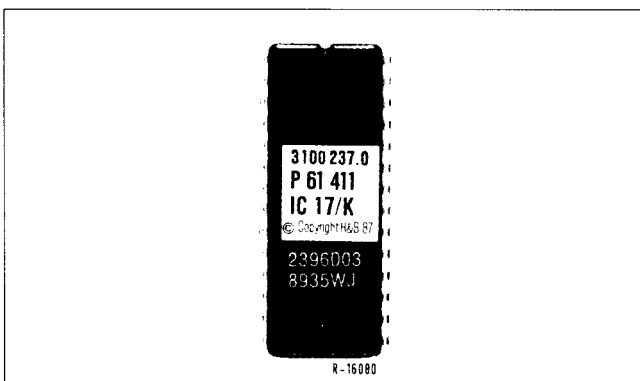
Fig. 2 EPROM with firmware
