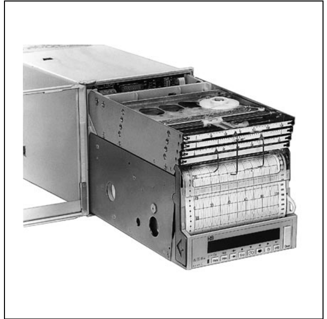
Fig. 5 Pulling forward the slide-in unit R-17073
