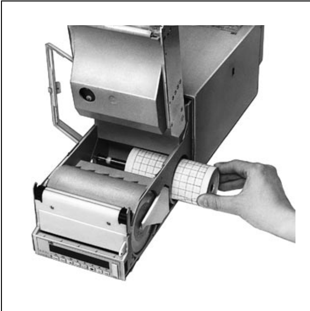
Fig. 8 Inserting the roll chart from the side R-17076
