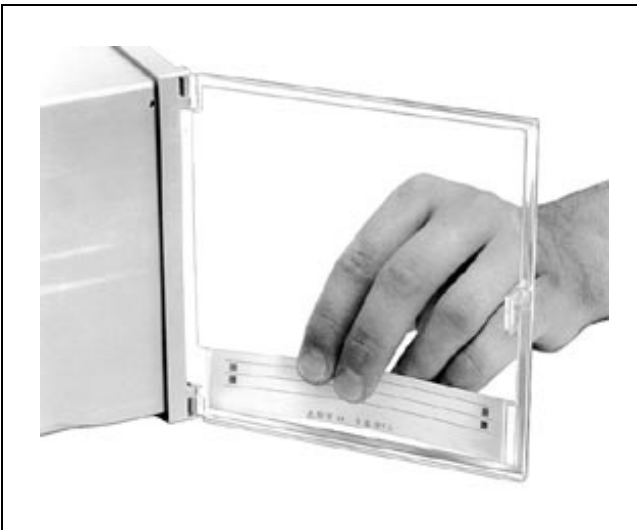
Fig. 18 Replacing the measuring point name plate Z-17676
