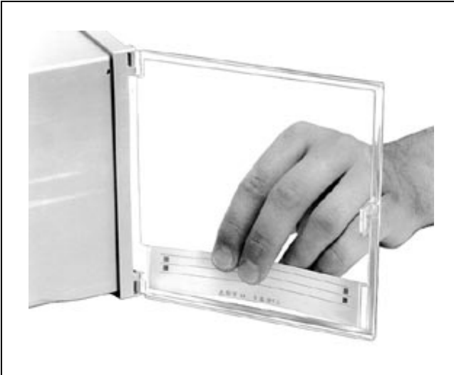
Fig. 19 Replacing the measuring point name plate Z-17676
