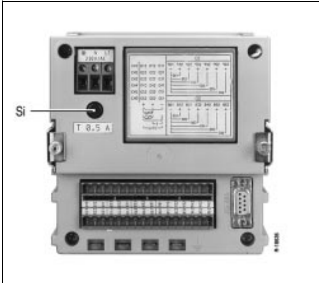
Fig. 21 Replacing fuse Si
