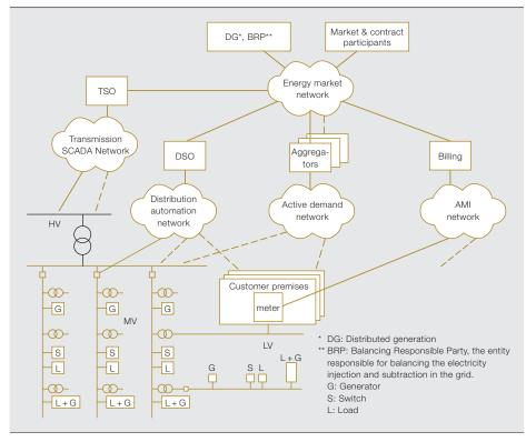
A single regional area network may support all Smart Grid functions of Distribution Automation, Active Demand control, and Automatic Meter Reading.
