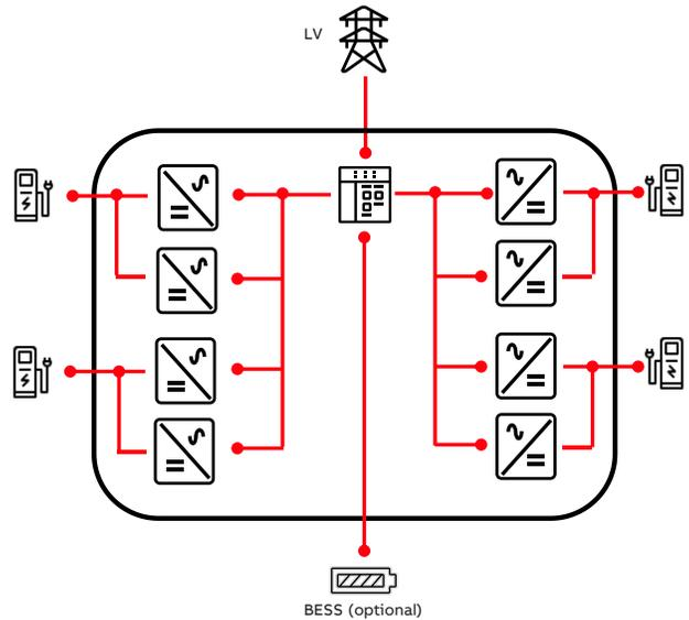
E-mobility EcoFlex HPC enclosure with integrated high-power chargers and LV distribution panel. (Charger posts installed externally.)
