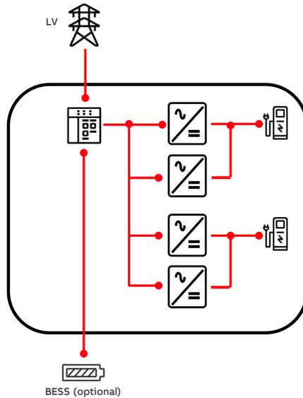
E-mobility EcoFlex HPC enclosure with integrated high-power chargers, charge posts and LV distribution panel.
