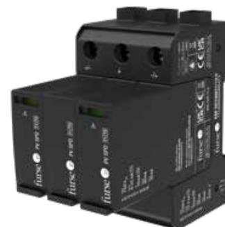
Combined Type 1 and 2 tested protector (BS EN 61643-31 and BS EN 50539-11) for a Photovoltaic PV solar panel system that is on a building where a structural Lightning Protection System (LPS) is employed, for equipotential bonding. For use at boundaries up to LPZ 0 to protect against flashover (on the DC side of the DC-AC inverter) through to LPZ 2 to protect the PV system from damage.
