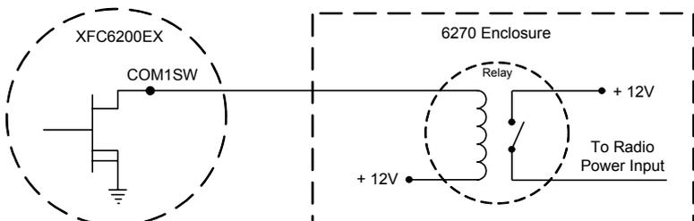
**Figure 11 (Using Interposing Relay)**
