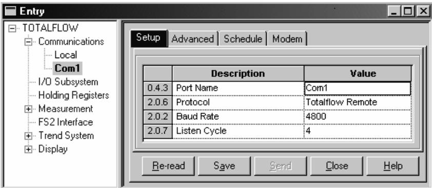
Figure 12 (Communications Setup)
