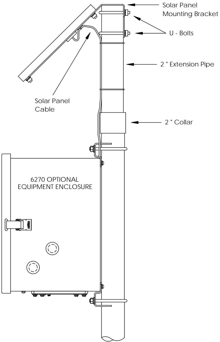
**Figure 7 (Solar Panel Mounting)**
