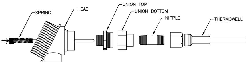
**Figure 5 (RTD Probe Assembly)**
