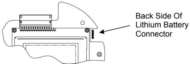
**Figure 8 (Lithium Battery Solder Pads)**
