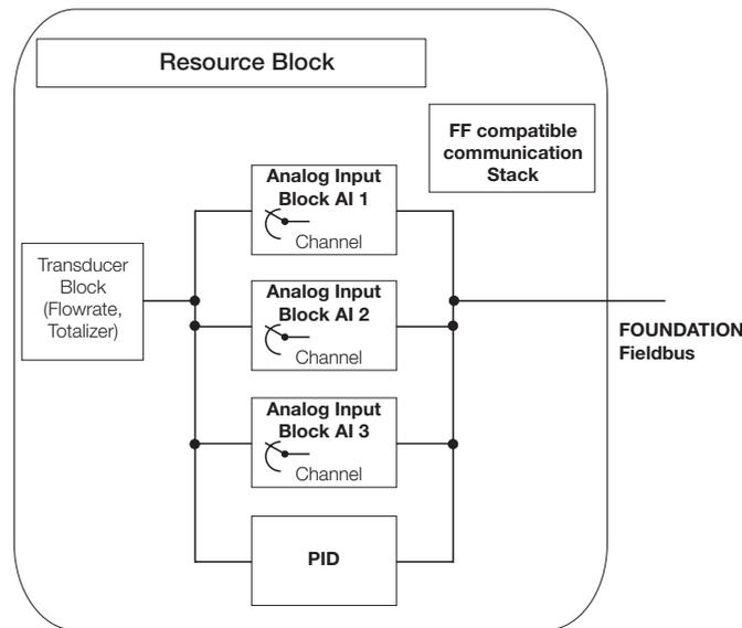
The Resource-Block, the AI-Blocks and the PID-Block are "Standard"-FF-Blocks. The correspond exactly to FF-Specification FF-891-1.4
