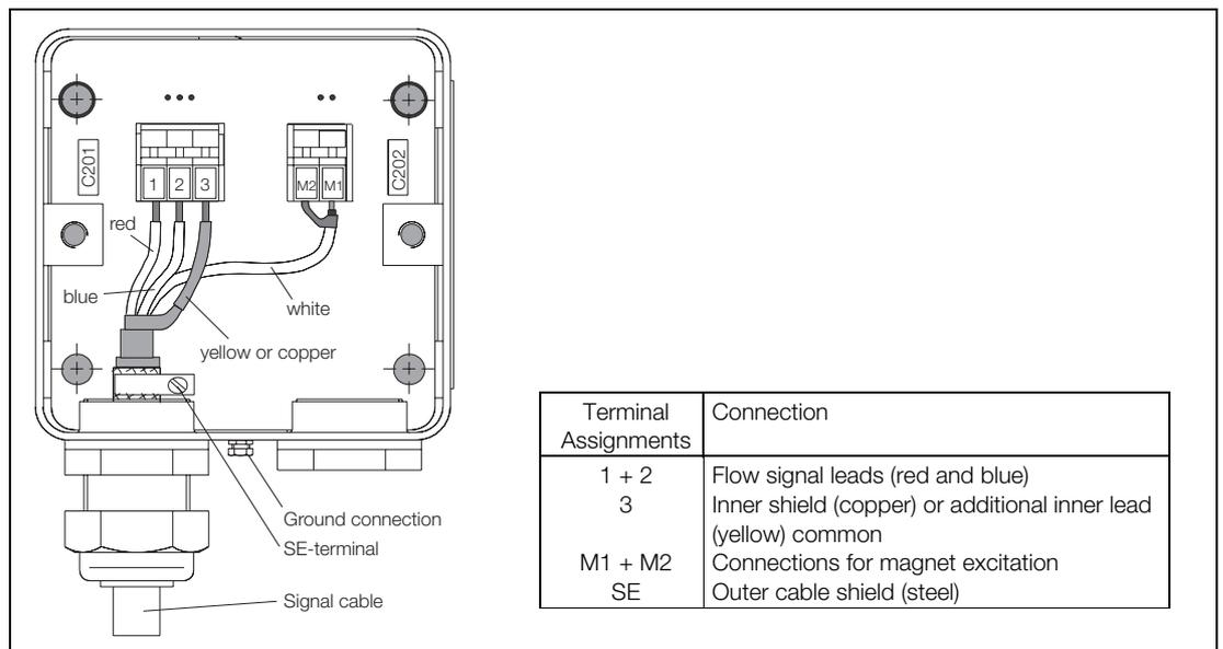
Fig. 29: Flowmeter Primary Connection Area
