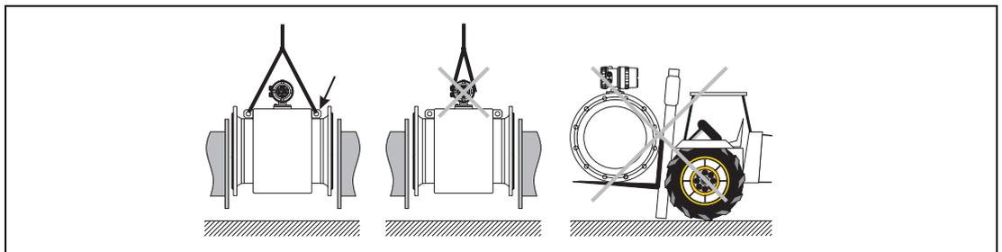
Fig. 3: Transport of Flanged Instruments  $\geq$  DN 350 [14"] [14"]
