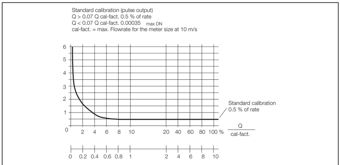
Fig. 78: Metering System Accuracy FXE4000 (COPA-XE / MAG-XE)
