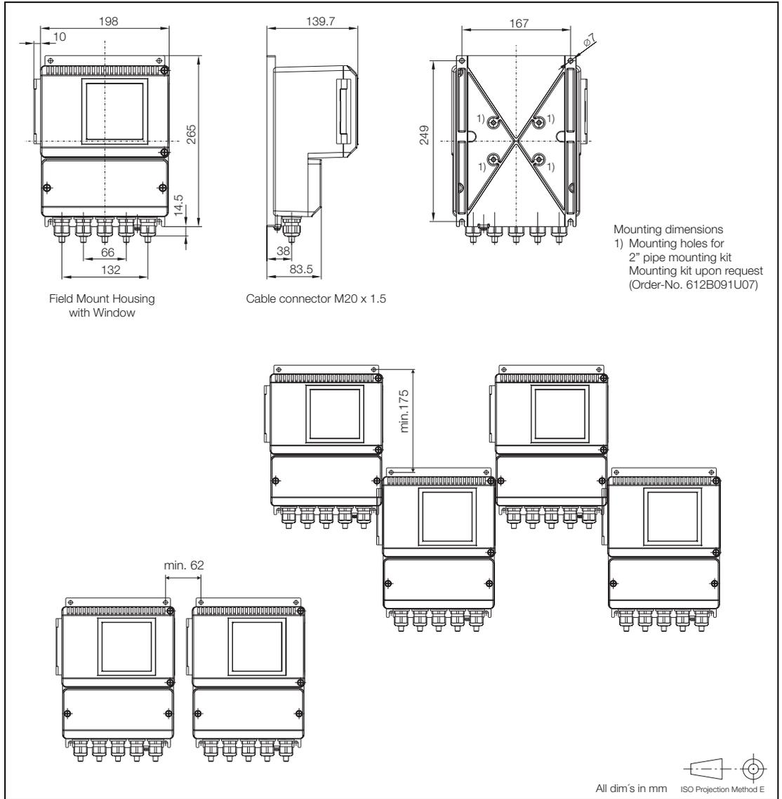
Fig. 74: Dimensions Converter Field Mount Housing, Mounting Options
