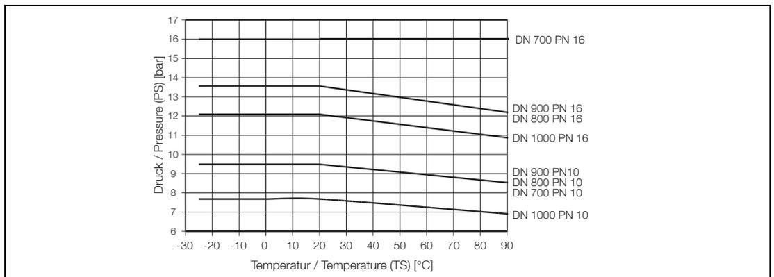
Fig. 50: DIN-Flanges SS No. 1.4571[316Ti] DN 700 - DN 1000
