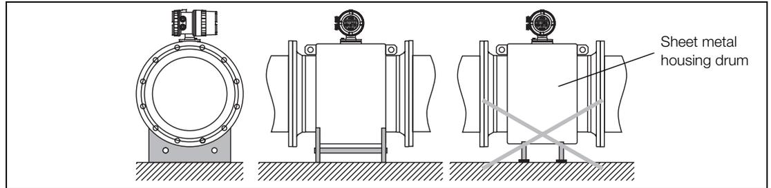
Fig. 4: Supports for Flowmeter Sizes  $\geq$  DN 350 [14"]
