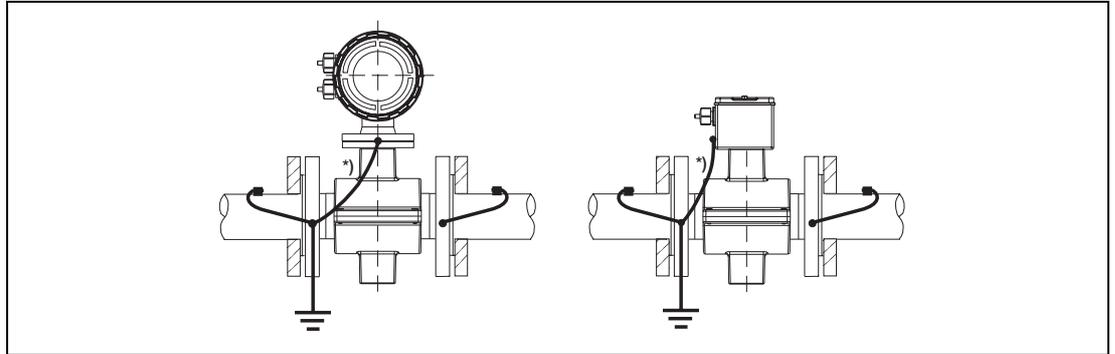
Fig. 19: Flowmeter Primary DN 3 - DN 100 [1/10" - 4"] Flanged
