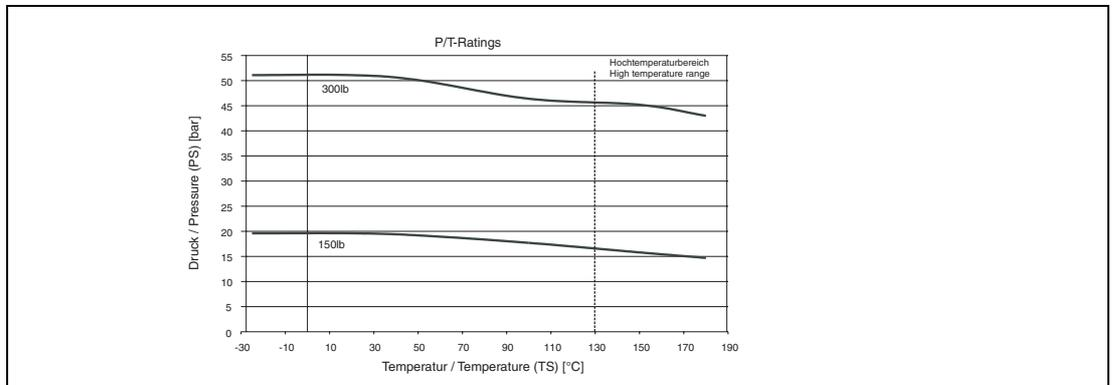
Fig. 49: ANSI-Flanges Steel to 12" (CL150/300) to 40" (CL150)
