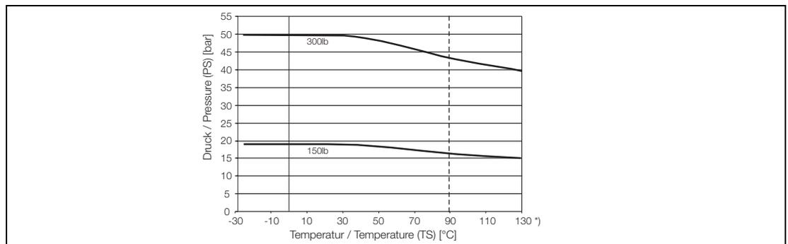
Fig. 55: ASME-Flanges SS No. 1.4571[316Ti] to 4"
