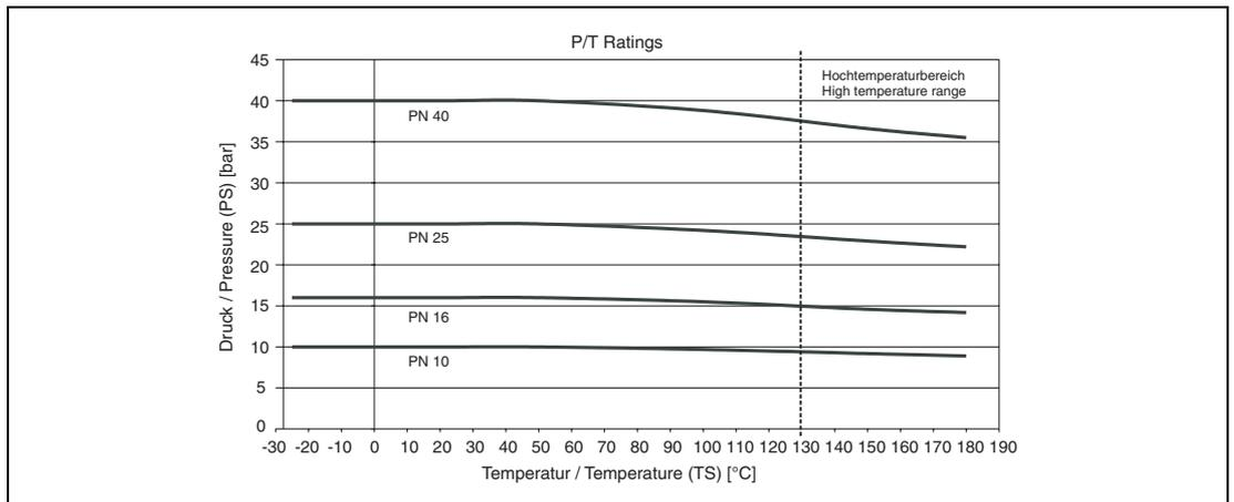
Fig. 46: DIN-Flanges SS No. 1.4571[316Ti] to DN 600
