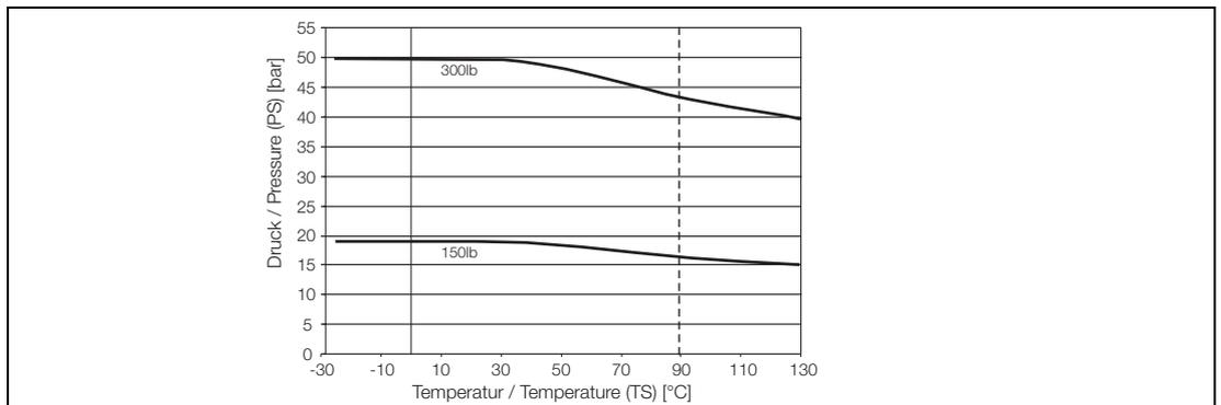
Fig. 47: ANSI-Flanges SS No. 1.4571[316Ti] to 12" (CL150/300) to 40"(CL150)
