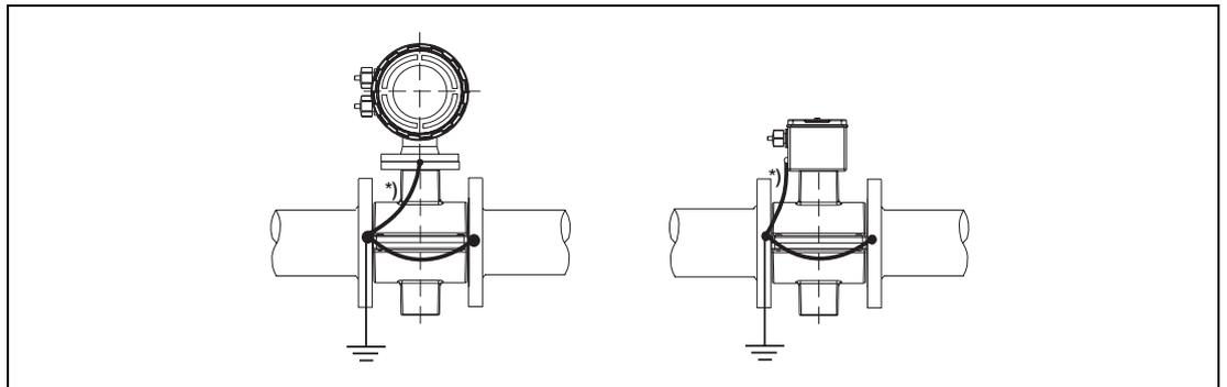
Fig. 18: Flowmeter Primary DN 3 - DN 100 [1/10" - 4"] Wafer Design
