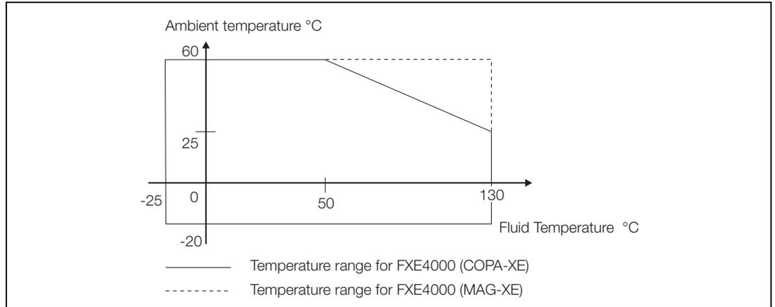
Fig. 57: Maximum Allowable Ambient temperature as a Function of the Fluid Temperature for Stainless Steel Process Connections and Wafer Designs
