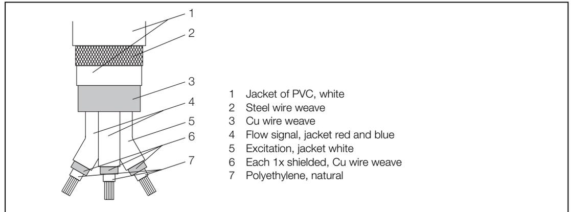
Fig. 26: Signal Cable Construction ABB No. D173D018U02
