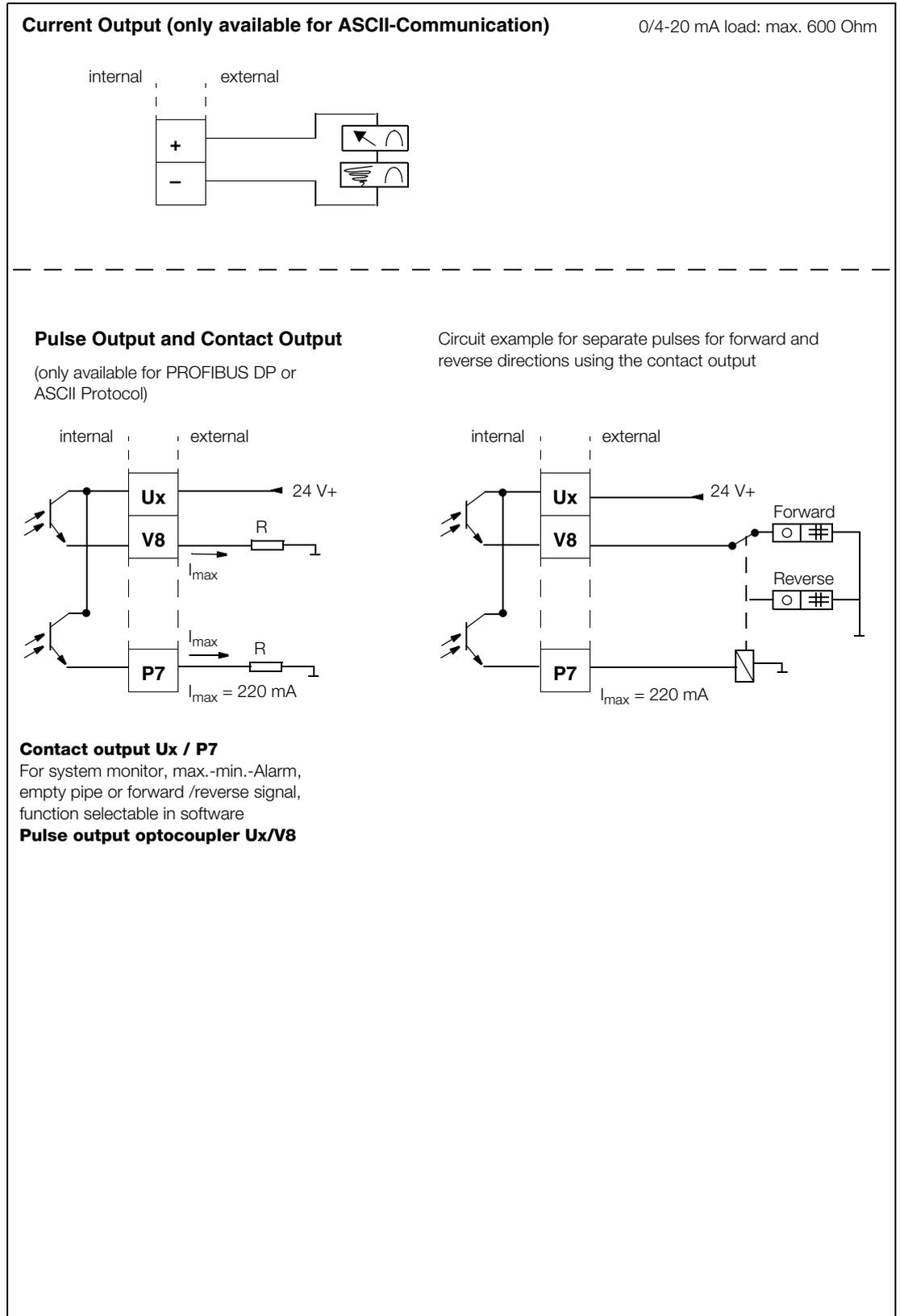
Fig. 42: Connection Examples for Peripherals for Digital Communication (PROFIBUS DP, PROFIBUS PA, FOUNDATION Fieldbus, ASCII)-Protocol
