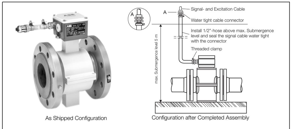
Fig. 32: Installation IP68 (Hose Connection)
