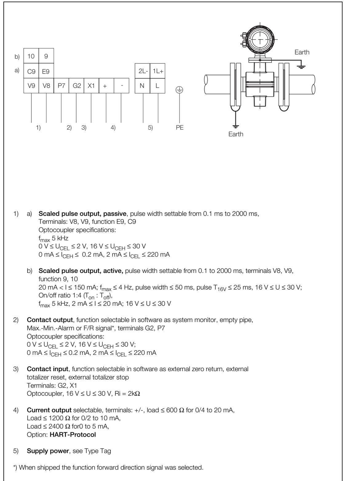
Fig. 37: Interconnection Diagram FXE4000 (COPA-XE), Connection Options for Analog Communication (incl. HART)
