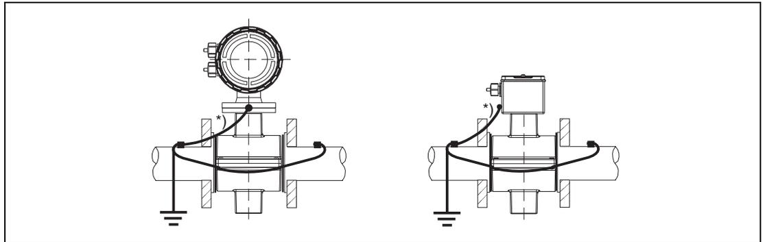
Fig. 20: Flowmeter Primary DN 3 - DN 100 [1/10" - 4"] Wafer Design
