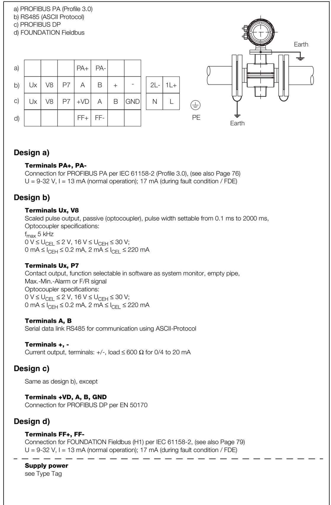
Fig. 38: Interconnection Diagram FXE4000 (COPA-XE), Connection Options for Digital Communication
