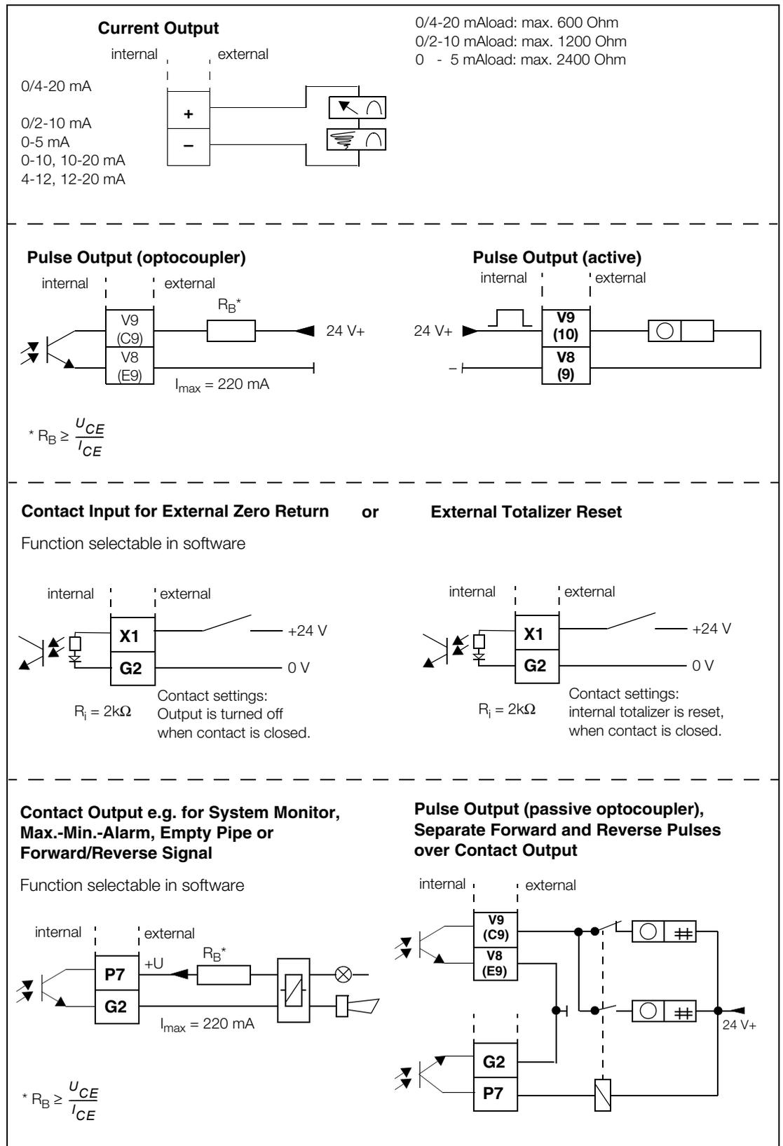
Fig. 41: Connection Examples for Peripherals for Analog Communication (incl. HART)
