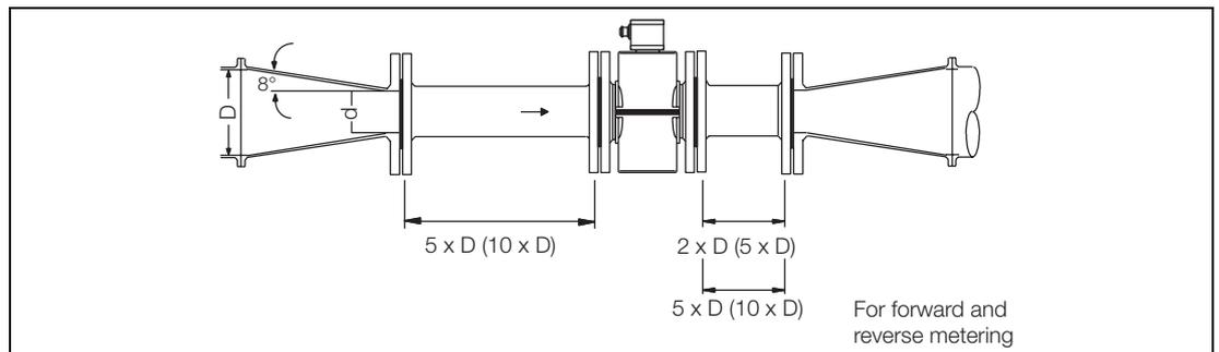
Fig. 16: Pipeline Installation, Reductions as Required
