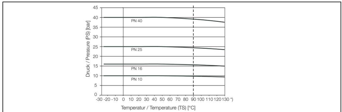
Fig. 54: DIN-Flanges SS No. 1.4571[316Ti] to DN 100
