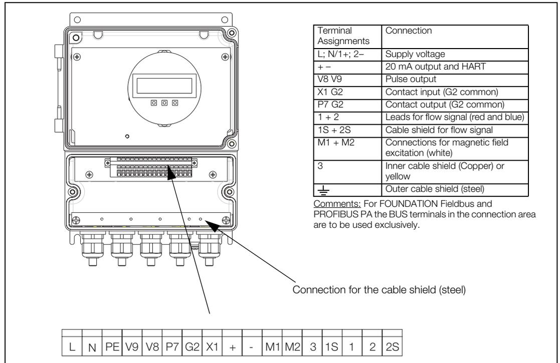
Fig. 33: Connection Box Field Mount Housing
