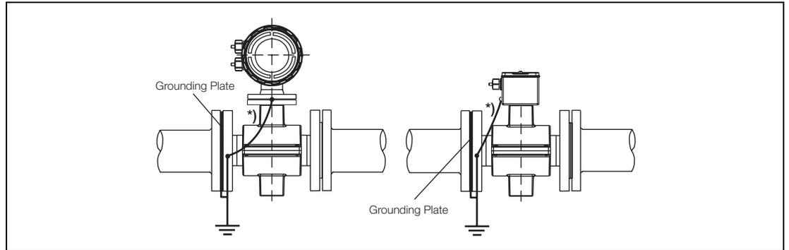
Fig. 21: Flowmeter Primary DN 3 - DN 100 [1/10" - 4"] Flanged
