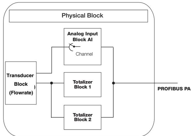
The measurement values are calculated in the Transducer-Block. The Transducer-Block provides the measured values internally. The cyclical output of the measured values externally occurs over the Analog Input Block (AI-Block). The FXE4000 has one AI-Block.
