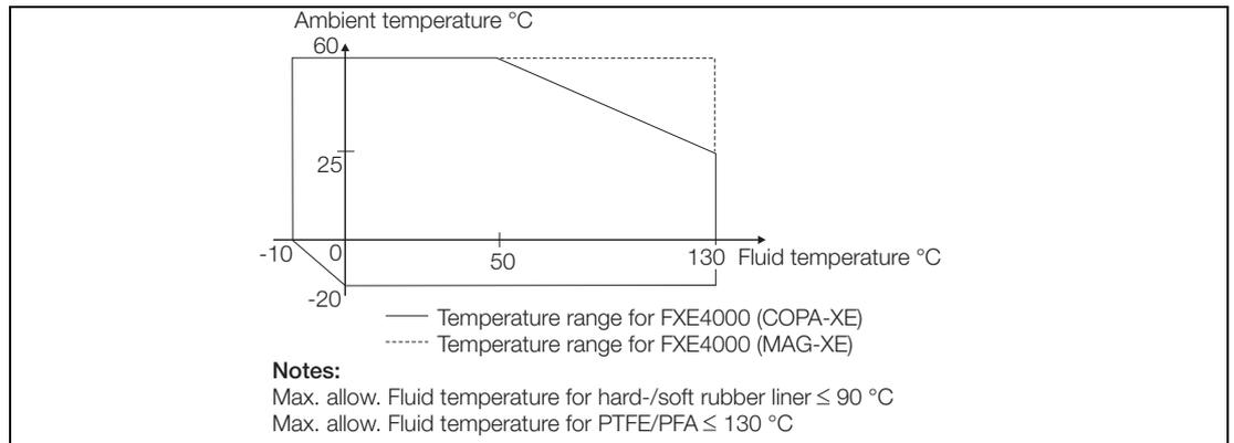
Fig. 52: Max.allow. Fluid Temperature as a Function of the Ambient Temperature for Instruments with Steel Flanges
