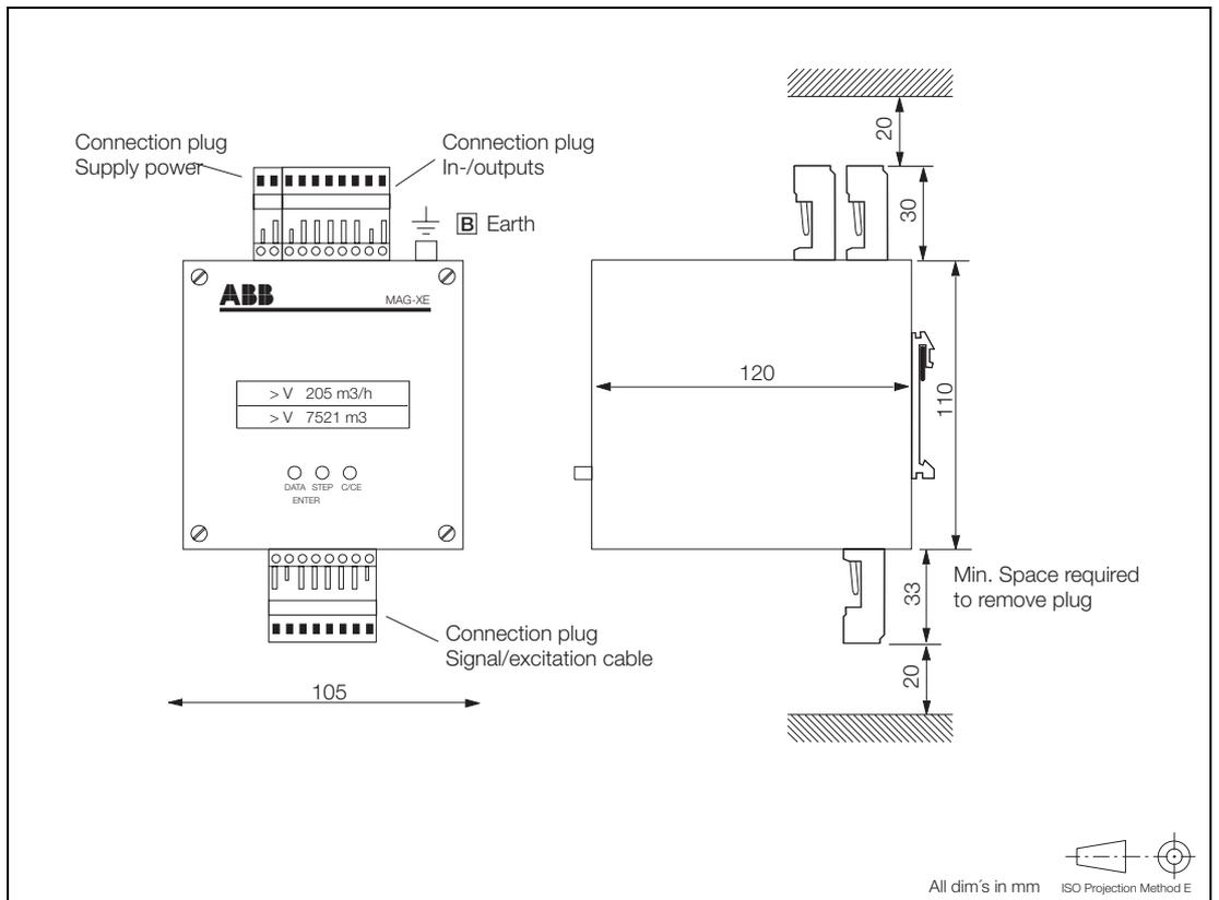
Fig. 77: Dimensions Converter FXE4000 (MAG-XE), Rail Mount Housing
