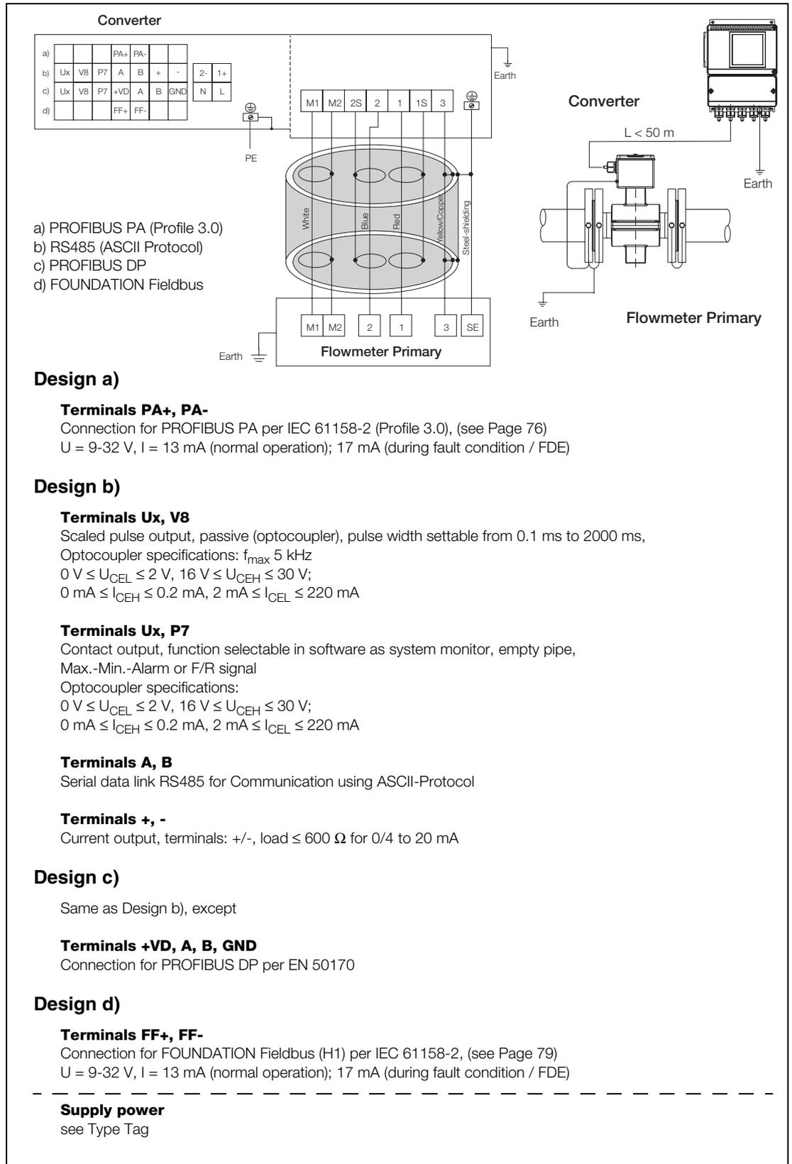
Fig. 40: Interconnection Diagram FXE4000 (MAG-XE), Connection Options for Digital Communication (PROFIBUS DP, PROFIBUS PA, FOUNDATION Fieldbus, ASCII)
