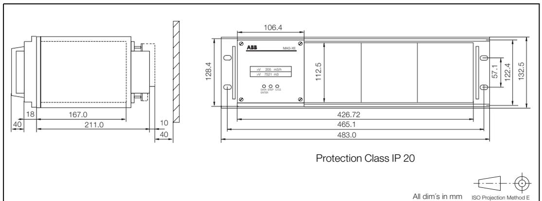
Fig. 75: Dimensions 19" Converter FXE4000 (MAG-XE), Card Frame
