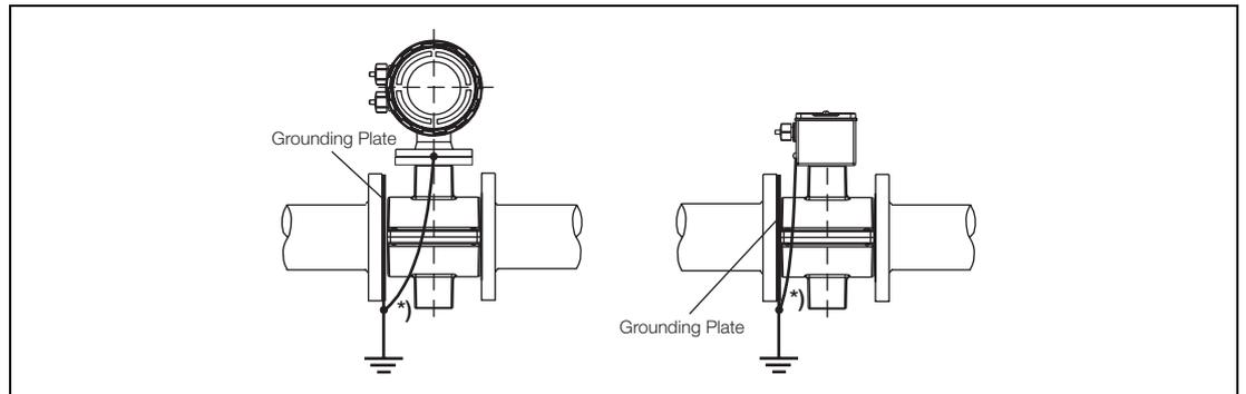
Fig. 22: Flowmeter Primary DN 3 - DN 100 [1/10" - 4"] Wafer Design
