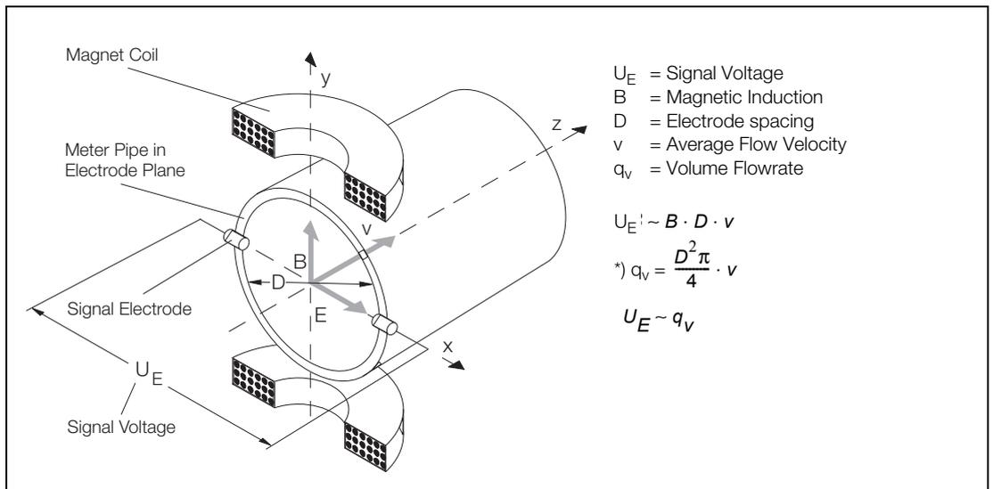
Fig. 1: Schematic of an Electromagnetic Flowmeter
