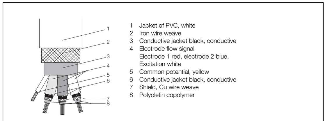
Fig. 27: Signal Cable Construction ABB No. D173D025U01
