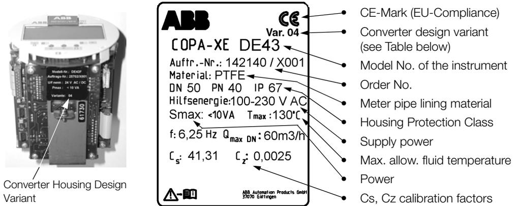
The identification of the converter design may be found on the tag on the metal frame of the converter (see Figure), or on the factory tag on the converter housing.
