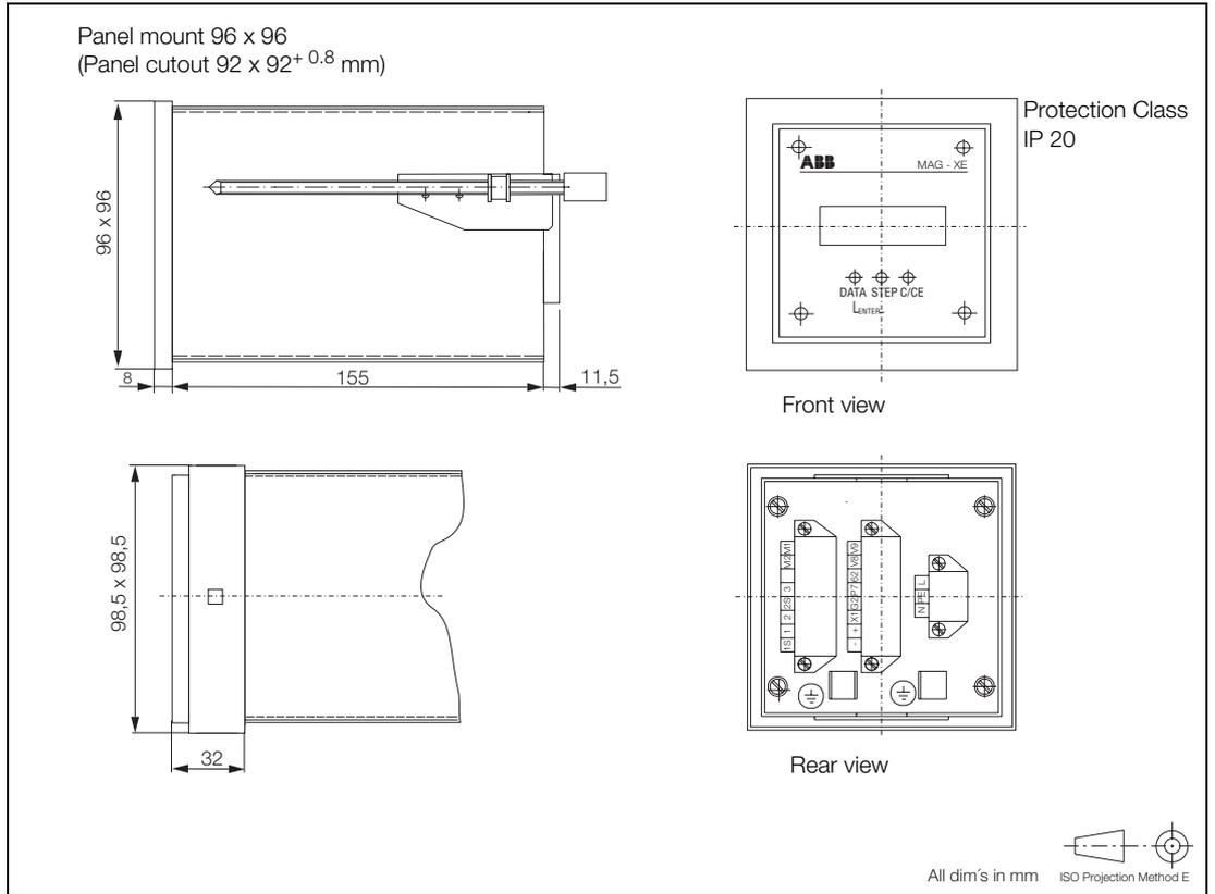
Fig. 76: Dimensions Converter FXE4000 (MAG-XE), Panel Mount Housing
