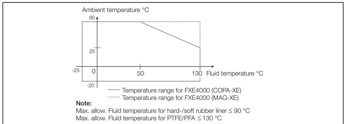
Fig. 53: Max. allow. Fluid Temperature as a Function of the Ambient Temperature for Instruments with Stainless Steel Flanges
