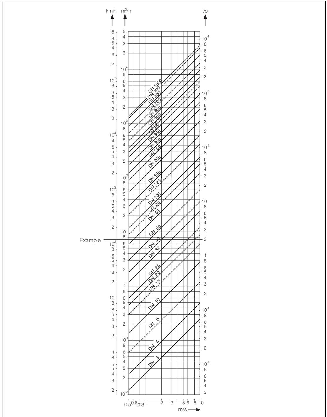
Fig. 15: Flowrate Nomograph DN 3 to DN 1000 [1/10" to 40"]
