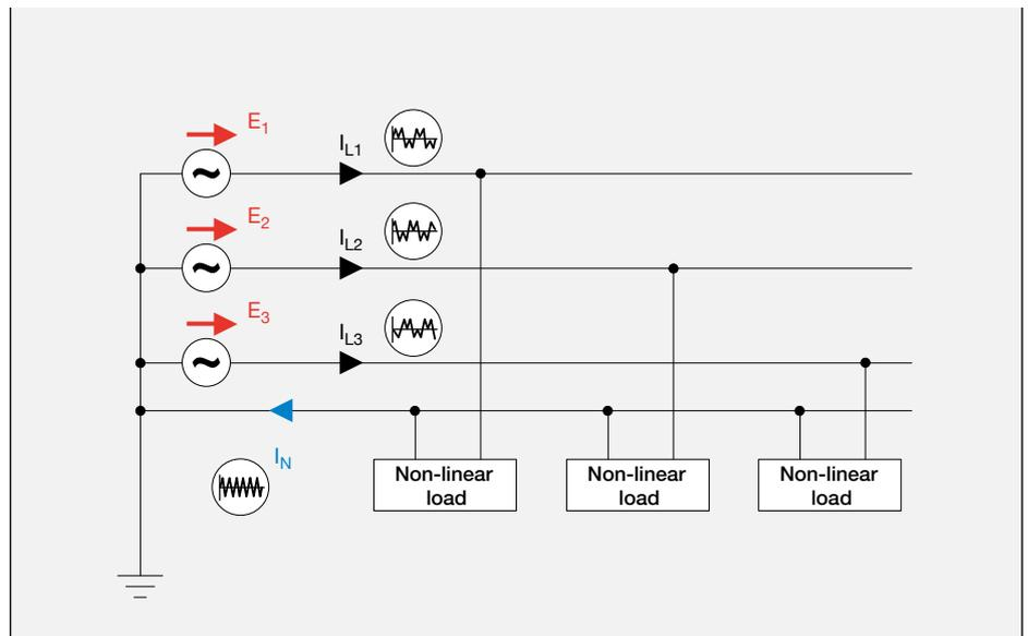
Neutral current in the case of non-linear balanced loads
